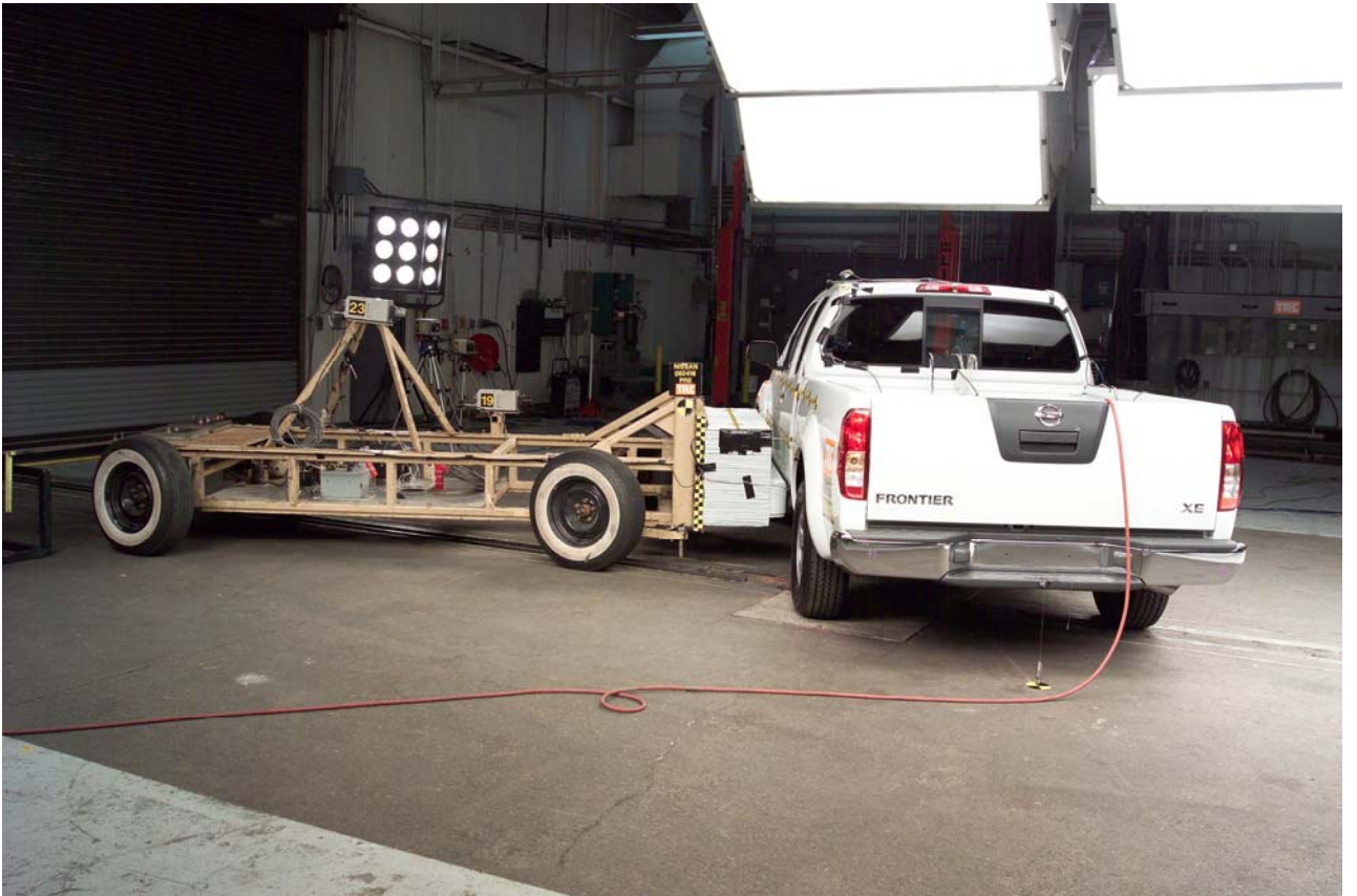
Figure A-69 Pre-Test Moving Barrier and Vehicle Rear View
