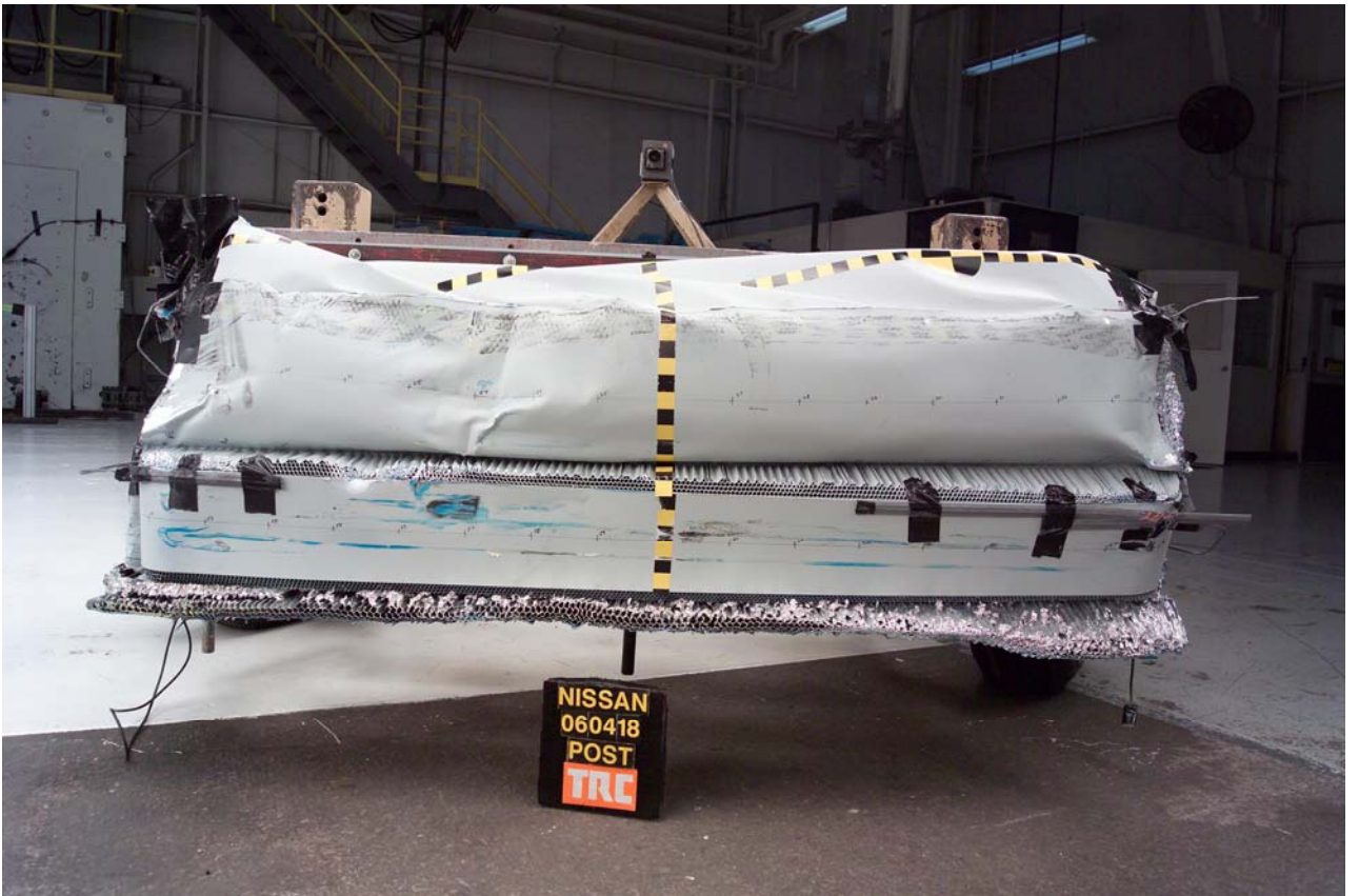
Figure A-56 Post-Test Front View of Deformable Barrier
