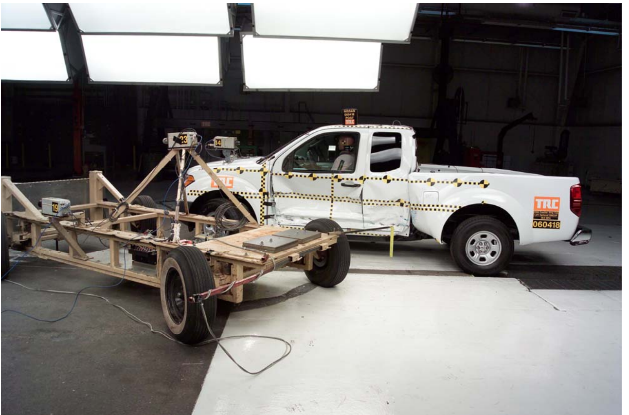
Figure A-67 Post-Test Moving Barrier and Vehicle Left Side View
