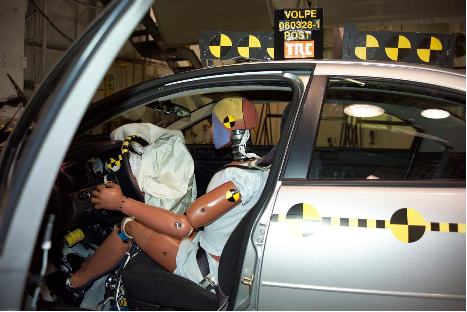
Figure A-42 Post-Test Driver Dummy - View 3 A-43
