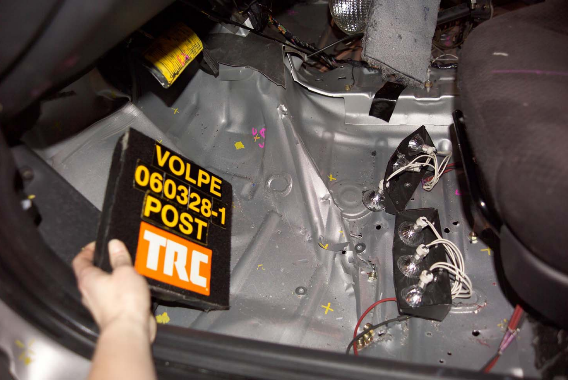
Figure A-53 Post-Test Driver Floorboard Deformation - View 5 A-54
