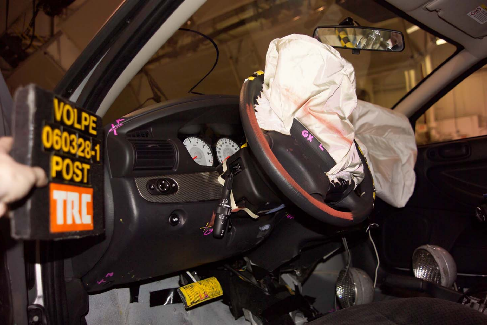
Figure A-57 Post-Test Driver Instrument Panel Damage - View 2 A-58
