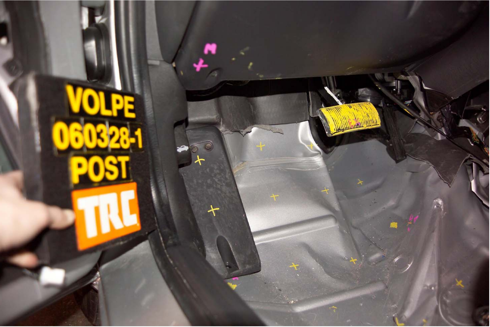
Figure A-52 Post-Test Driver Floorboard Deformation - View 4 A-53
