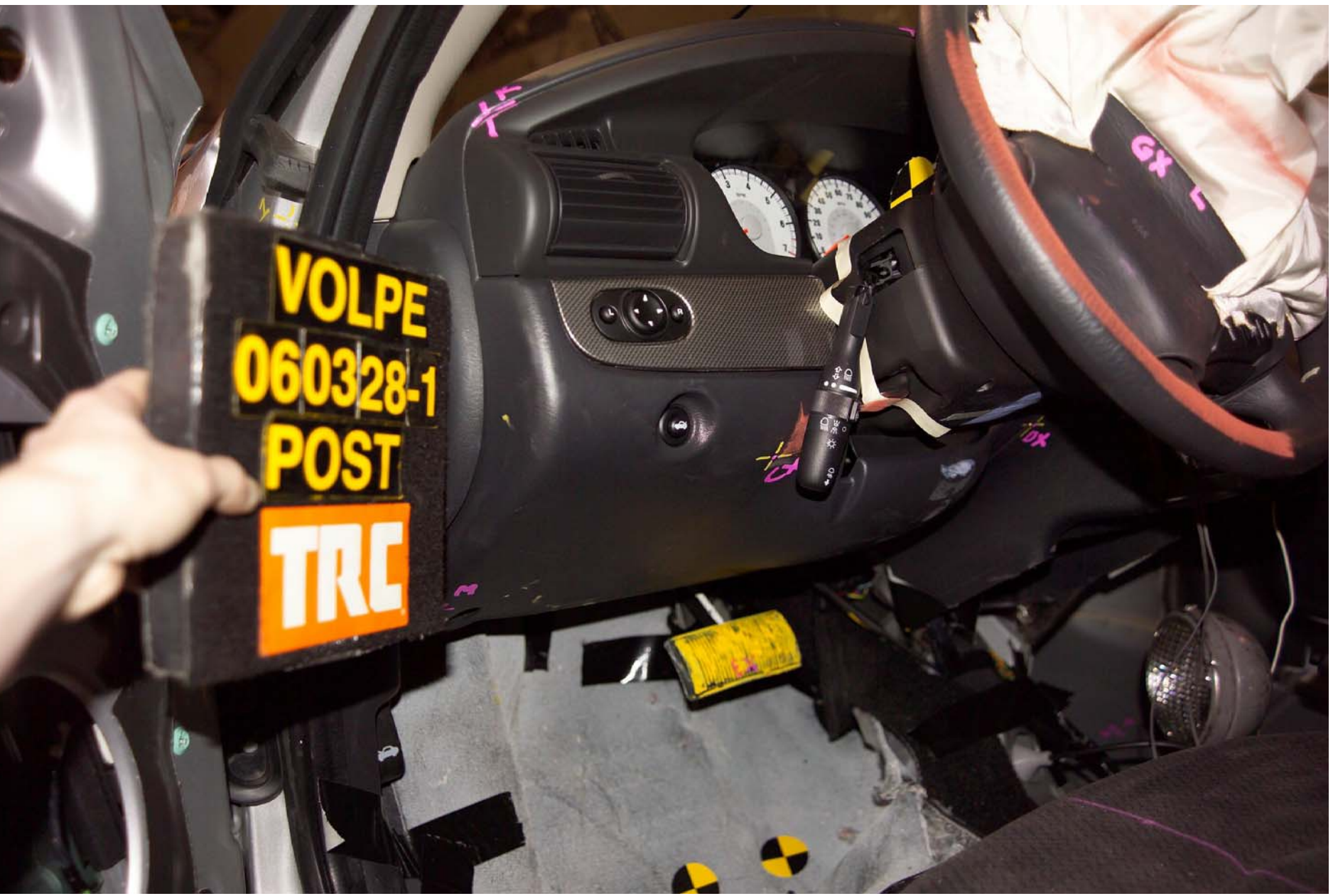
Figure A-56 Post-Test Driver Instrument Panel Damage - View 1 A-57
