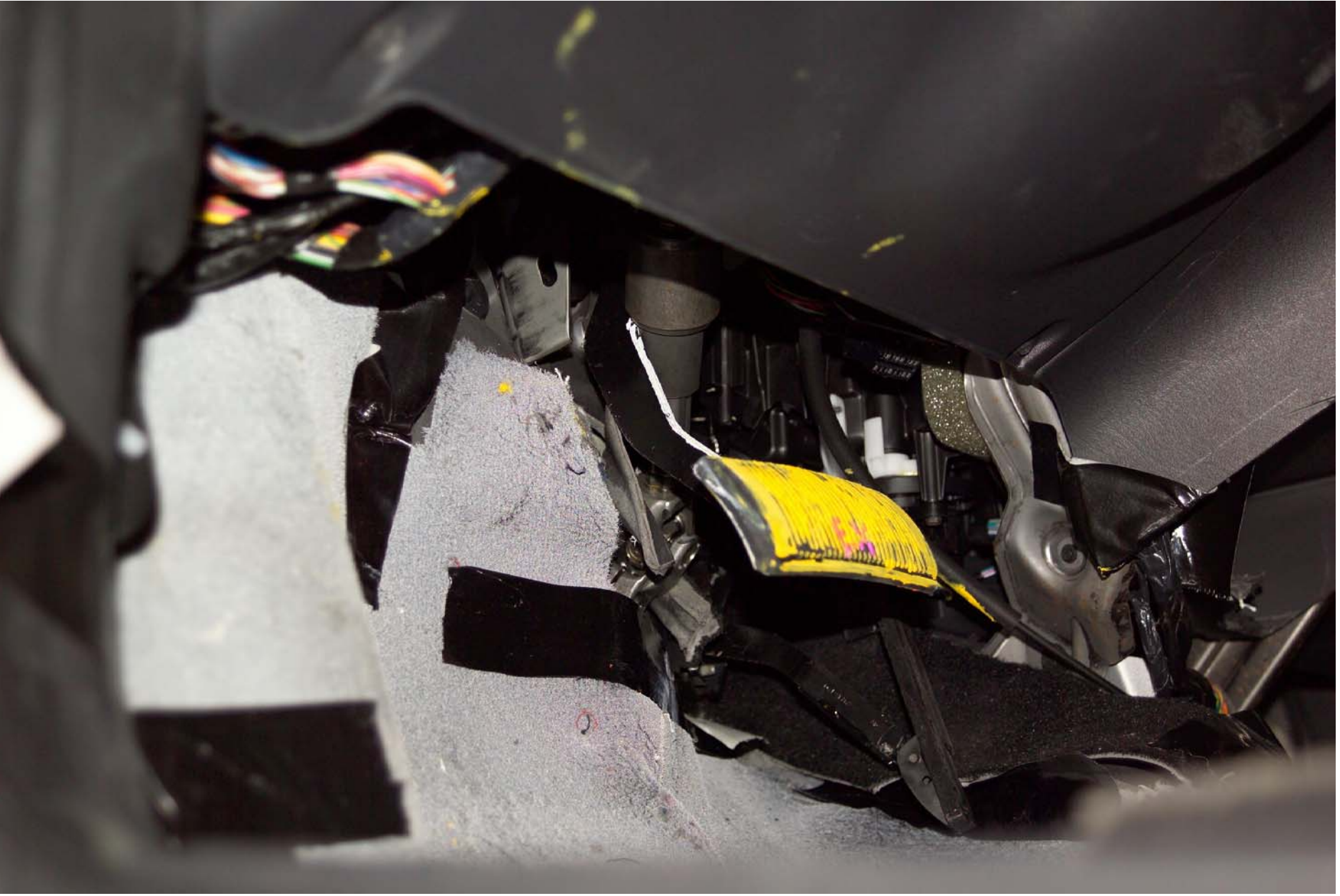
Figure A-55 Post-Test Driver Toeboard Deformation - View 2 A-56
