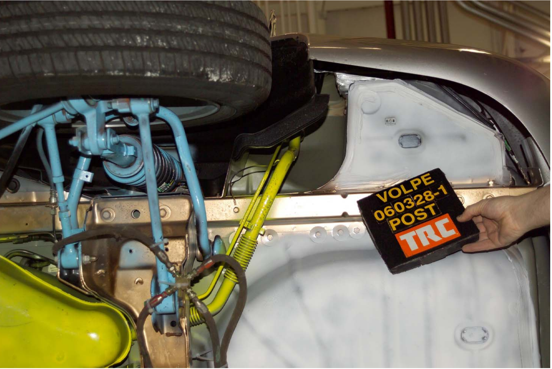
Figure A-34 Post-Test Fuel Filler Neck View
