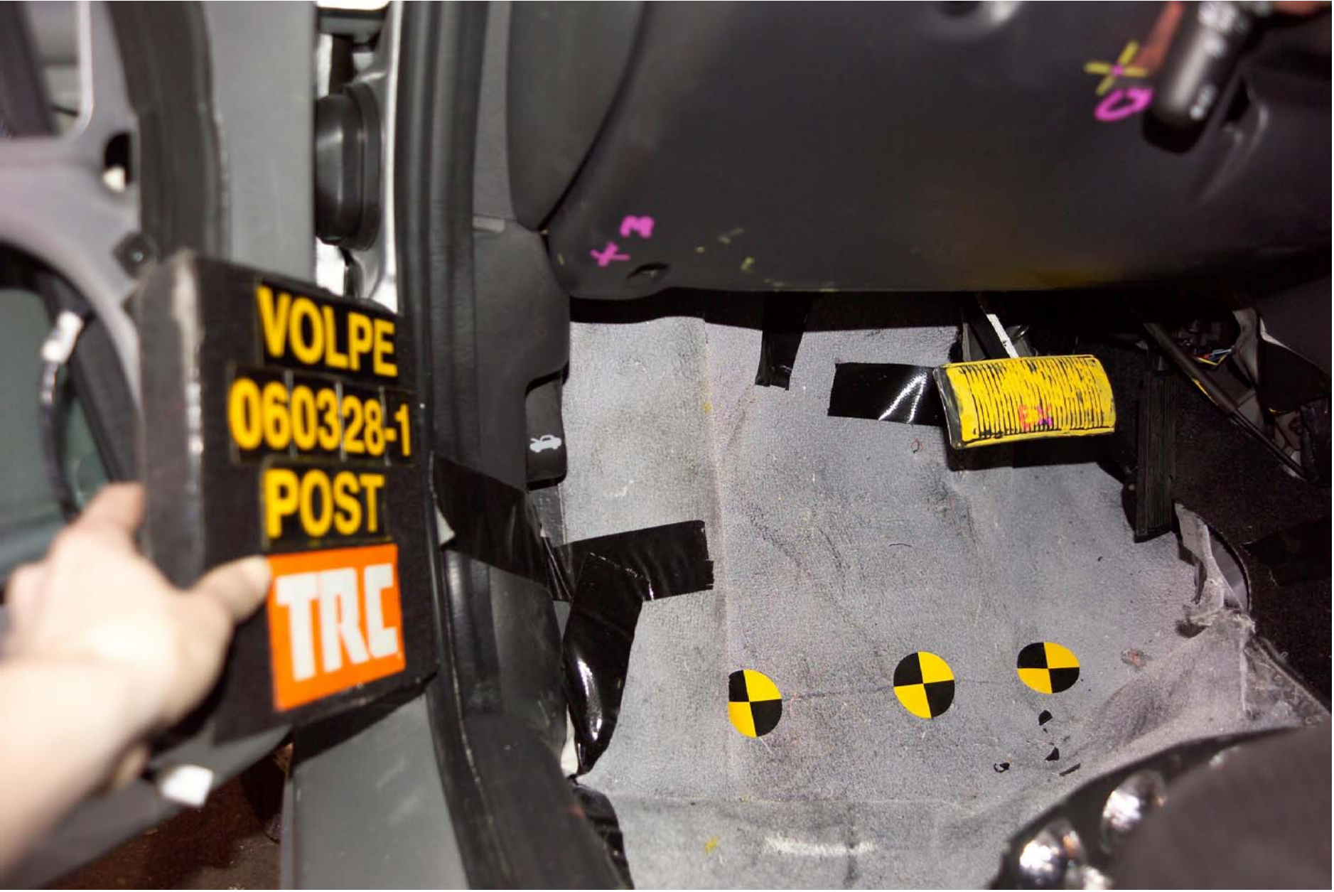
Figure A-49 Post-Test Driver Floorboard Deformation - View 1 A-50
