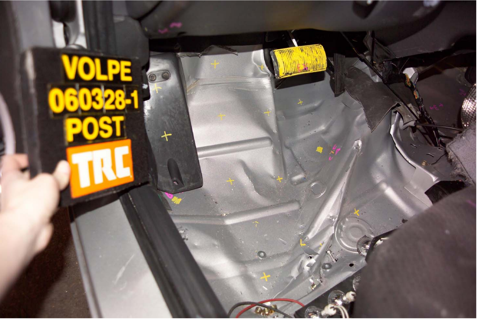
Figure A-51 Post-Test Driver Floorboard Deformation - View 3 A-52
