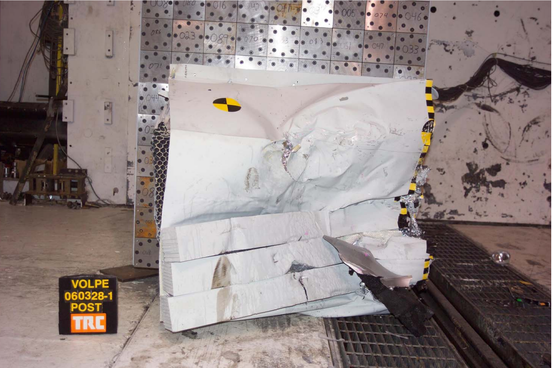
Figure A-59 Post-Test Barrier Front View A-60
