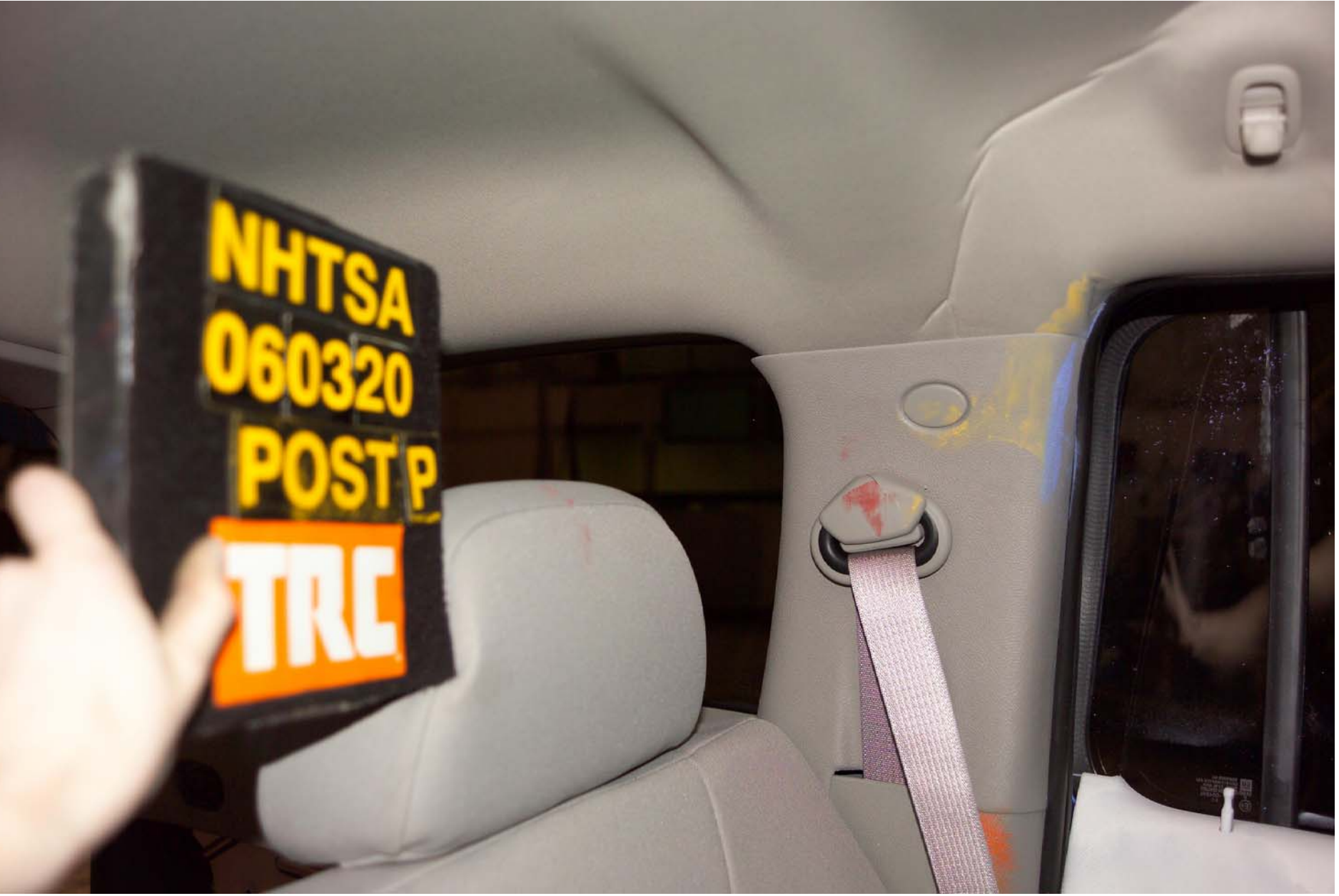
Figure A-60 Post-Test Rear SID HIII Contact - View 1 A-64
