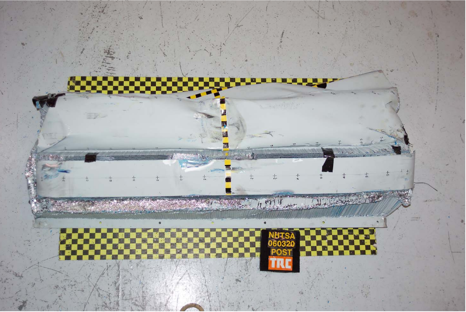
Figure A-17 Post-Test Frontal View of Impactor Face A-21
