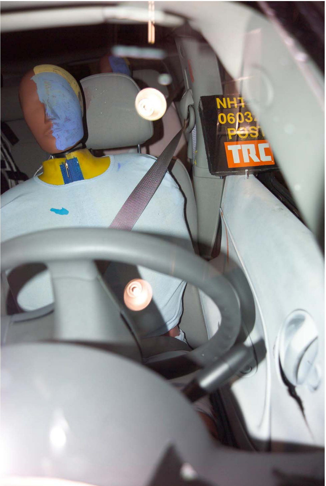
Figure A-48 Post-Test Left View of Front SID HIII and Door Clearance
