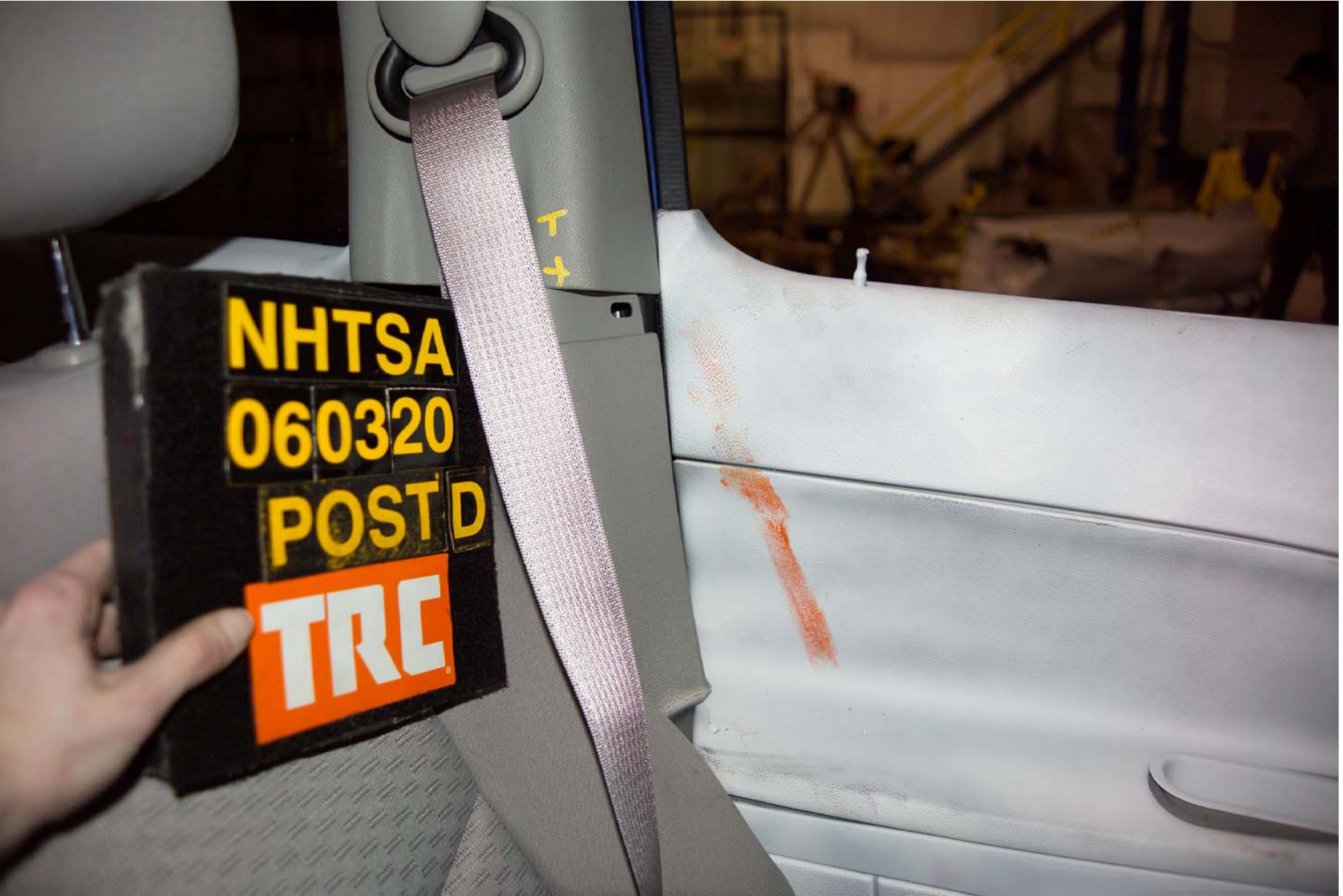
Figure A-56 Post-Test Front SID HIII Contact - View 3 A-60
