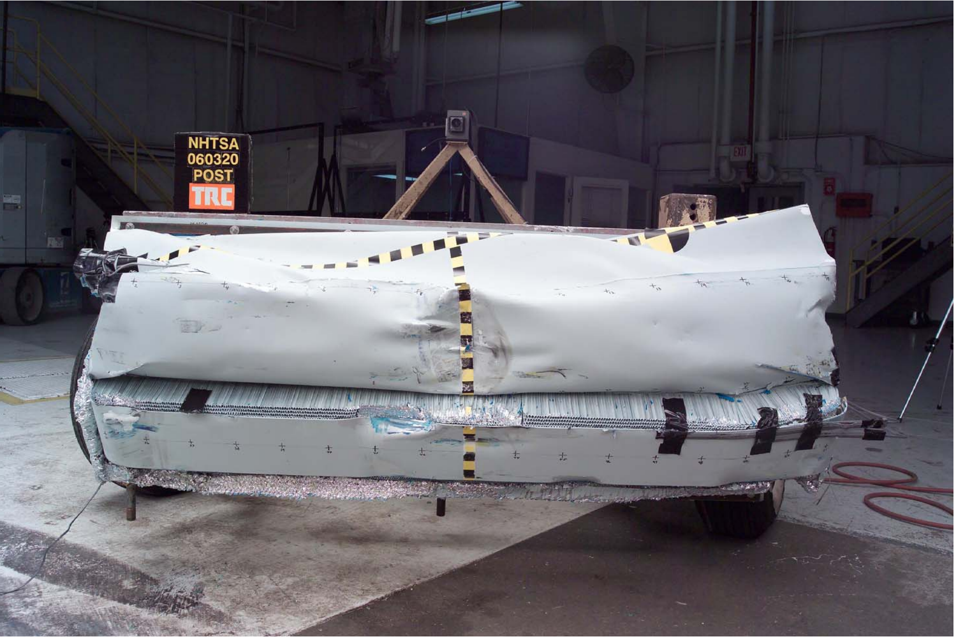
Figure A-25 Post-Test Front View of Impactor A-29
