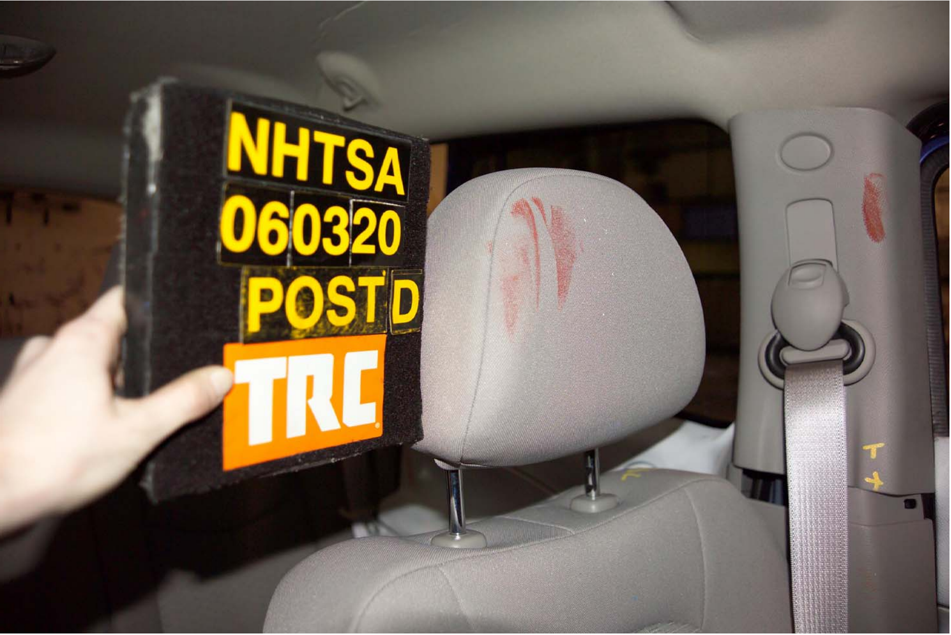
Figure A-54 Post-Test Front SID HIII Contact - View 1 A-58
