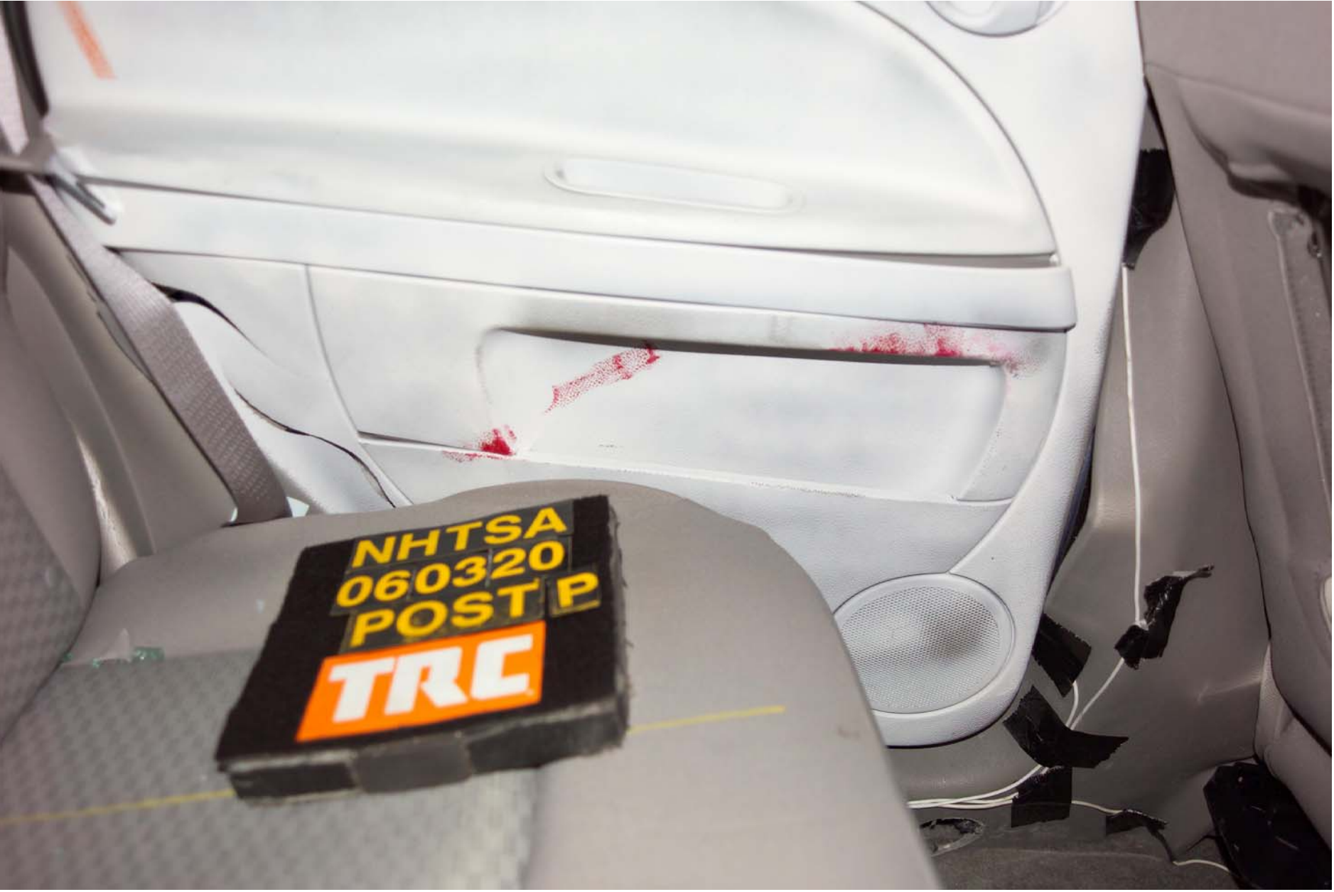
Figure A-62 Post-Test Rear SID HIII Contact - View 3 A-66
