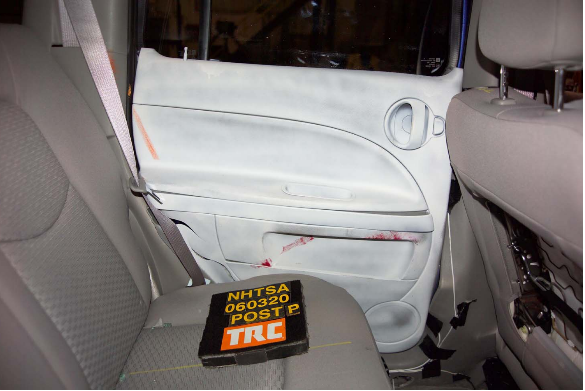
Figure A-59 Post-Test Interior of Rear Panel Showing SID HIII Impact Locations
