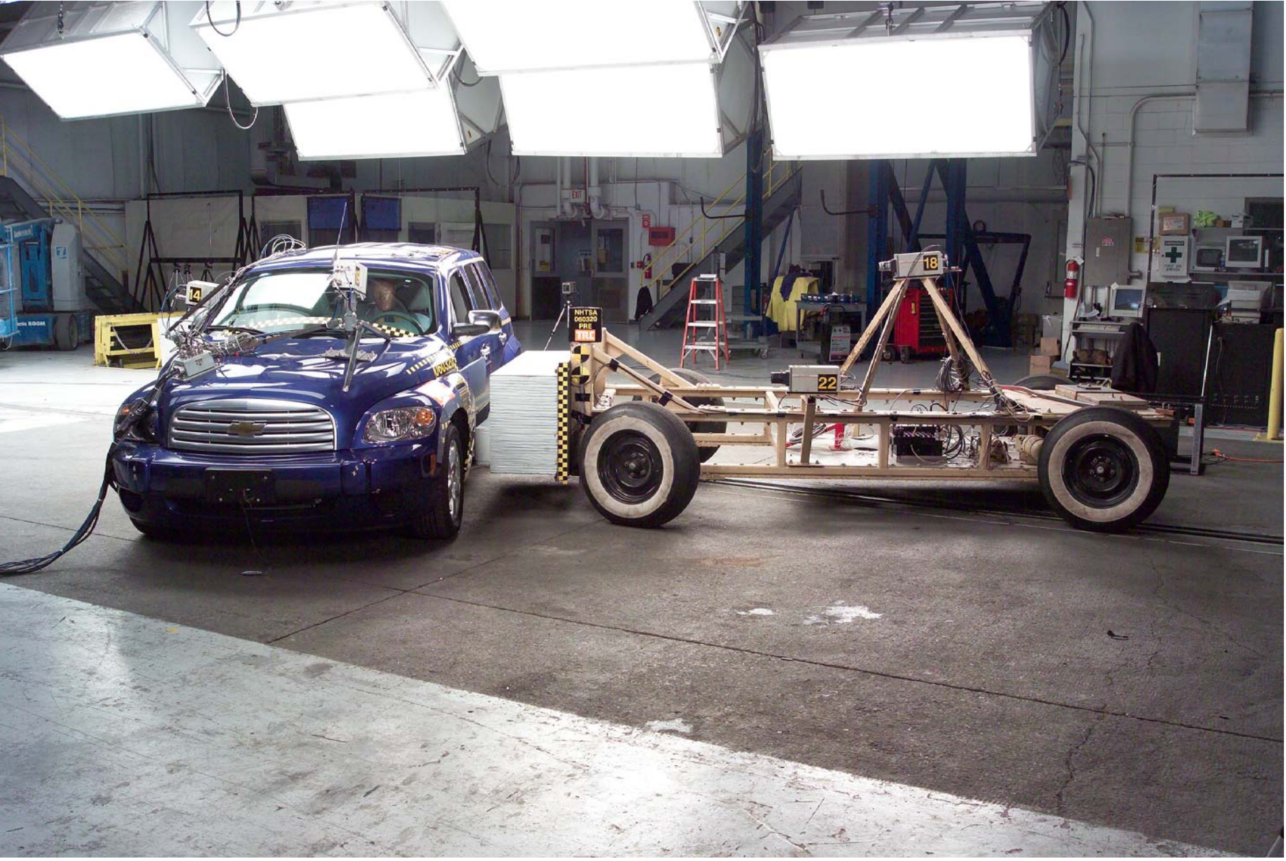
Figure A-63 Pre-Test Left Side View of MDB With Impactor Face in Position A-67
