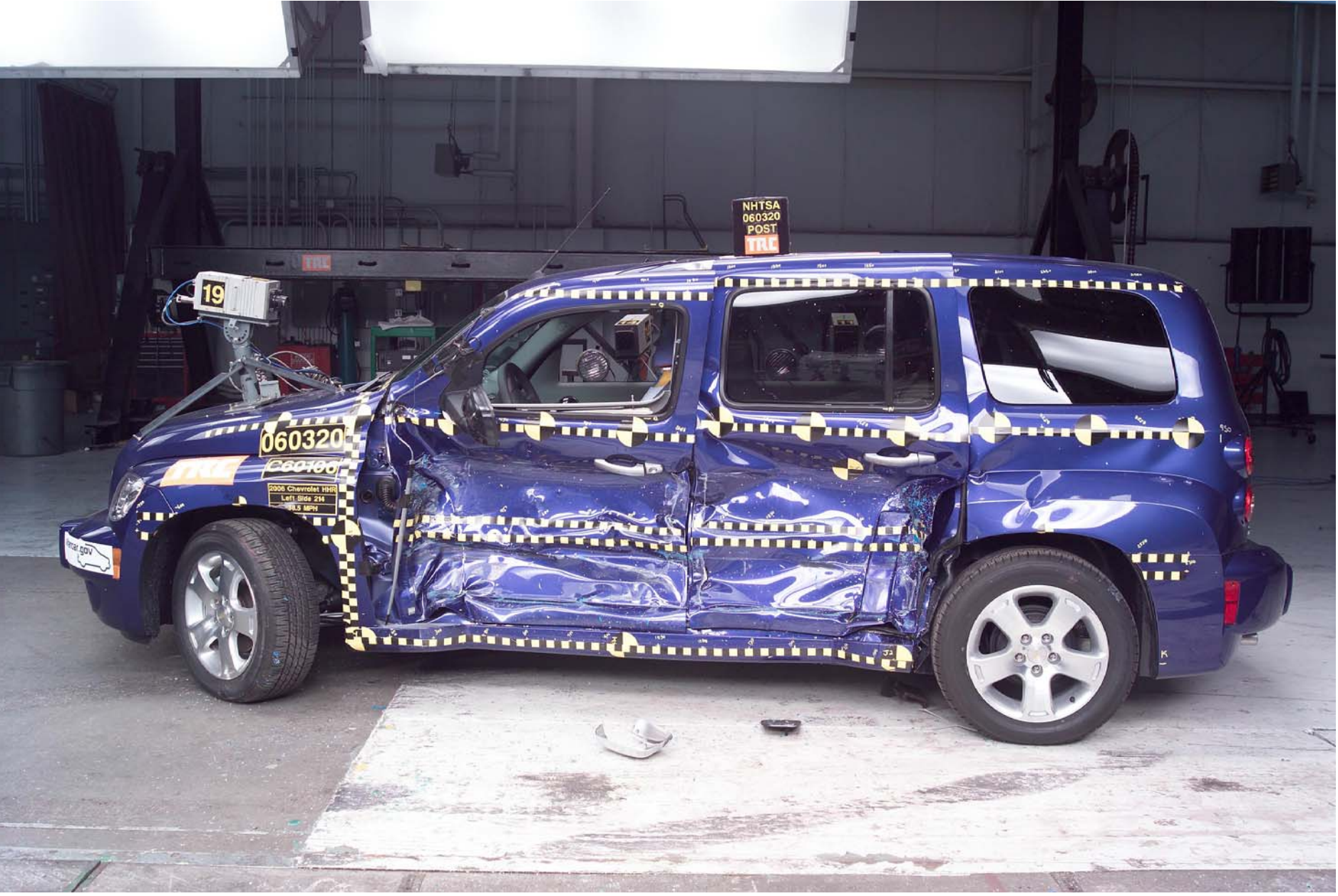
Figure A-5 Post-Test Impacted Side View of Test Vehicle A-9
