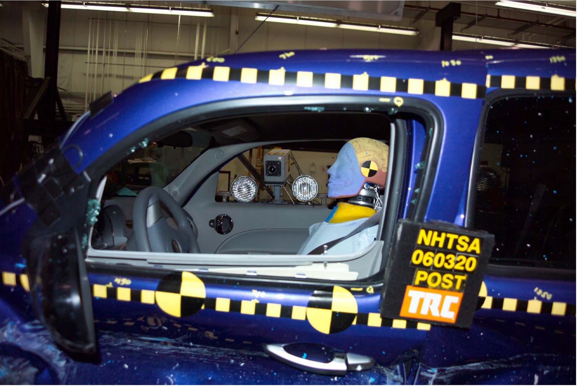
Figure A-45 Post-Test Left View of Front SID HIII A-49
