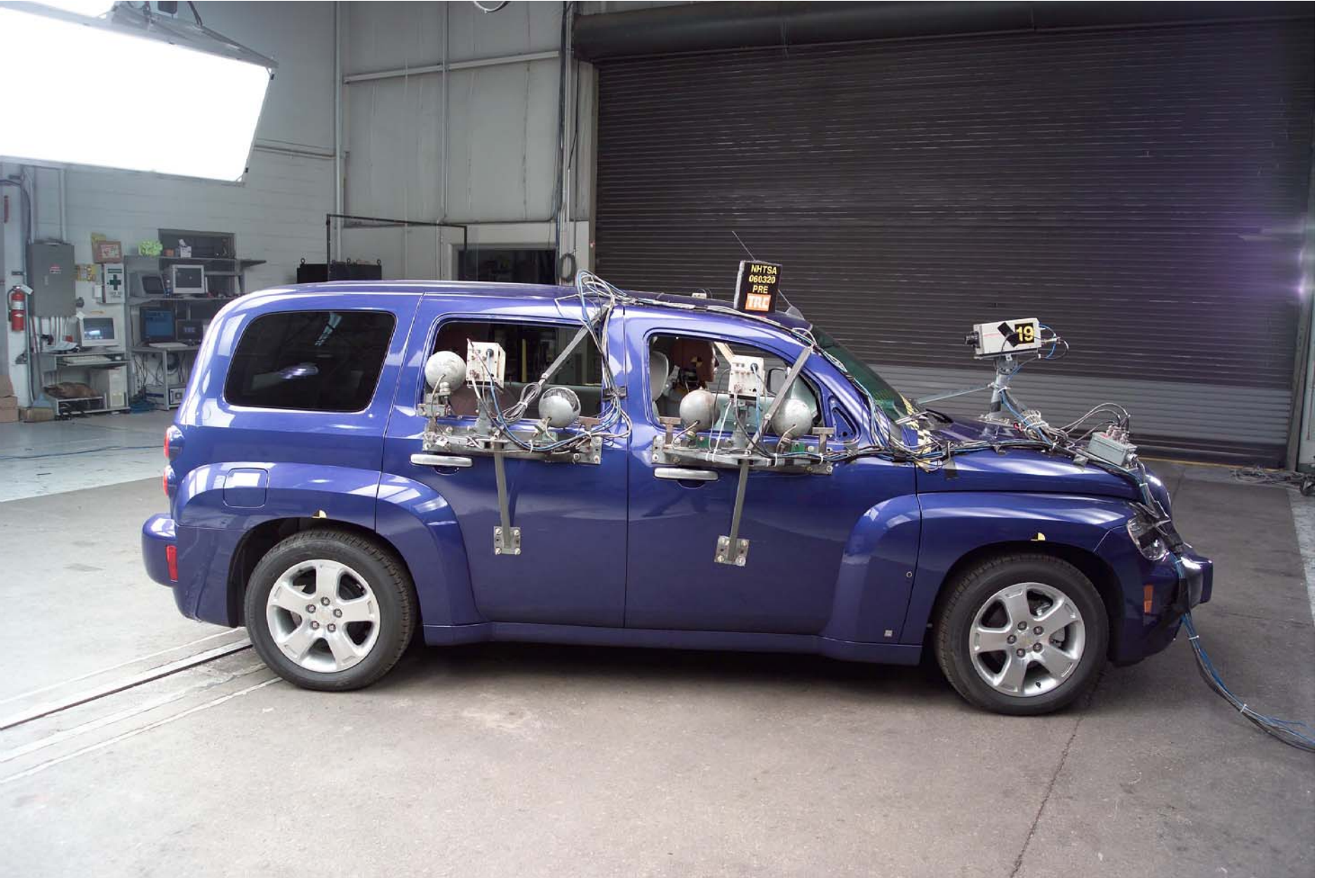
Figure A-12 Pre-Test Right Side View of Test Vehicle A-16
