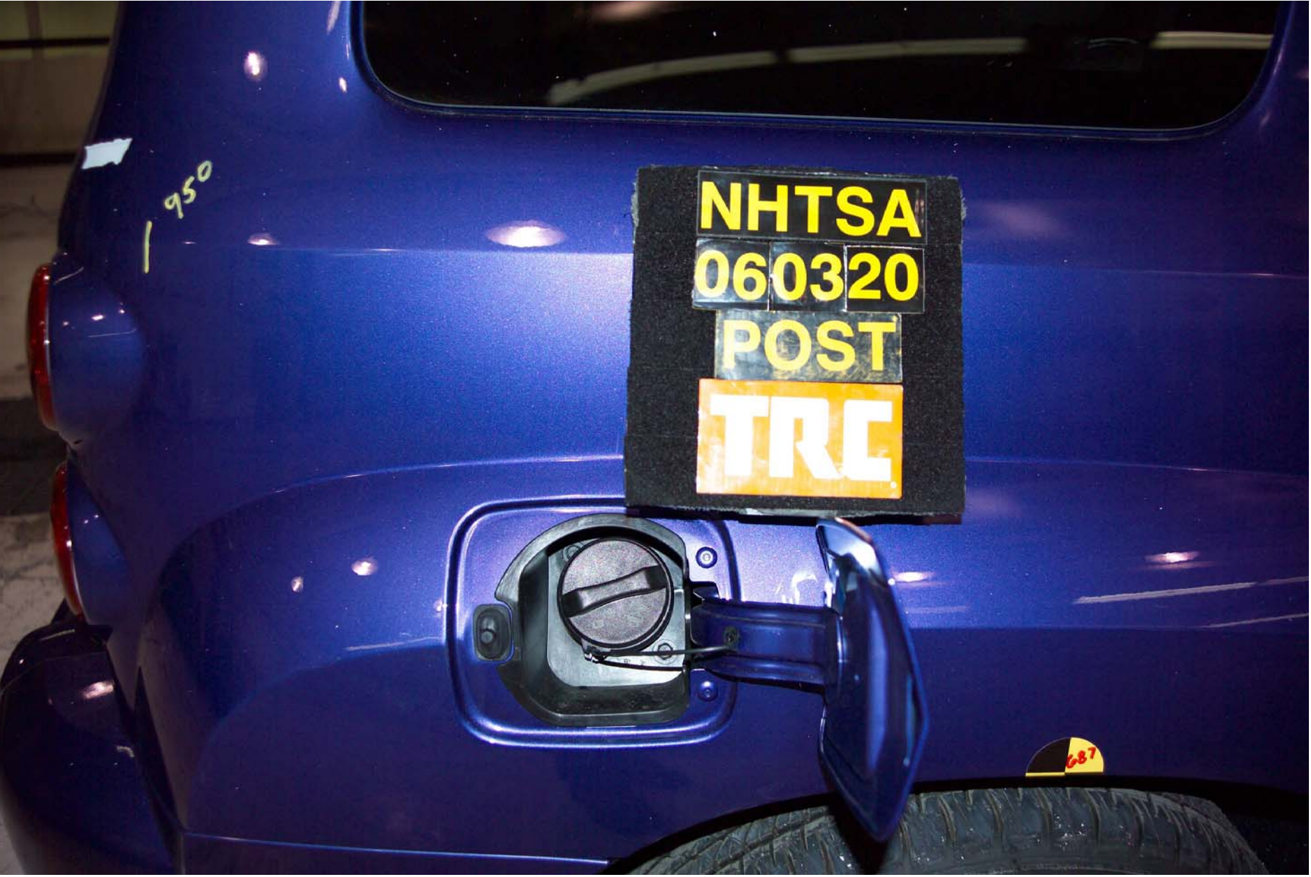
Figure A-79 Post-Test Fuel Cap A-83
