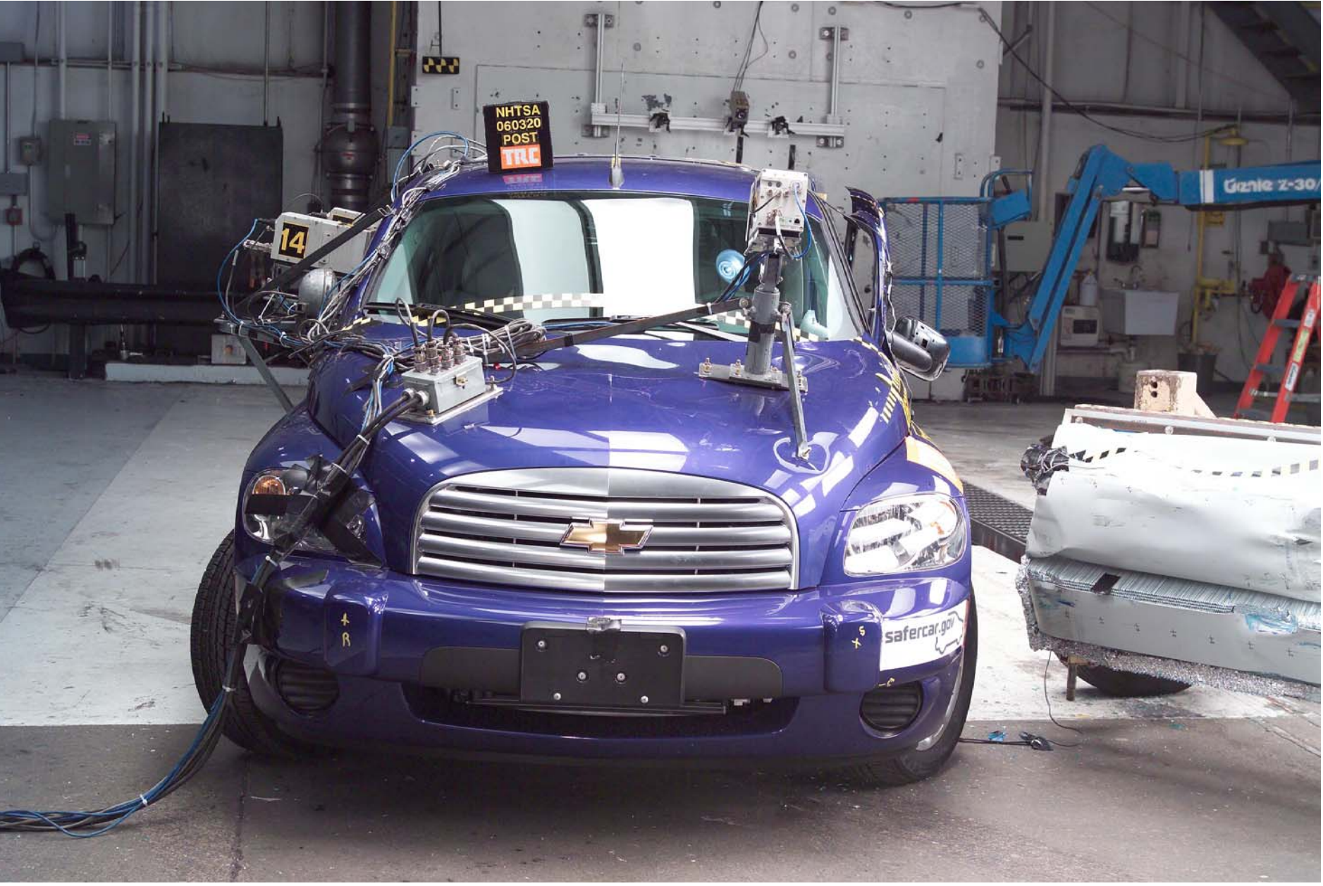
Figure A-2 Post-Test Front View of Test Vehicle A-6
