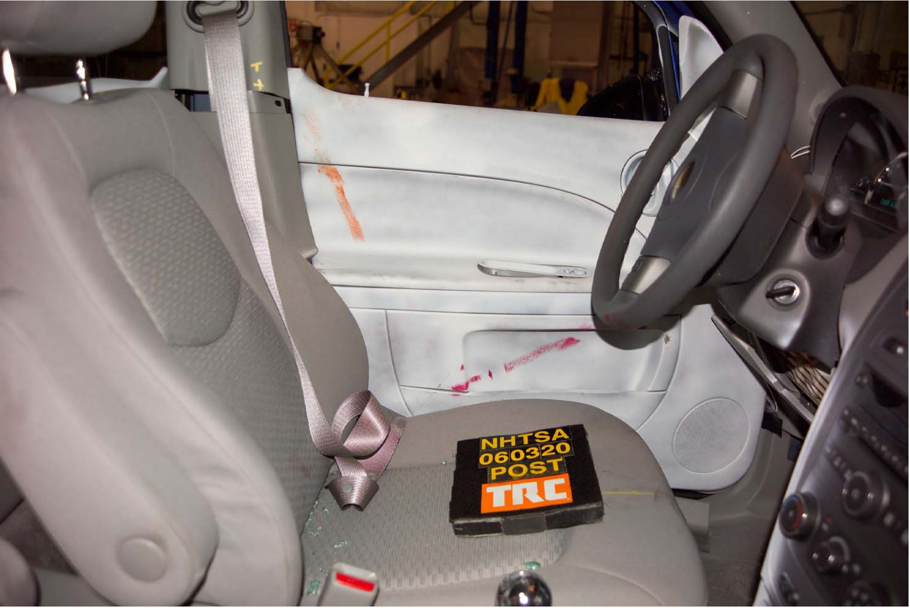
Figure A-53 Post-Test Interior of Front Door Showing SID HIII Impact Locations
