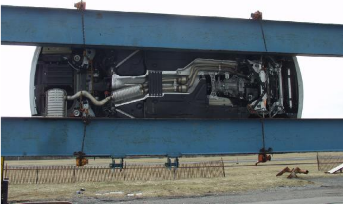
Figure A-53: Rollover 270 Degrees
