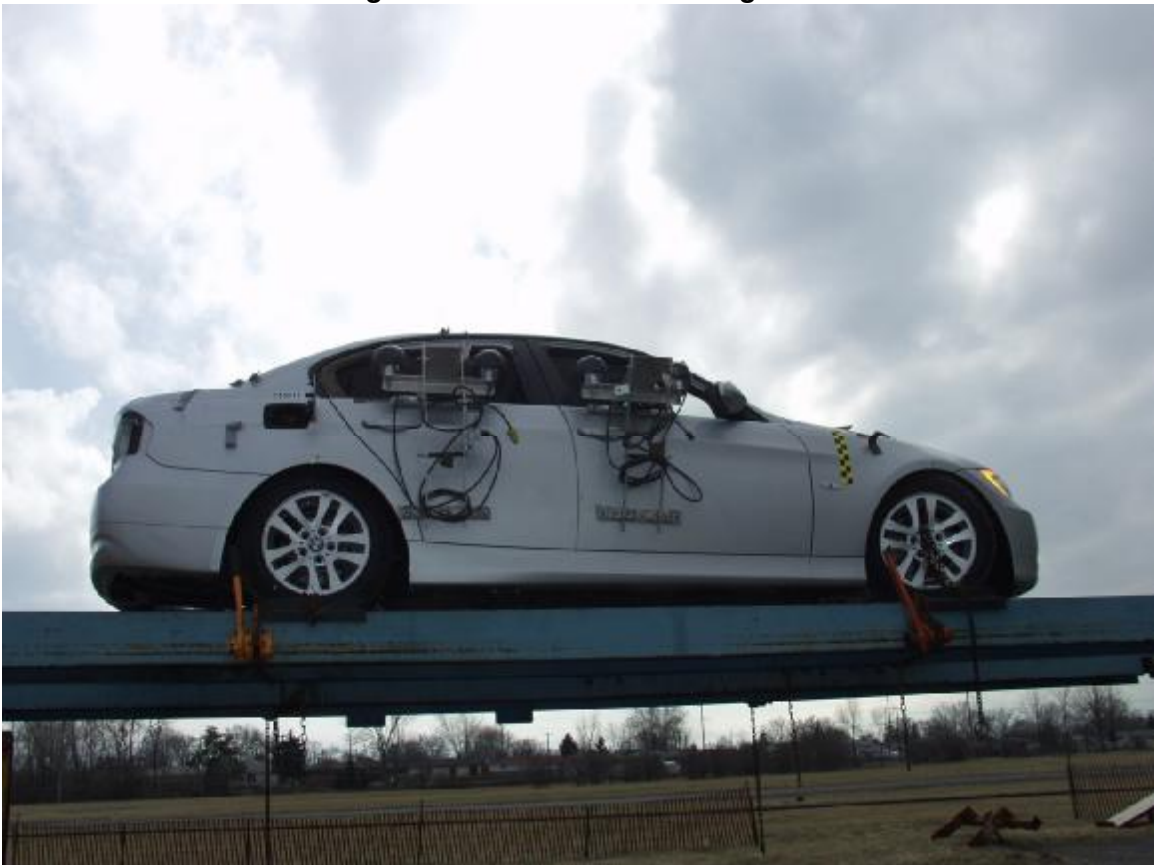
Figure A-54: Rollover 360 Degrees
