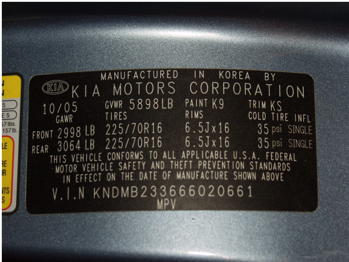
Figure A-3: Vehicle Certification Label
