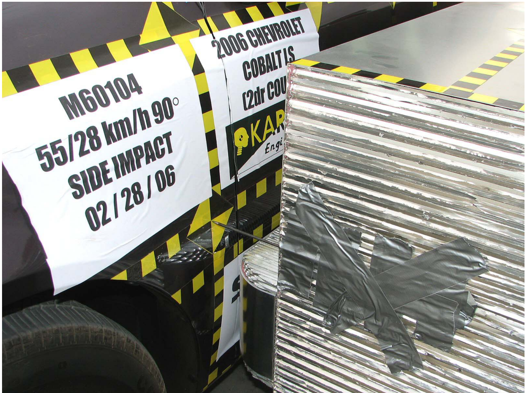
Figure A-25: Pre-Test Left Impact Point
