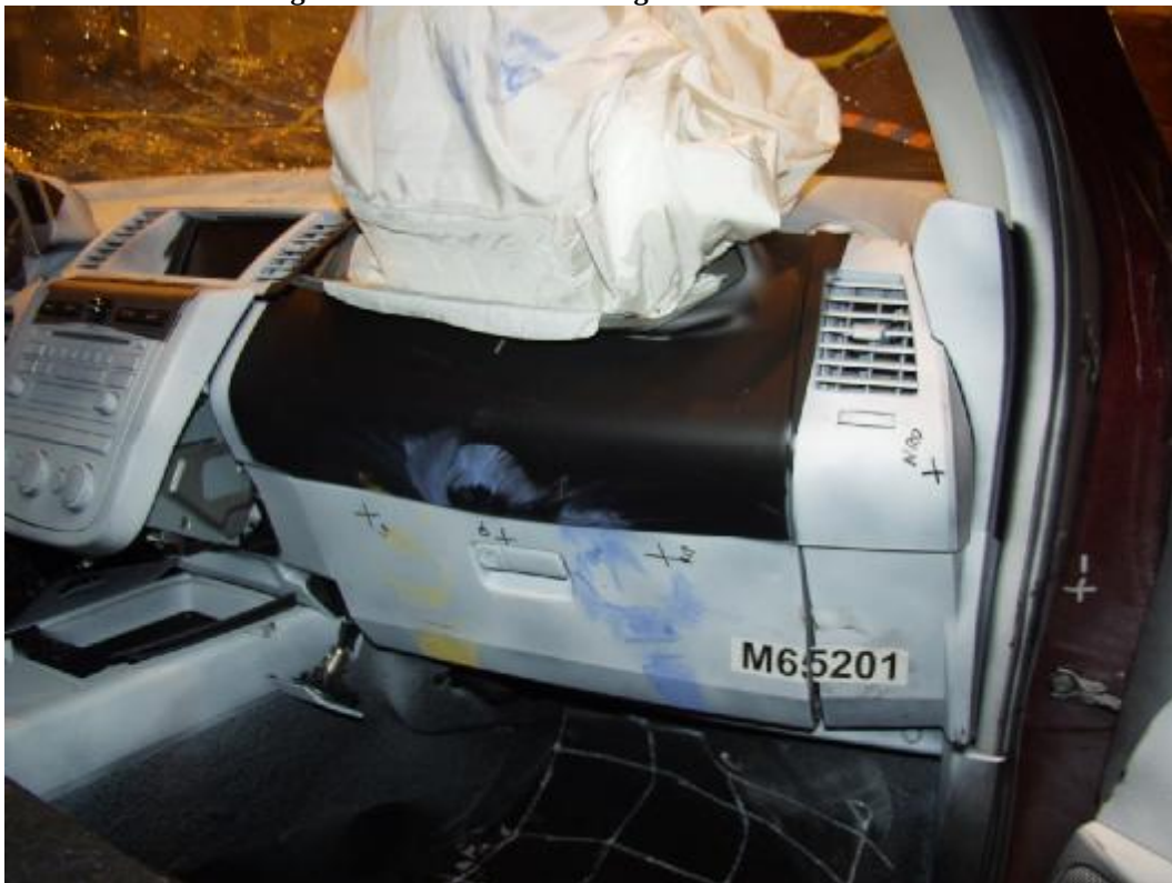
Figure A-53: Post-Test Passenger Knee Bolster View
