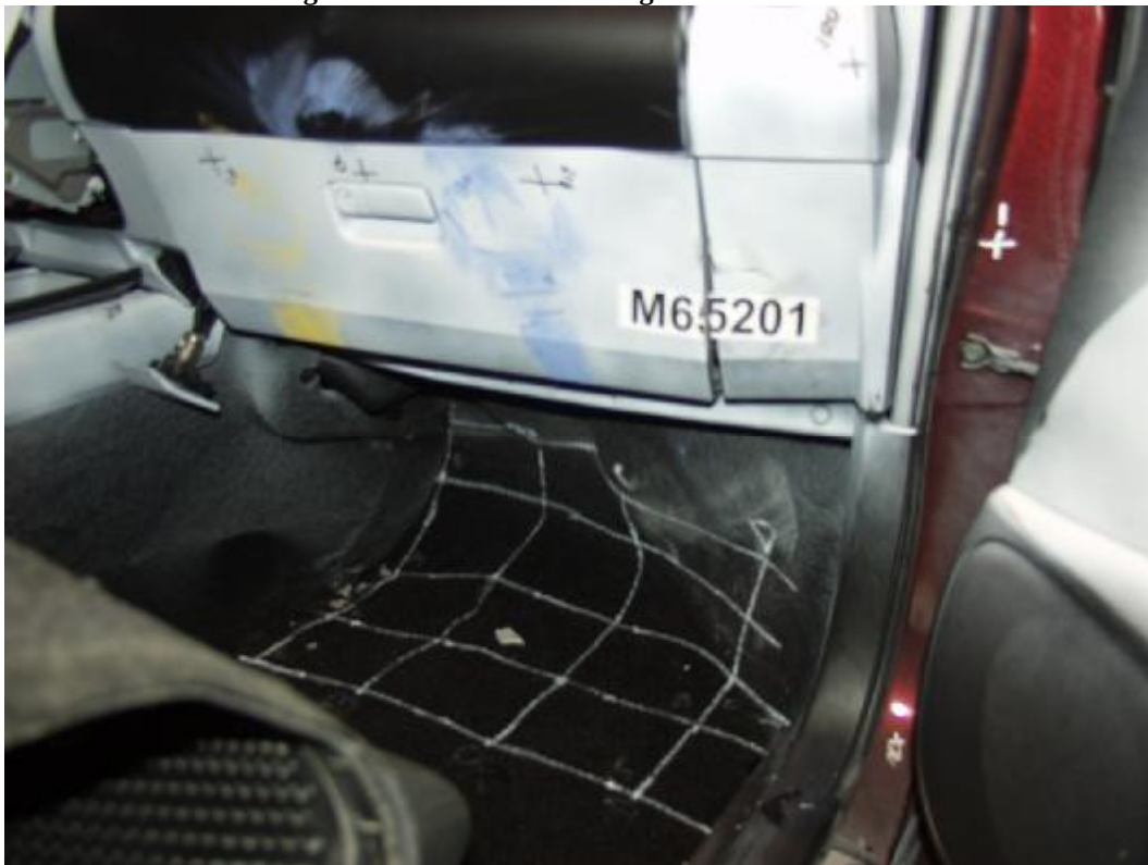
Figure A-55: Post-Test Passenger Floor Pan View
