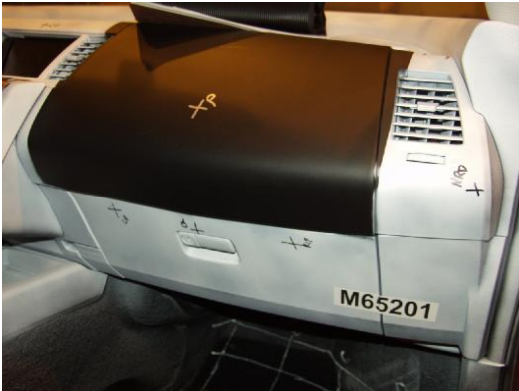
Figure A-52: Pre-Test Passenger Knee Bolster View
