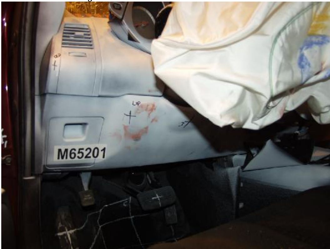
Figure A-39: Post-Test Driver Knee Bolster View
