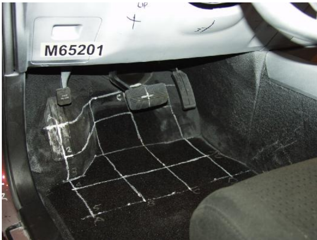
Figure A-40: Pre-Test Driver Floor Pan View
