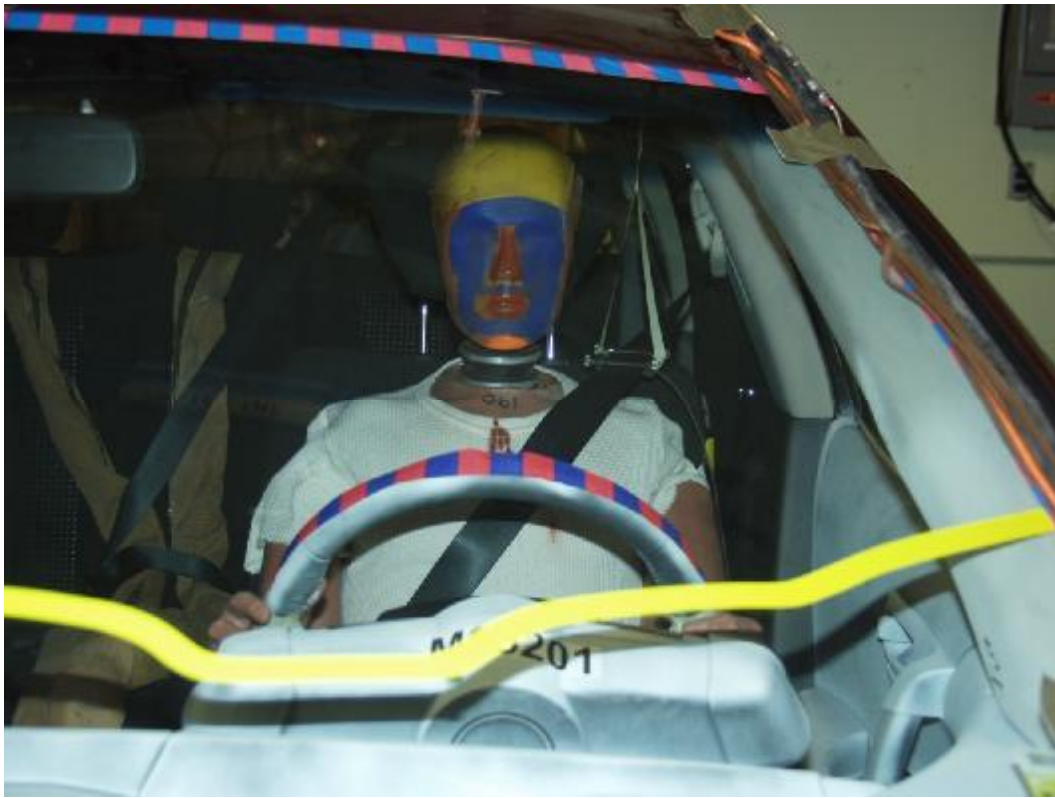
Figure A-30: Pre-Test Driver Head Location
