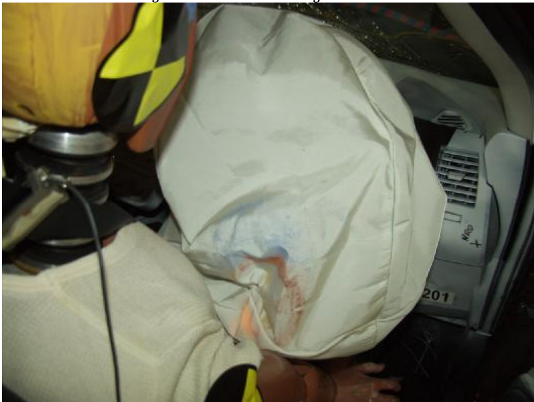
Figure A-57: Post-Test Passenger Contact to Airbag
