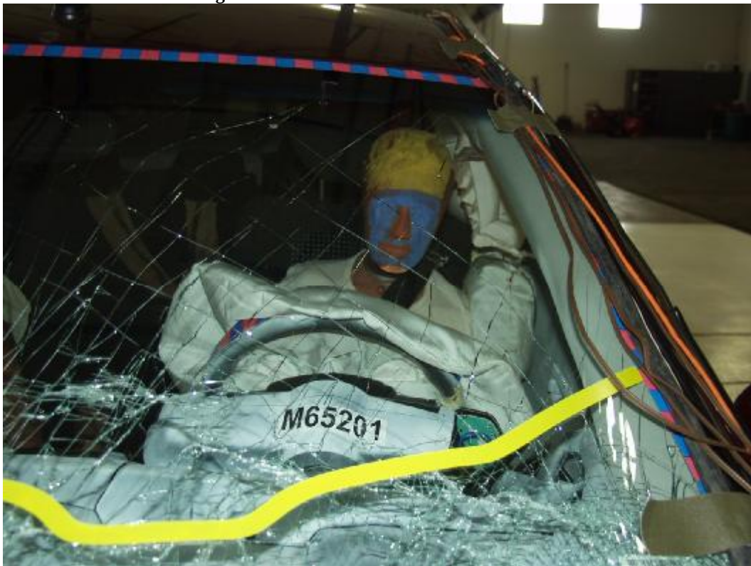
Figure A-31: Post-Test Driver Head Location
