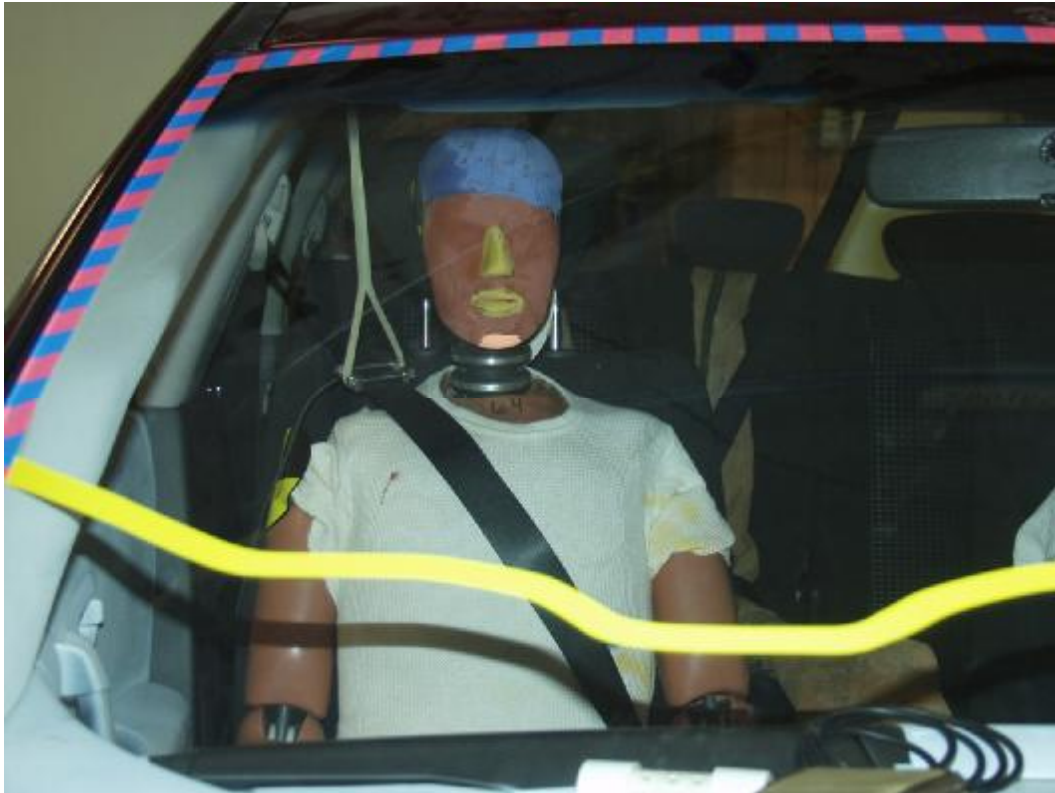
Figure A-44: Pre-Test Passenger Head Location
