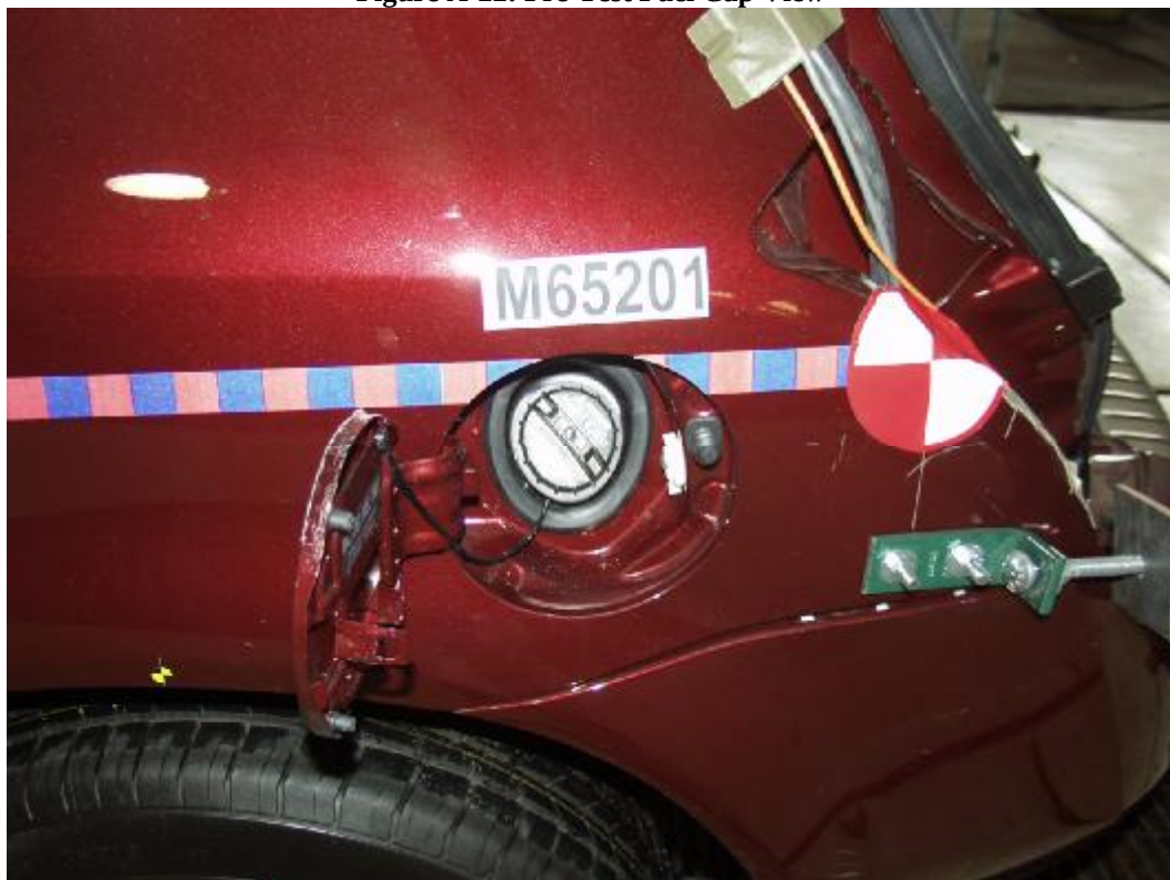
Figure A-23: Post-Test Fuel Cap View
