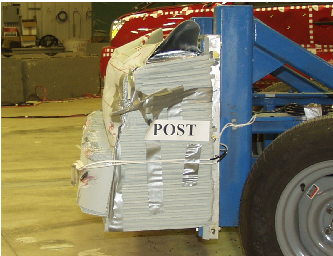
Figure A-56: Post test left side view of MDB barrier face
