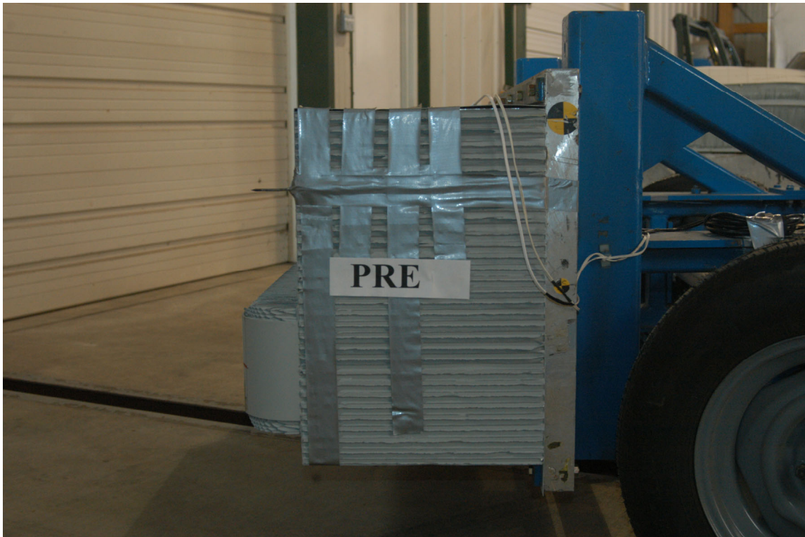
Figure A-55: Pre test left side view of MDB barrier face
