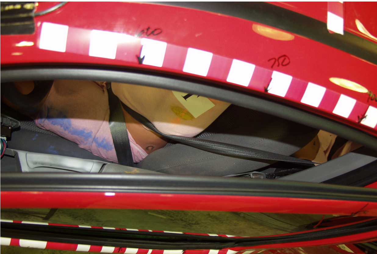
Figure A-38: Post test driver shoulder clearance
