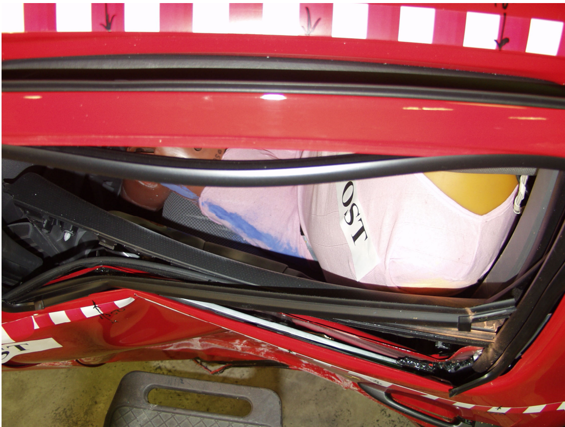
Figure A-46: Post test passenger shoulder clearance
