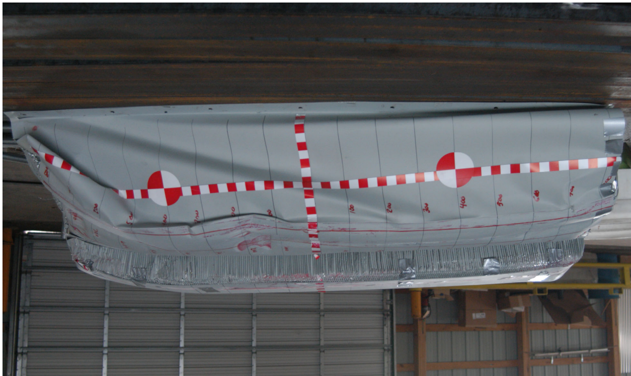
Figure A-58: Post test left side view of MDB barrier face
