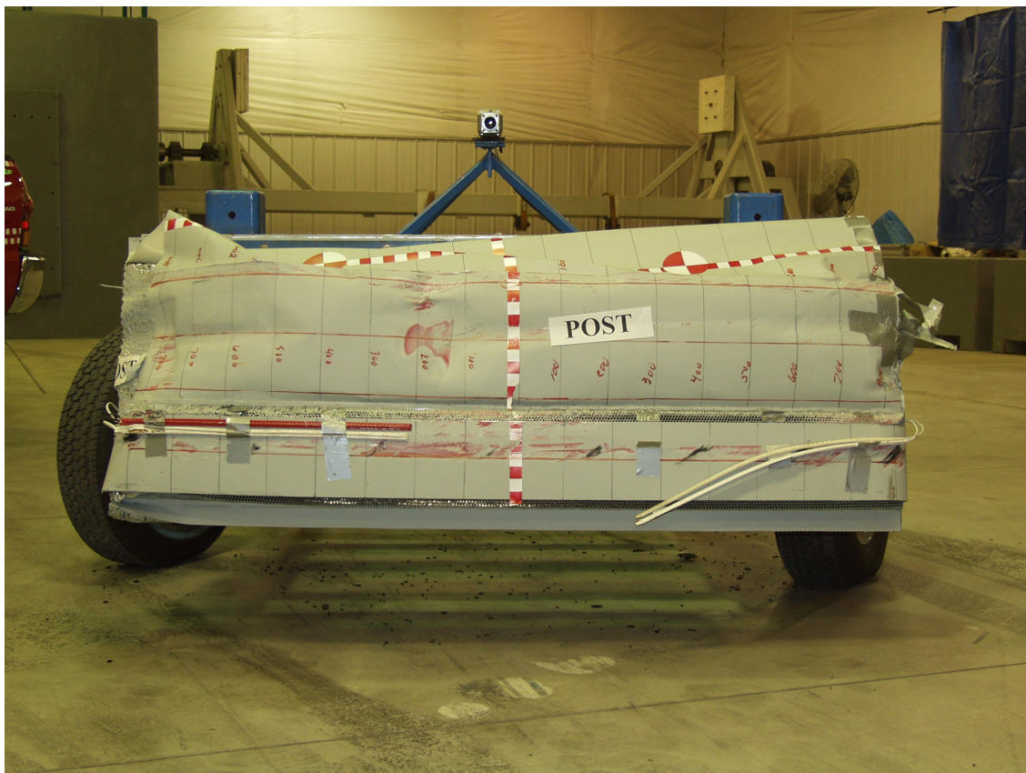
Figure A-52: Post test front view of MDB barrier face
