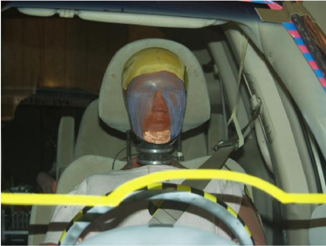
Figure A-30: Pre-Test Driver Head Location
