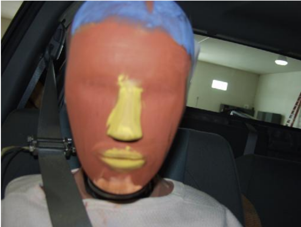
Figure A-56: Post-Test Passenger Head View
