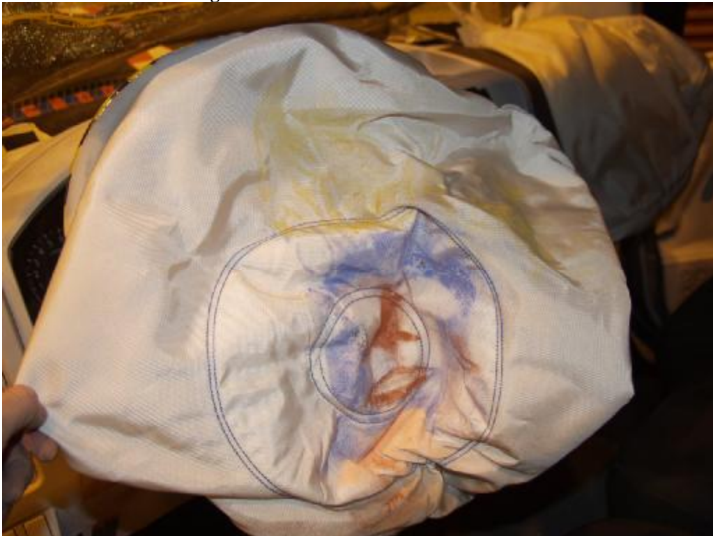
Figure A-43: Post-Test Driver Contact to Airbag
