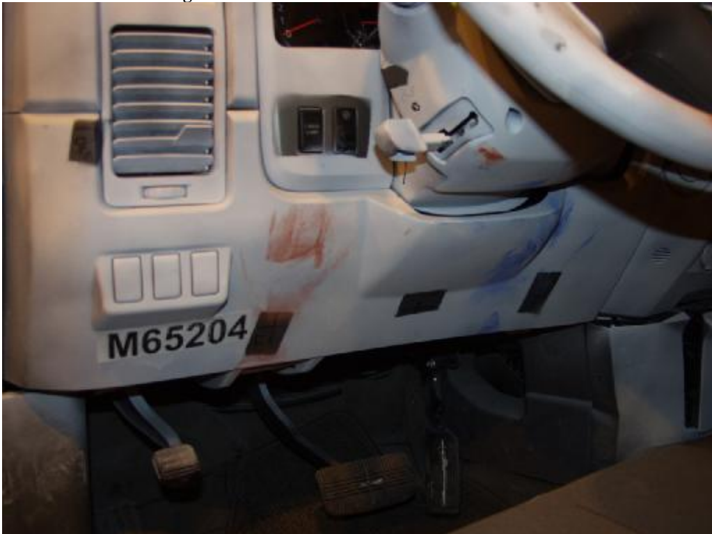
Figure A-39: Post-Test Driver Knee Bolster View
