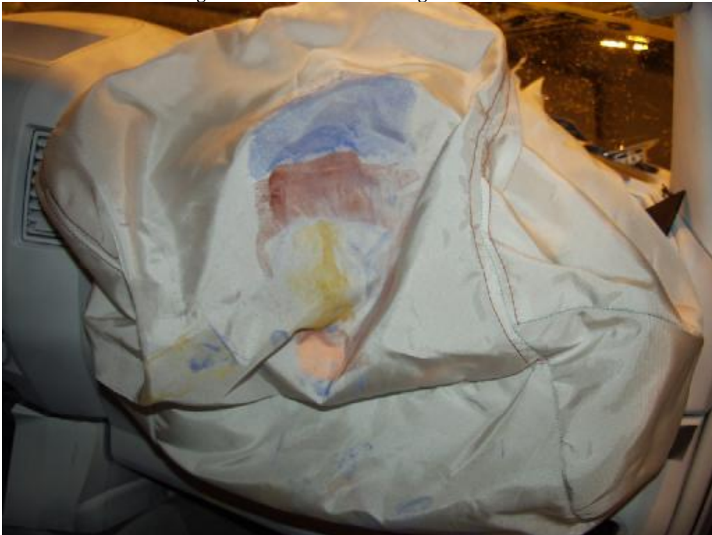
Figure A-57: Post-Test Passenger Contact to Airbag
