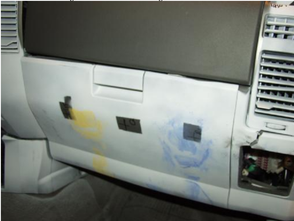
Figure A-53: Post-Test Passenger Knee Bolster View
