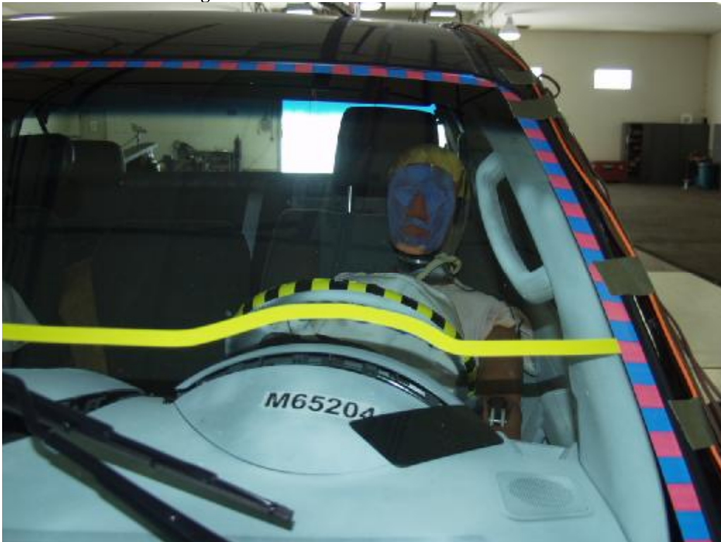
Figure A-31: Post-Test Driver Head Location
