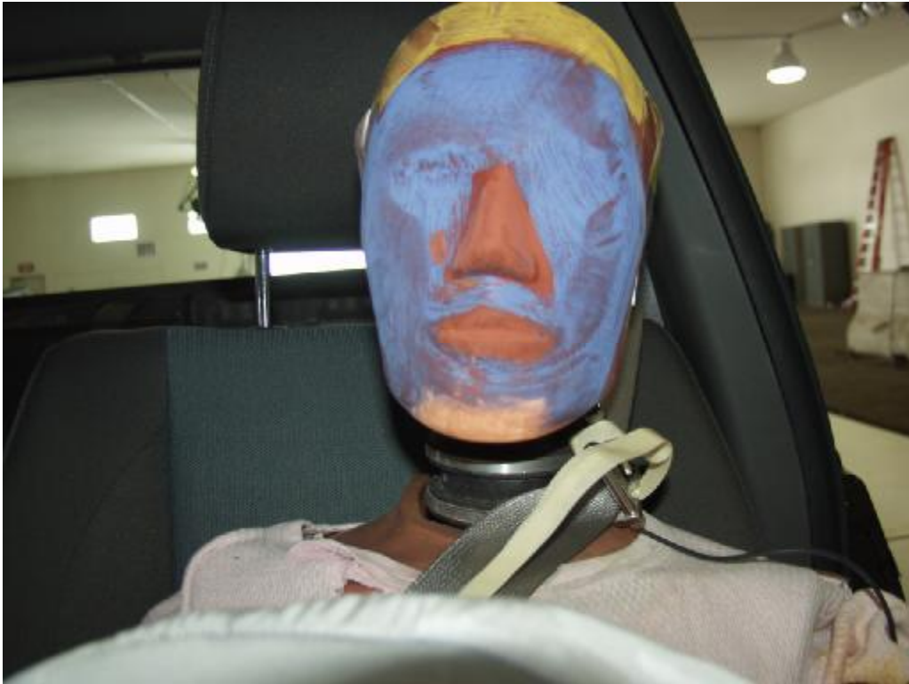
Figure A-42: Post-Test Driver Head View
