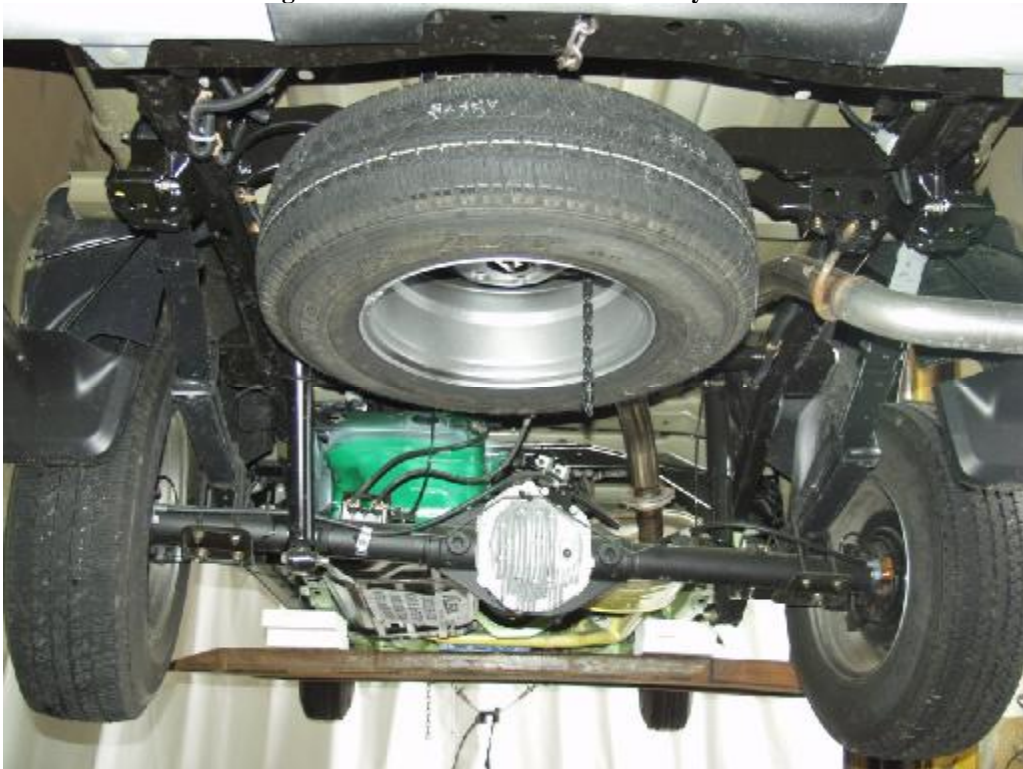
Figure A-29: Post-Test Rear Underbody View
