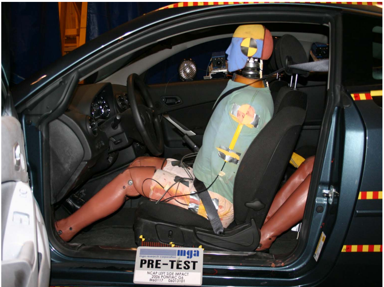
Pre-Test Driver Dummy (Door Open)
