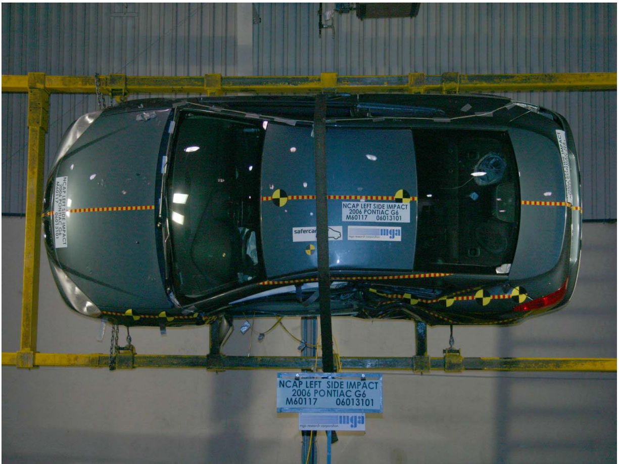
Vehicle on Rollover Device (270 Degrees)
