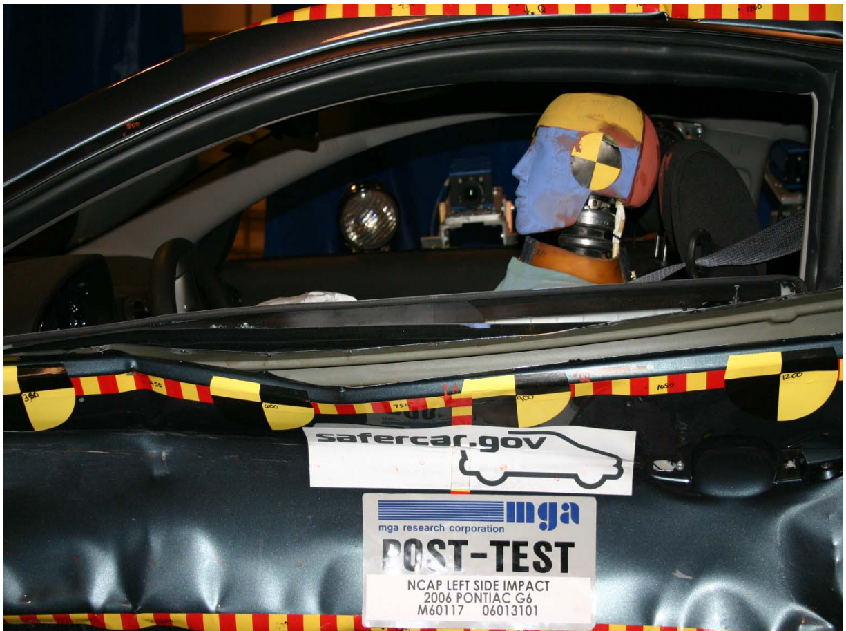
Post-Test Driver Dummy (Through Window)
