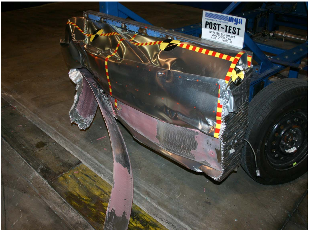
Post-Test Left Side View of Deformable Barrier
