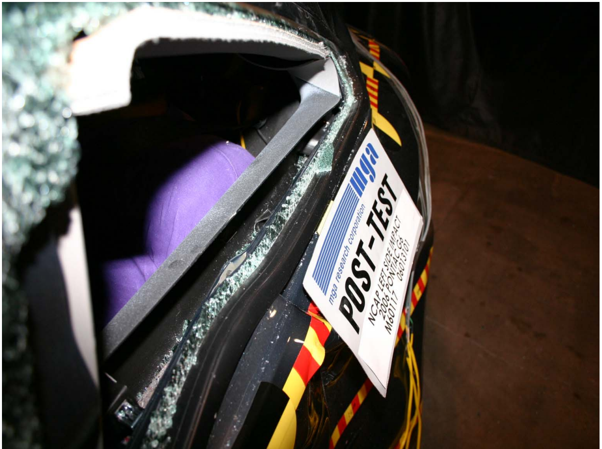
Post-Test Passenger Dummy Clearance From Door
