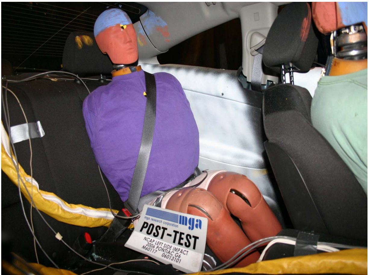
Post-Test Passenger Dummy Right Side View
