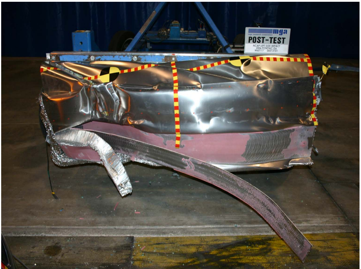
Post-Test Front View of Deformable Barrier
