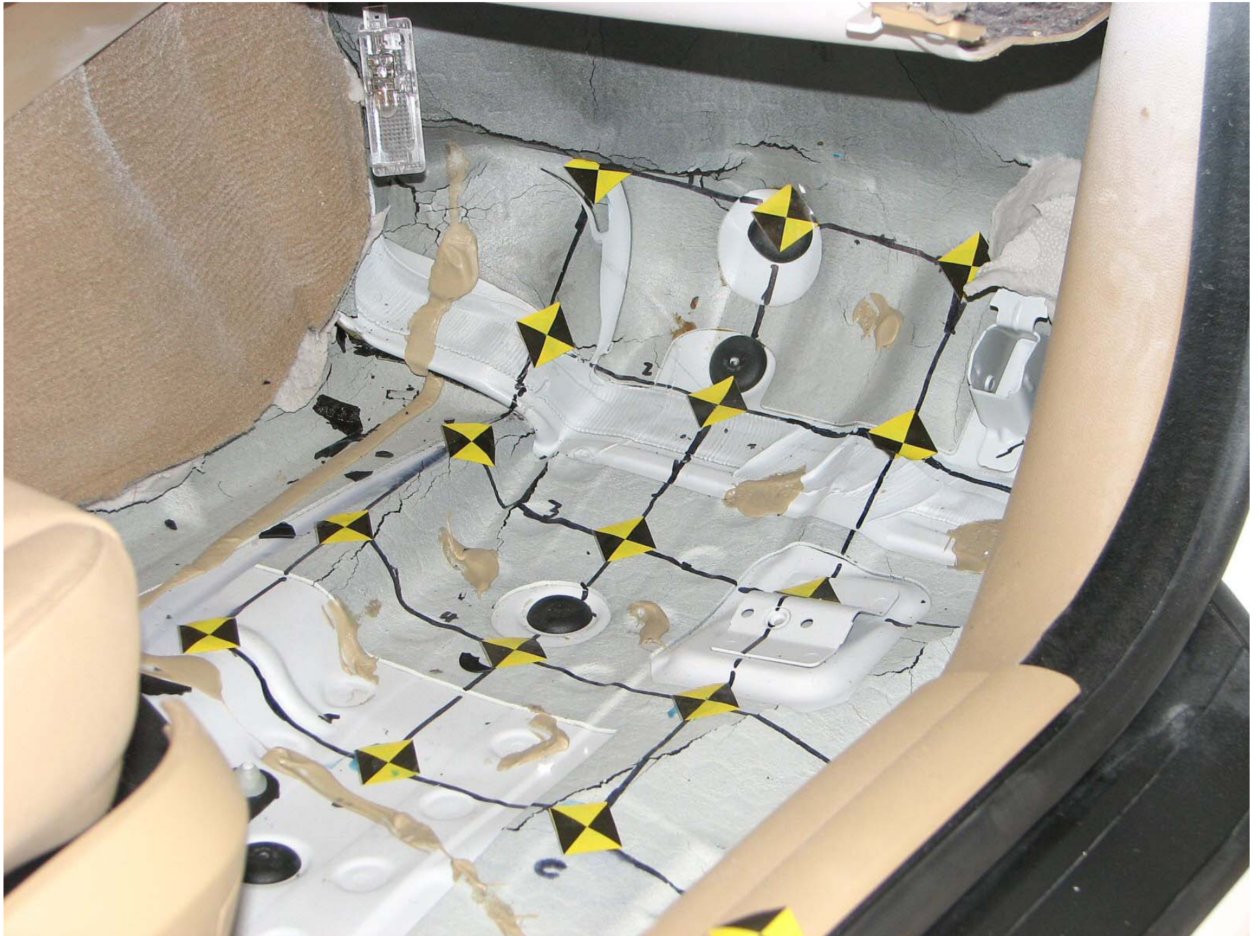
Figure A-55: Post-Test Passenger Side Floor Pan
