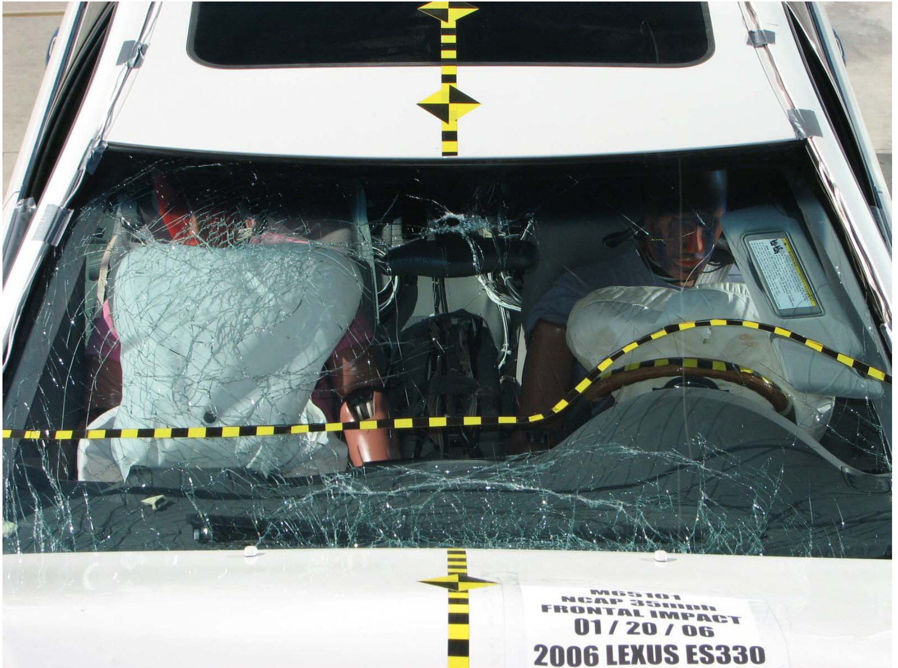
Figure A-19: Post-Test Windshield
