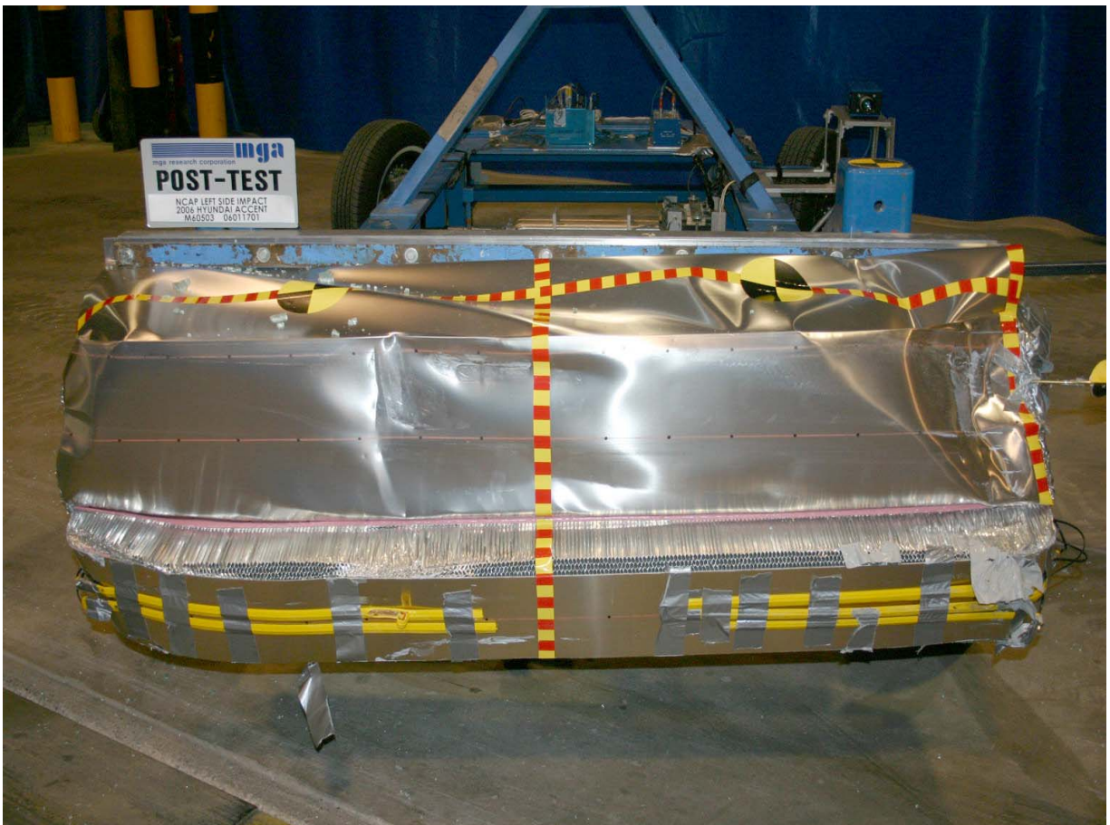
Post-Test Front View of Deformable Barrier
