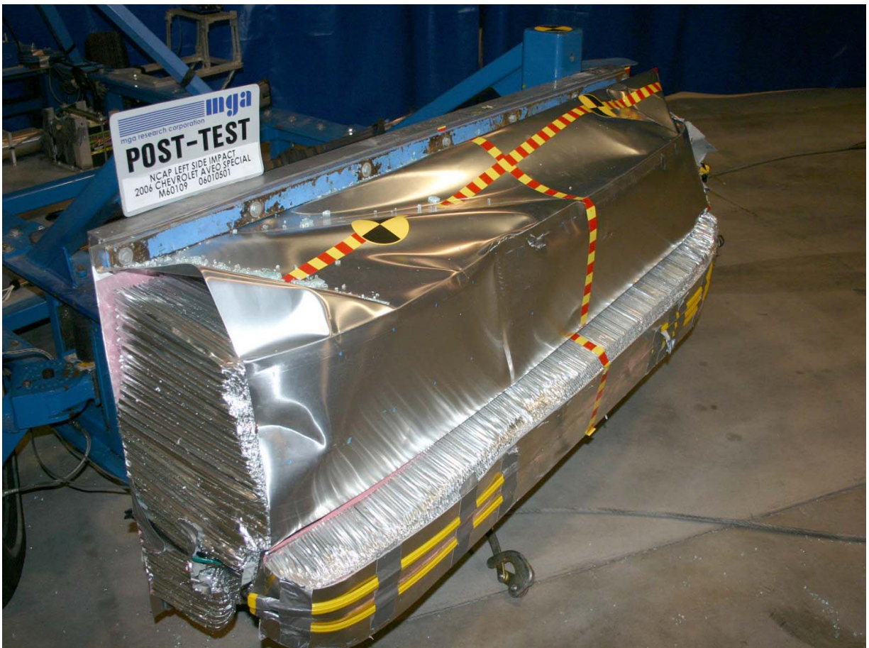
Post-Test Right Side View of Deformable Barrier
