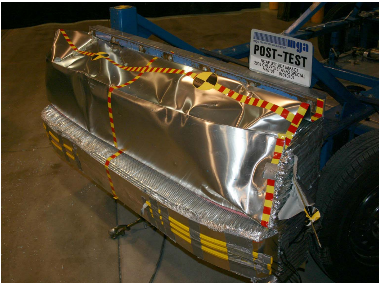
Post-Test Left Side View of Deformable Barrier
