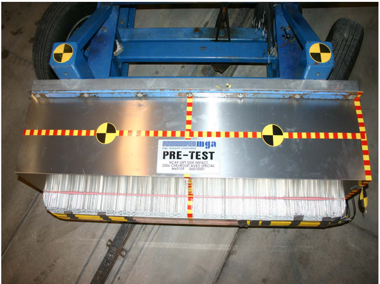
Pre-Test Top View of Deformable Barrier
