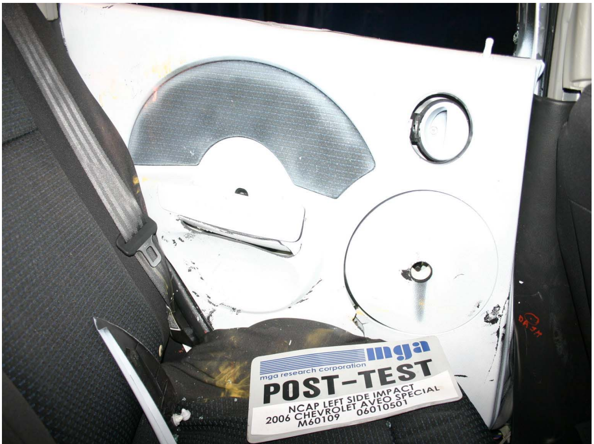
Post-Test Passenger Dummy Torso Contact
