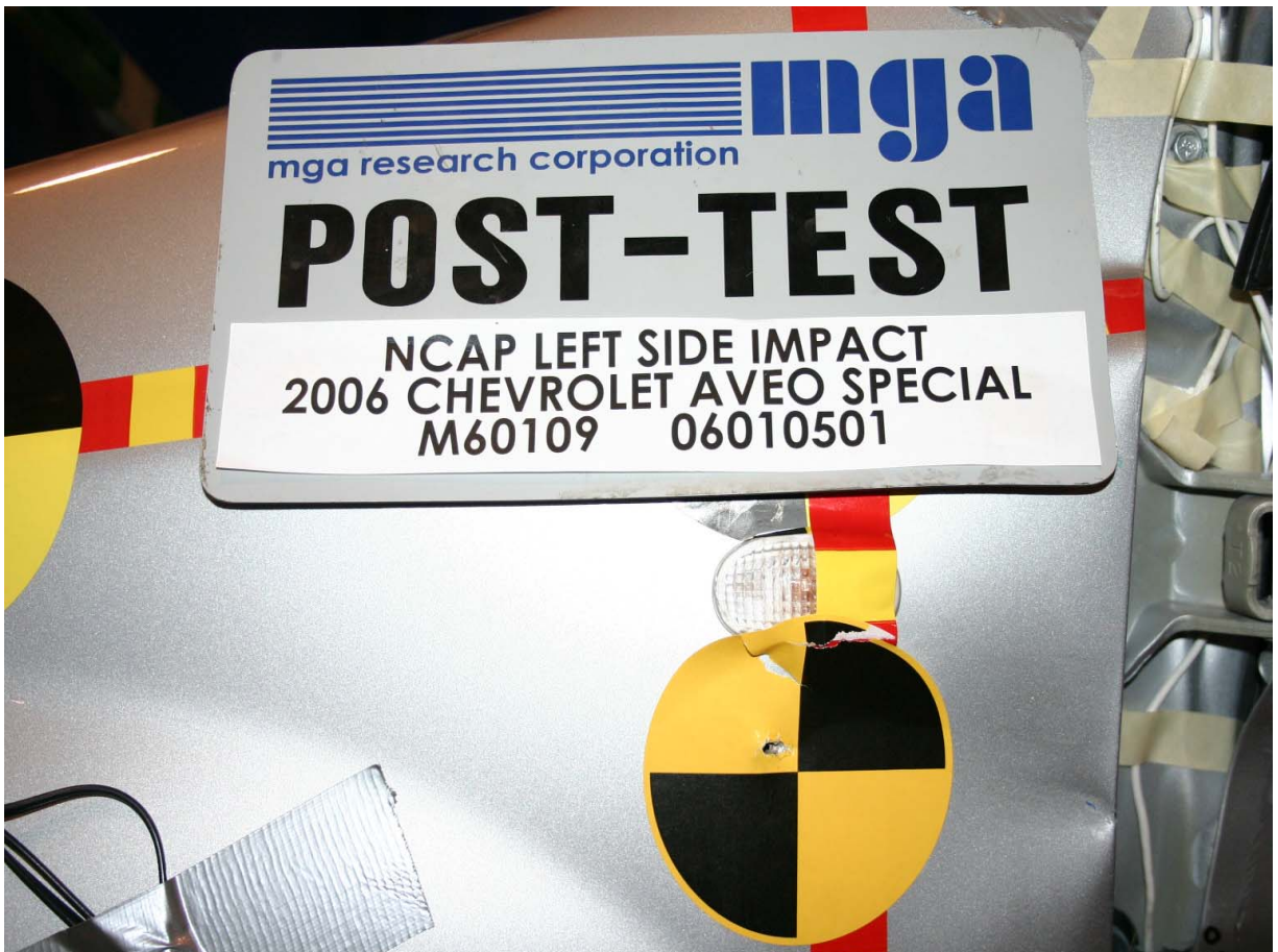
Post-Test Left Impact Point
