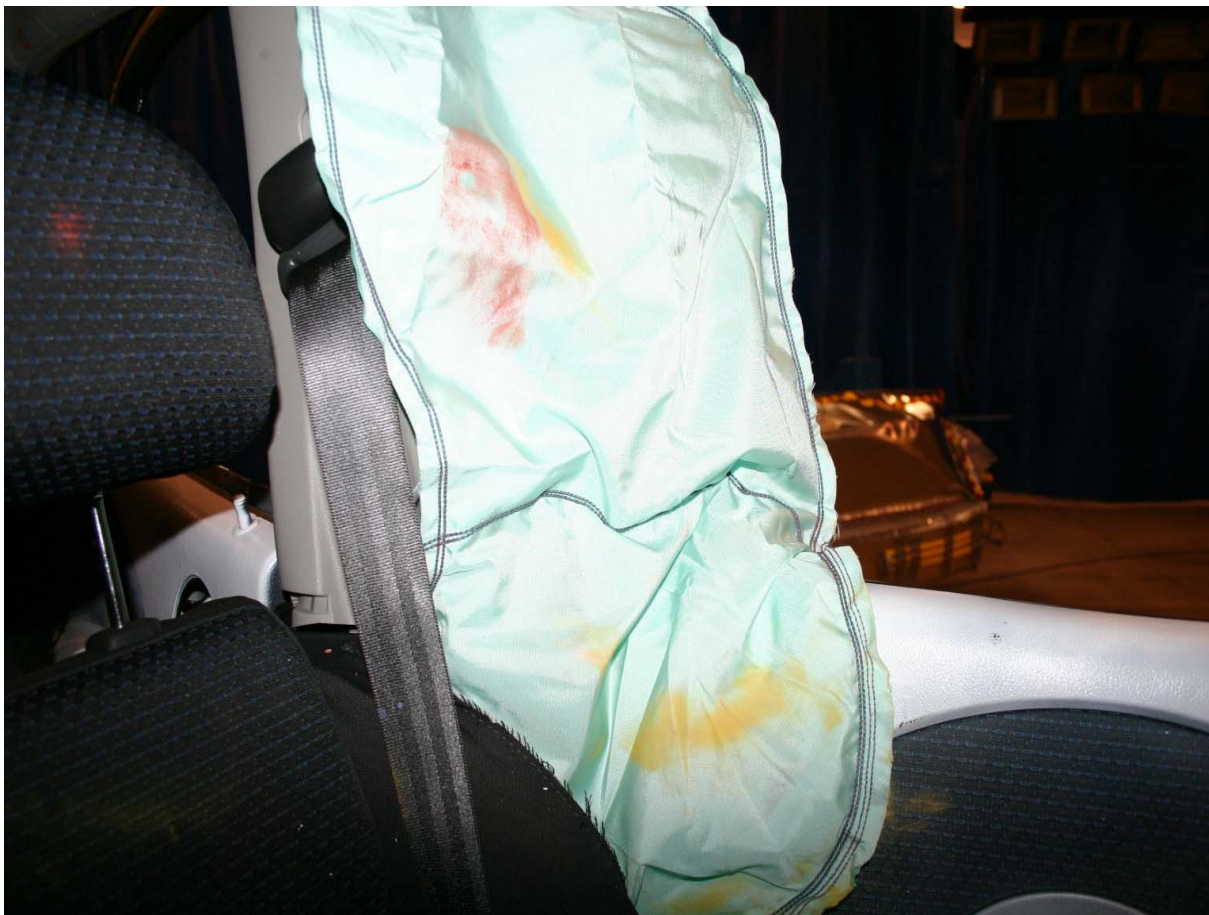
Post-Test Driver Dummy Torso Contact
