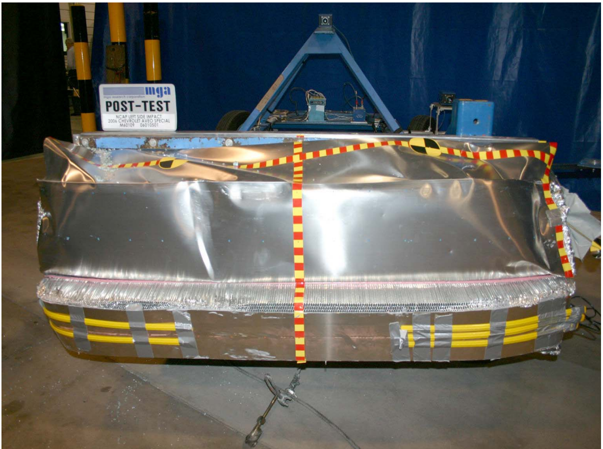
Post-Test Front View of Deformable Barrier
