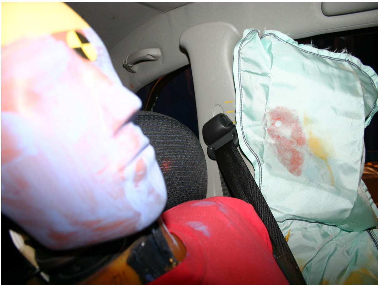
Post-Test Driver Dummy Head Contact
