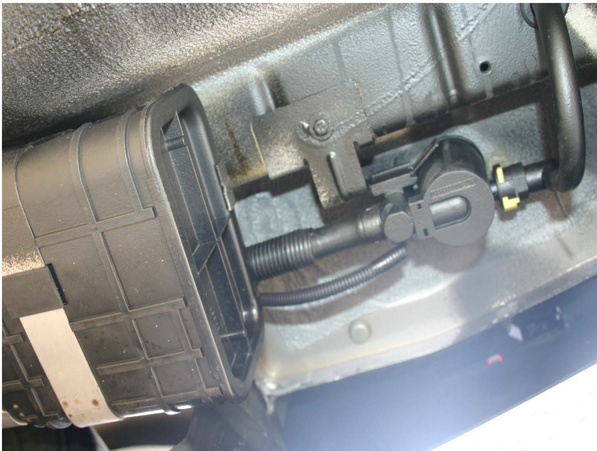
Fuel Leakage Location View #1
