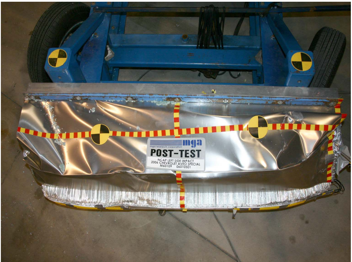
Post-Test Top View of Deformable Barrier
