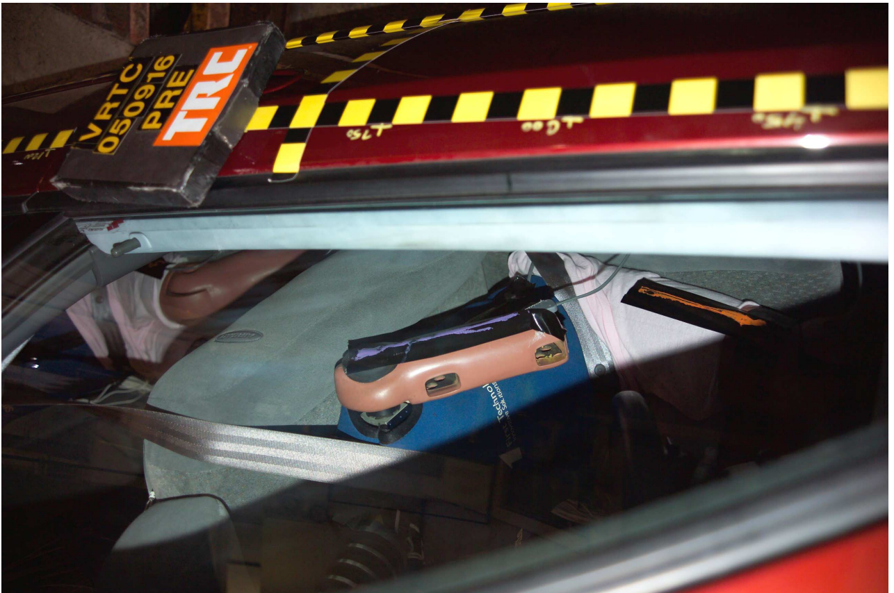
Figure A-52 Pre-Test Left View of Front SID-II and Door Clearance
