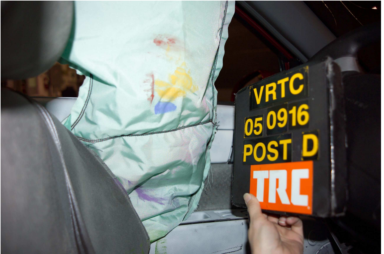
Figure A-61 Post-Test Front SID-IIs Contact - View 1
