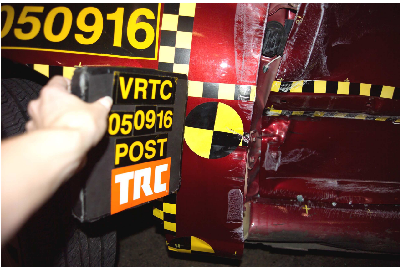
Figure A-40 Post-Test Primary Impact Point View
