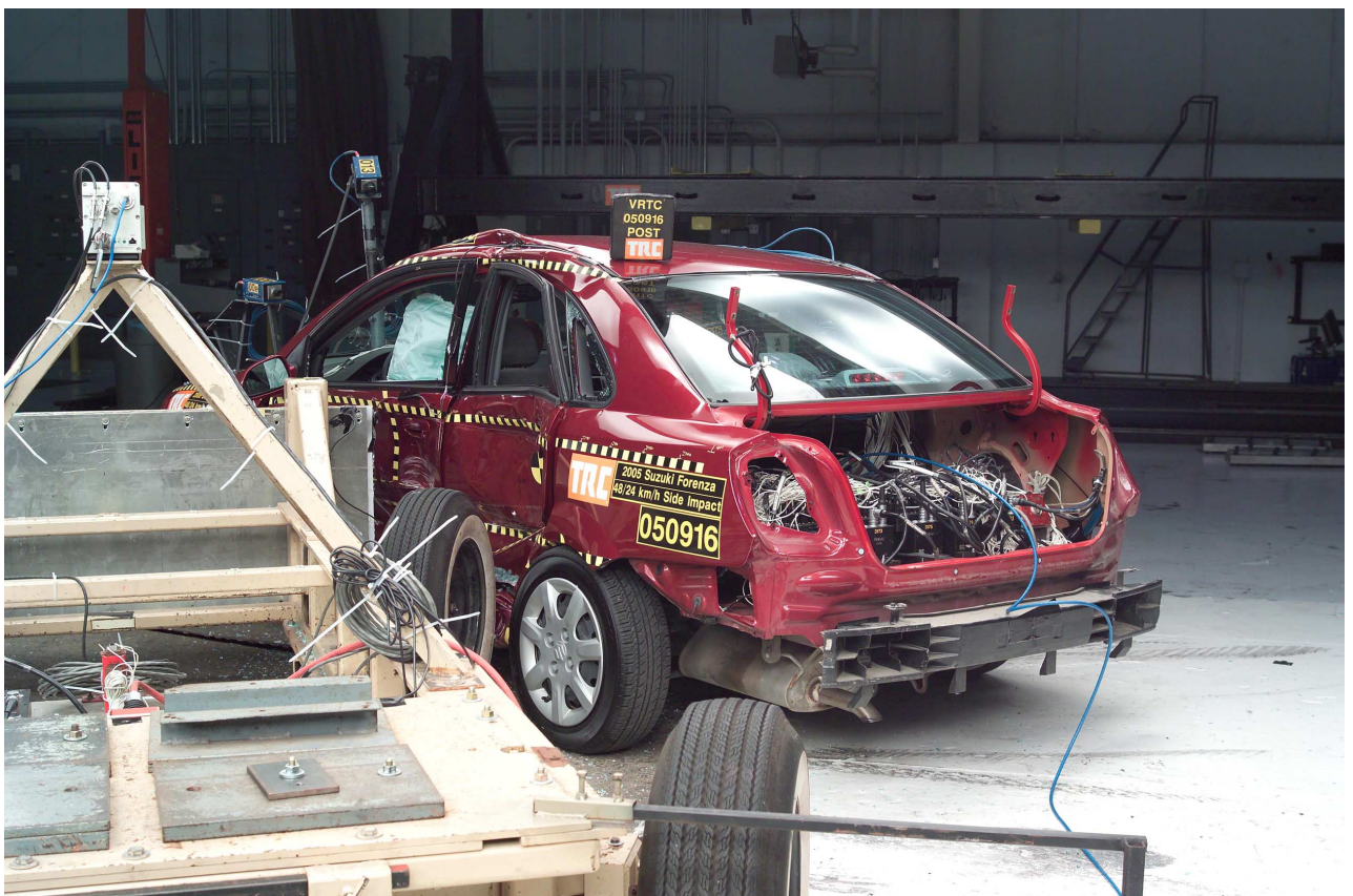
Figure A-26 Post-Test Right Side View of MDB with Impactor Face in Position
