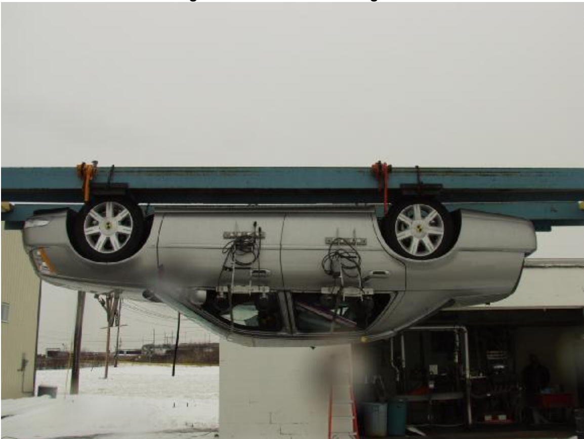
Figure A-52: Rollover 180 Degrees
