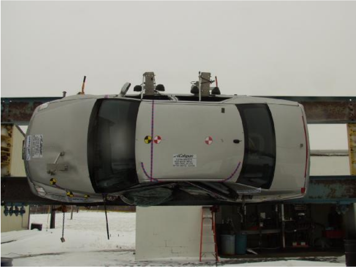
Figure A-51: Rollover 90 Degrees
