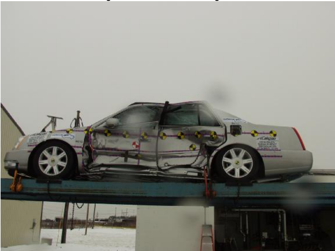
Figure A-54: Rollover 360 Degrees
