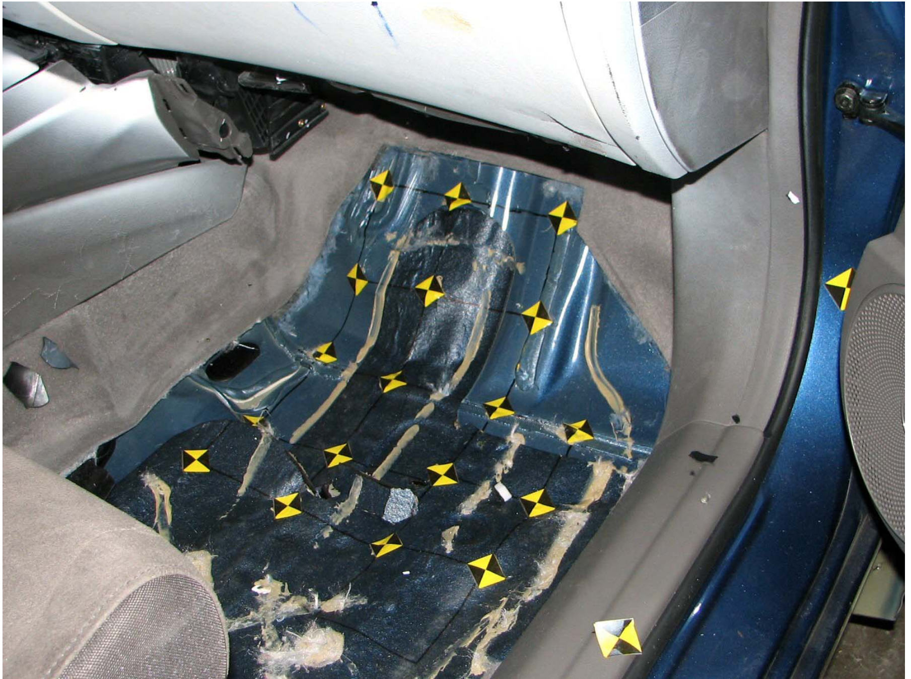
Figure A-55: Post-Test Passenger Side Floor Pan
