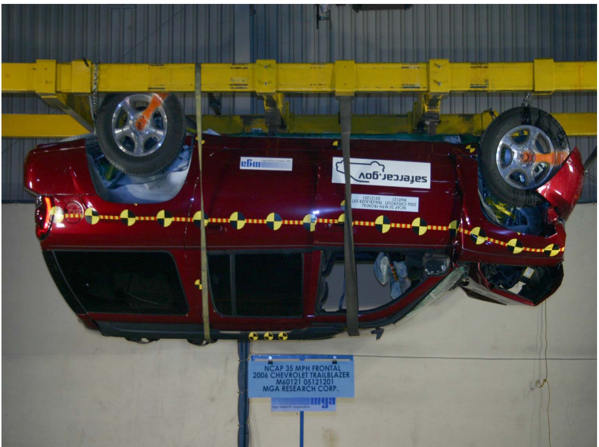
Vehicle on Rollover Device at 180 Degrees
