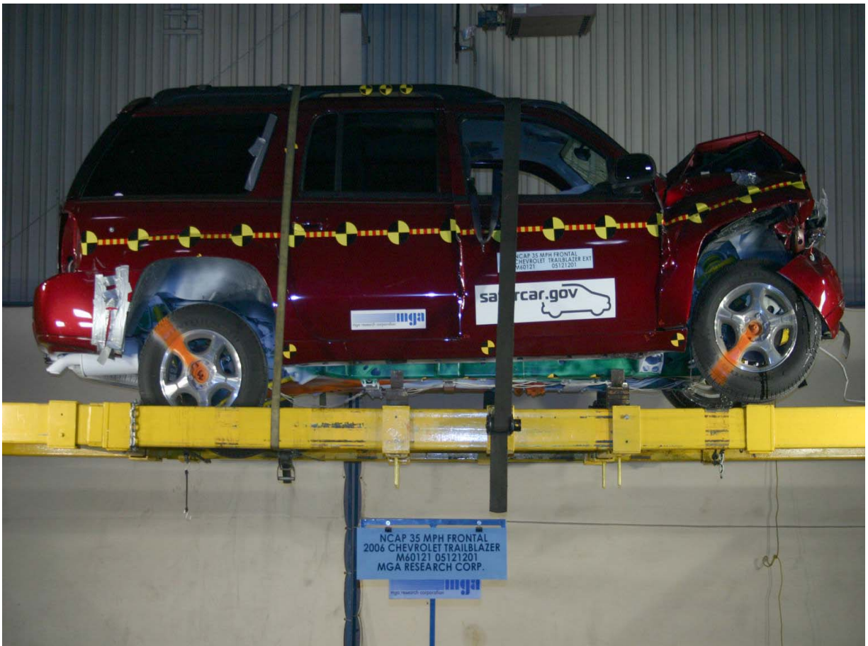
Vehicle on Rollover Device at 360 Degrees
