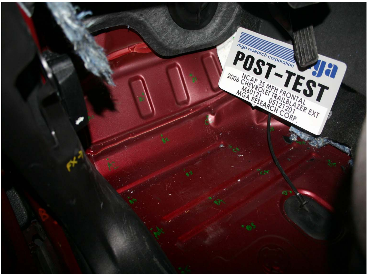
Post-Test Driver Side Floor Pan
