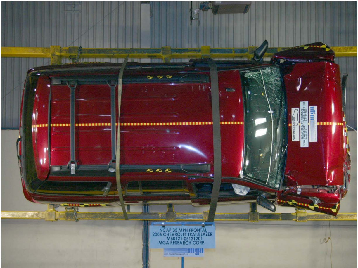
Vehicle on Rollover Device at 270 Degrees
