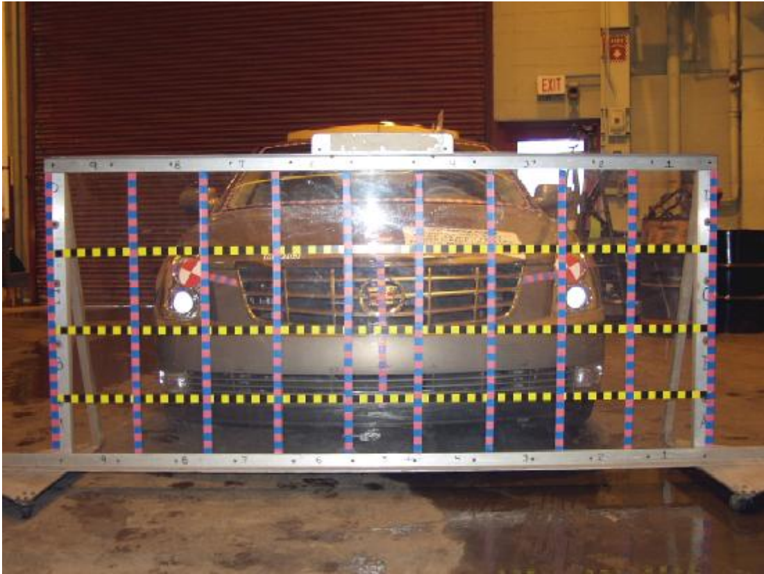
Figure A-1: Load Cell Locations
