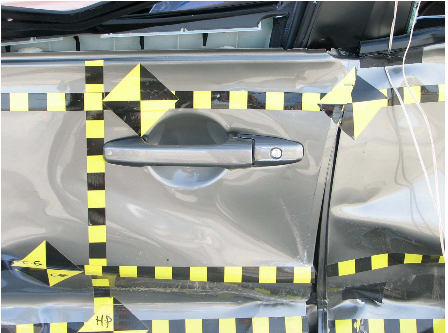
Figure A-32: Post-Test Left Front Door
