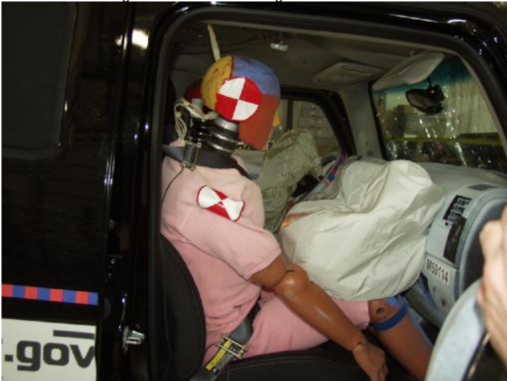
Figure A-49: Post-Test Passenger and Interior View
