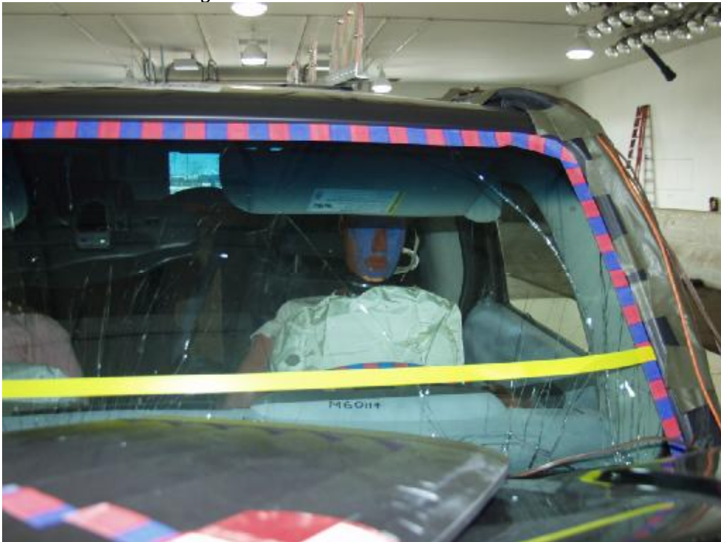
Figure A-31: Post-Test Driver Head Location
