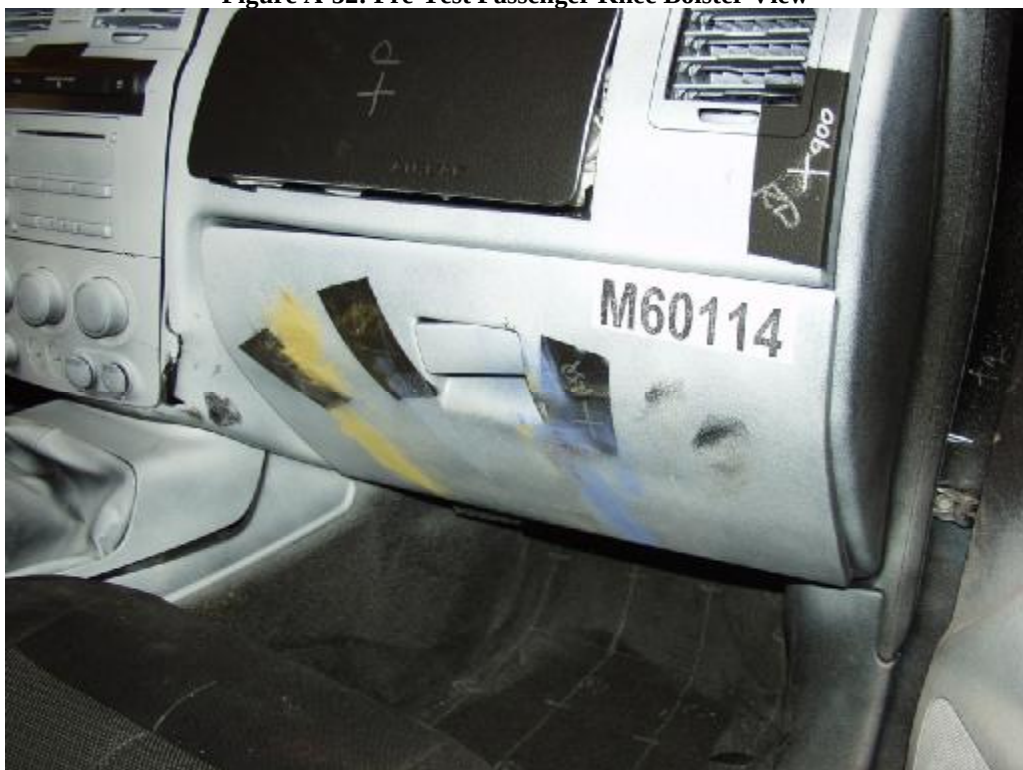
Figure A-53: Post-Test Passenger Knee Bolster View
