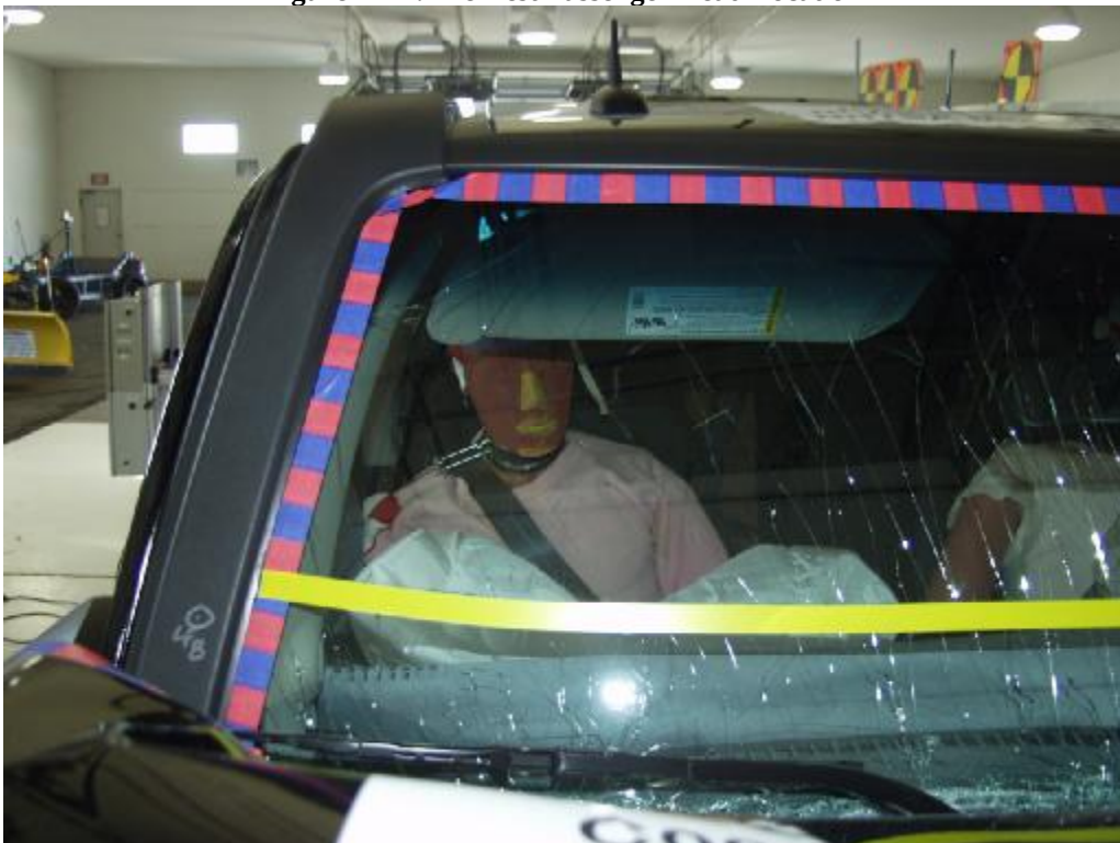
Figure A-45: Post-Test Passenger Head Location
