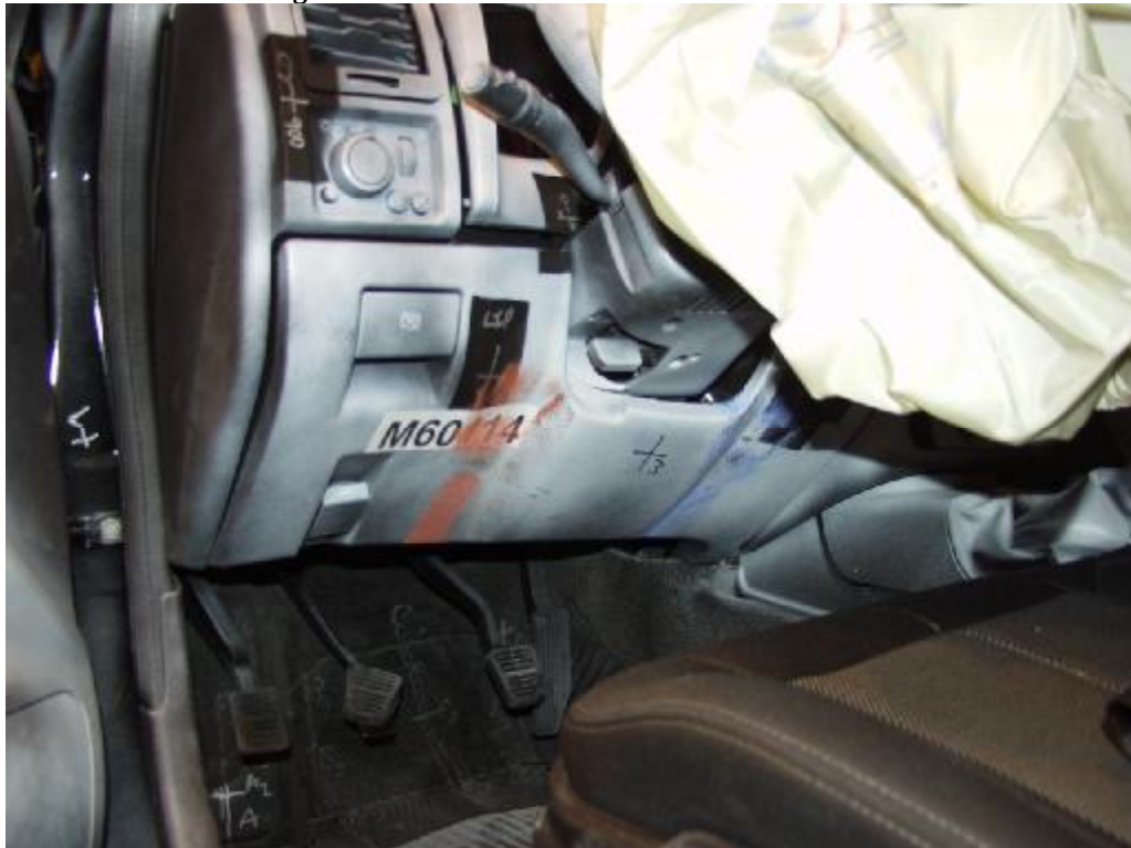
Figure A-39: Post-Test Driver Knee Bolster View
