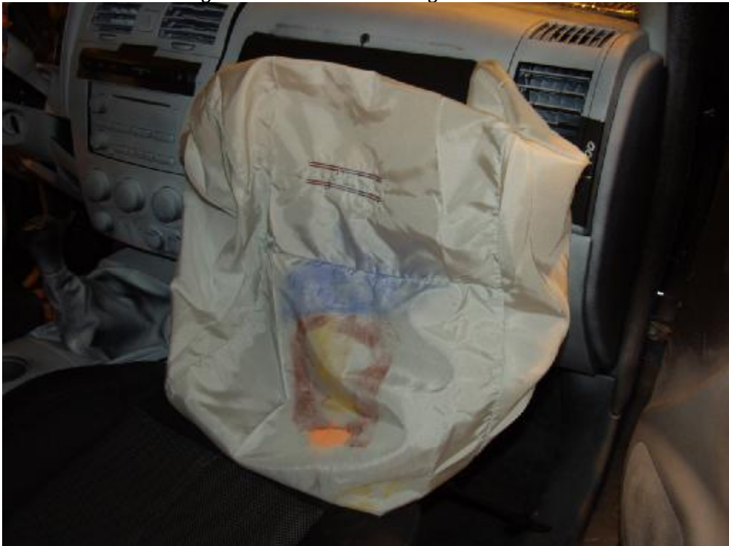
Figure A-57: Post-Test Passenger Contact to Airbag
