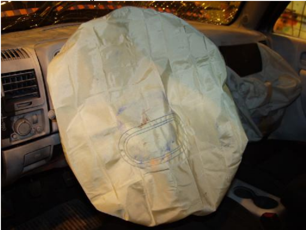
Figure A-43: Post-Test Driver Contact to Airbag
