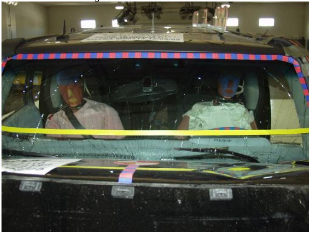
Figure A-19: Post-Test Windshield View
