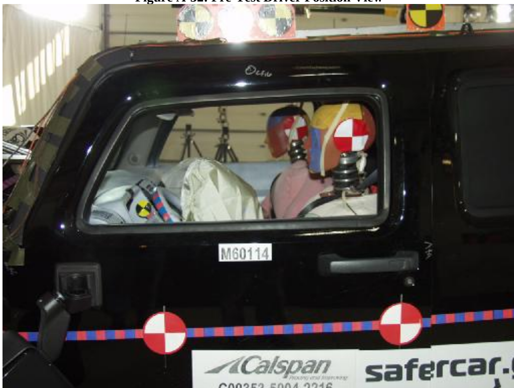
Figure A-33: Post-Test Driver Position View
