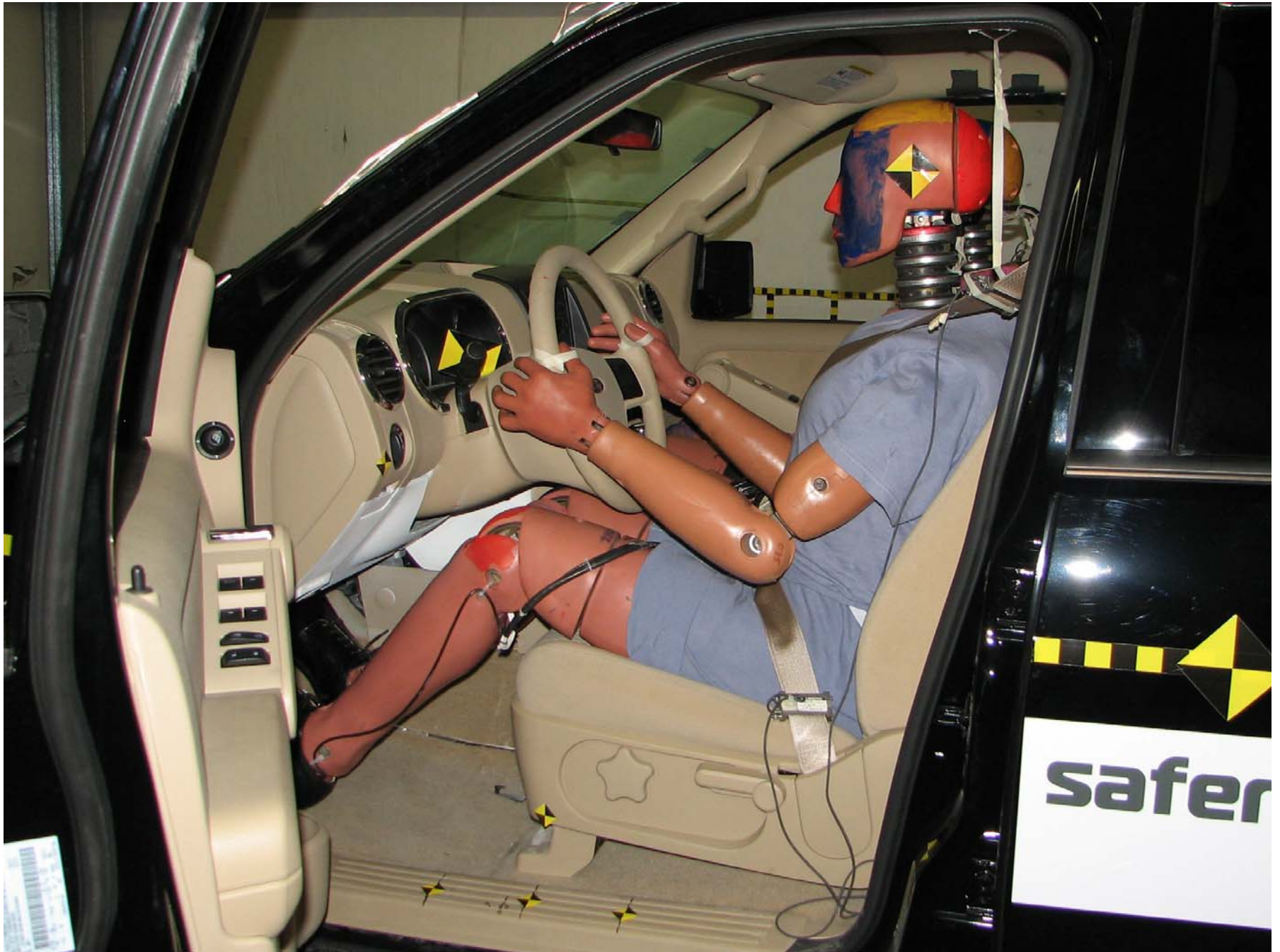
Figure A-34: Pre-Test Driver Dummy (Door Open)
