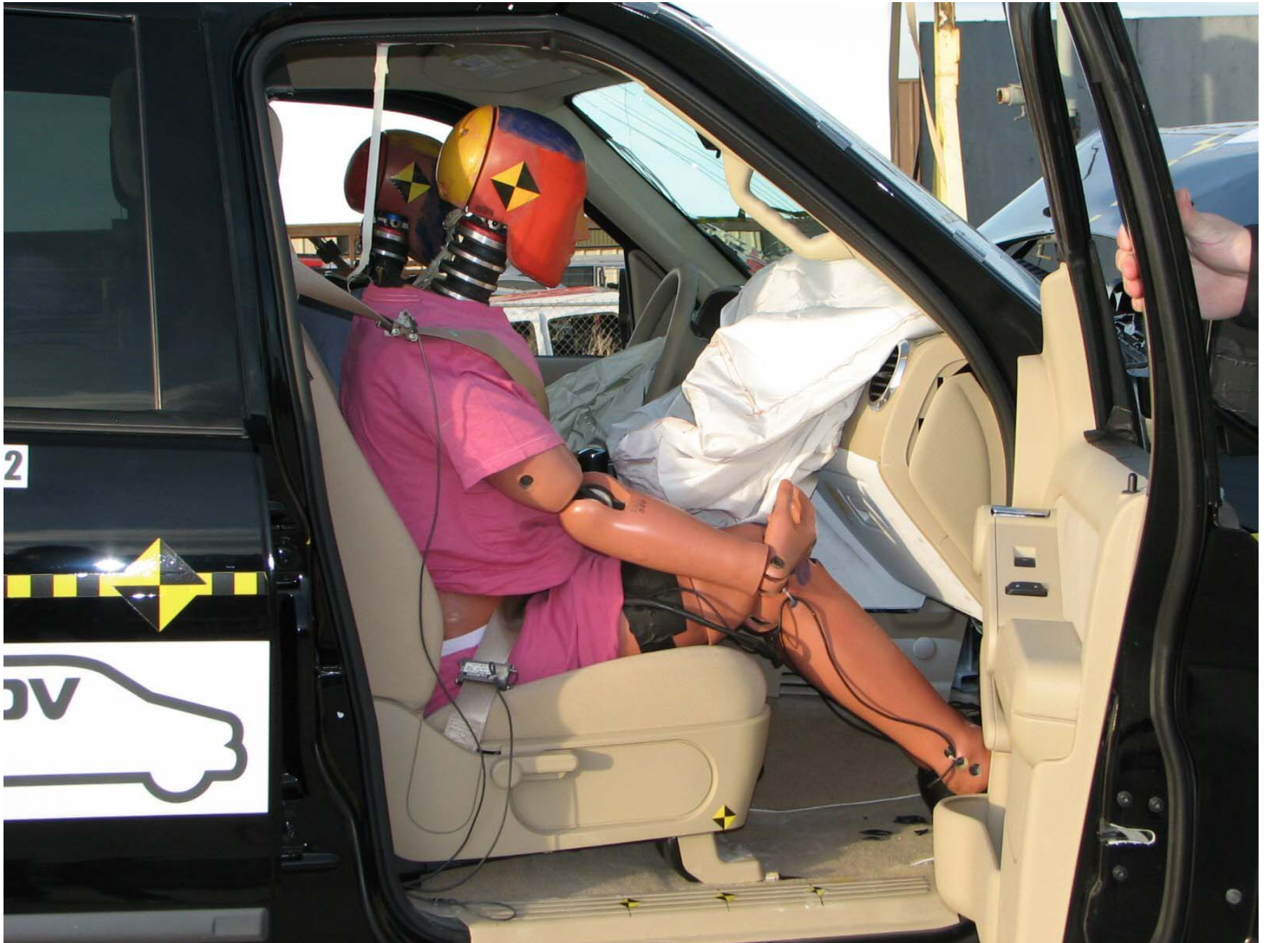
Figure A-49: Post-Test Passenger Dummy (Door Open)
