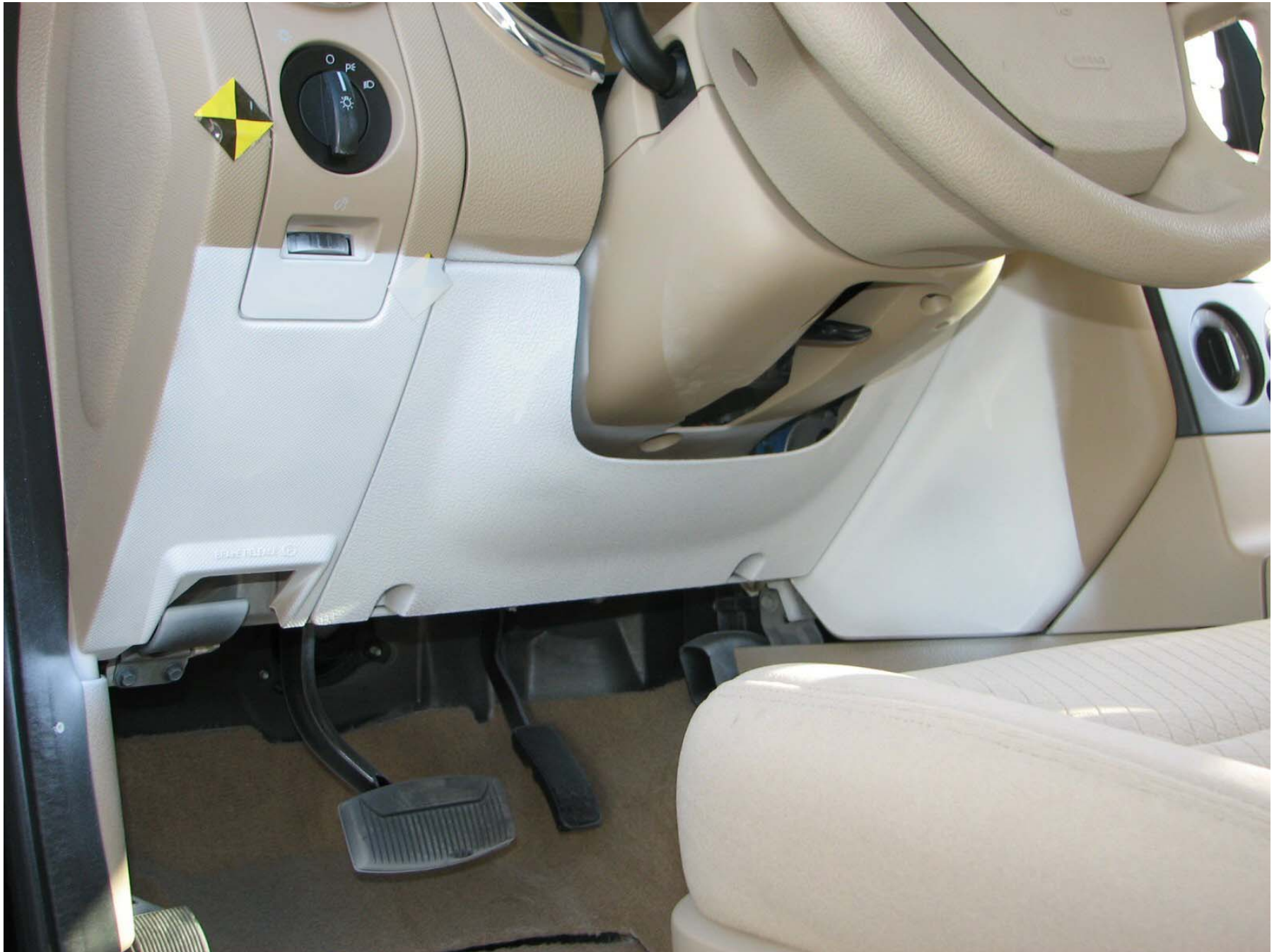
Figure A-38: Pre-Test Driver Side Knee Bolster
