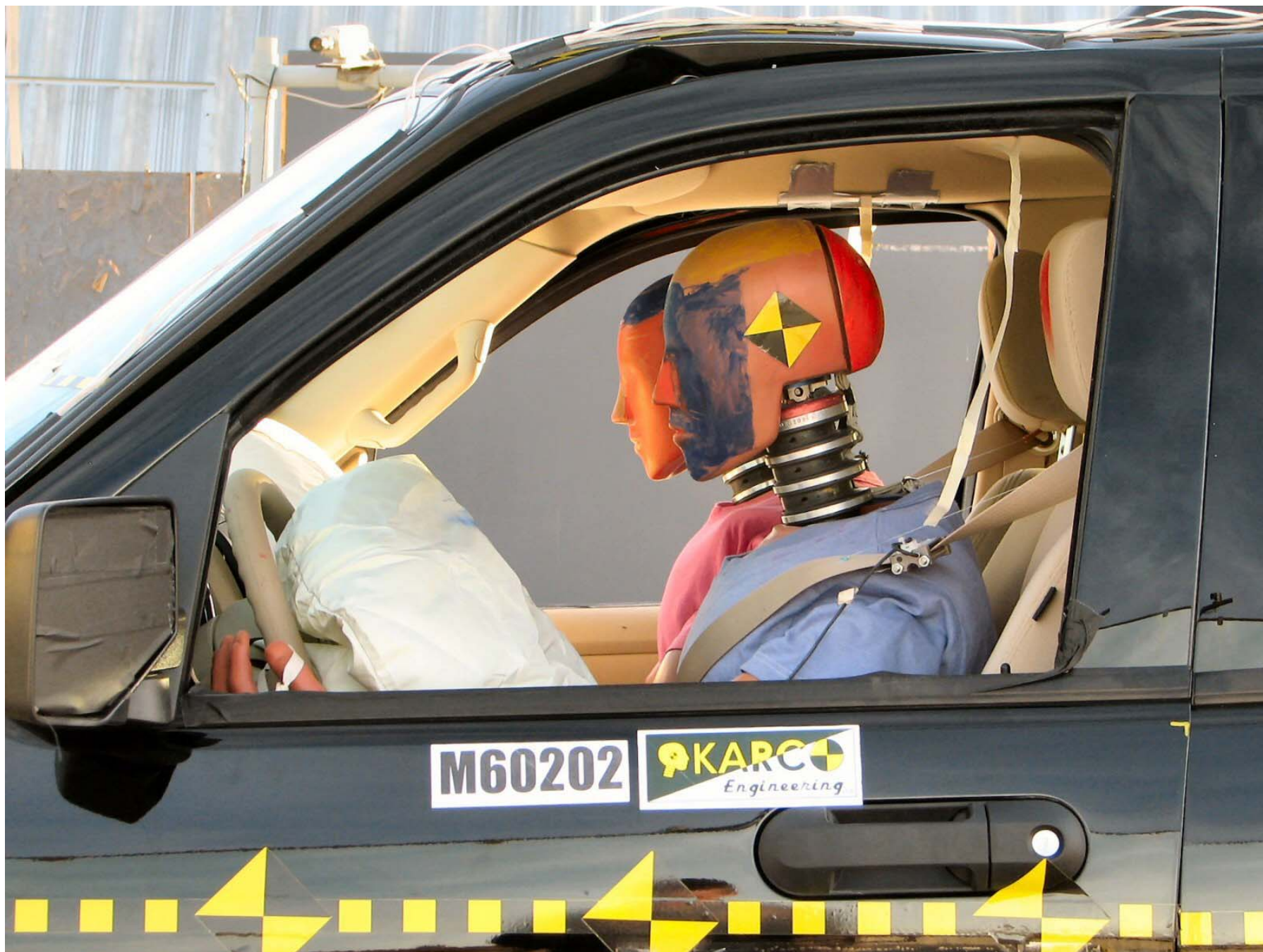
Figure A-33: Post-Test Driver Dummy (Through Window)
