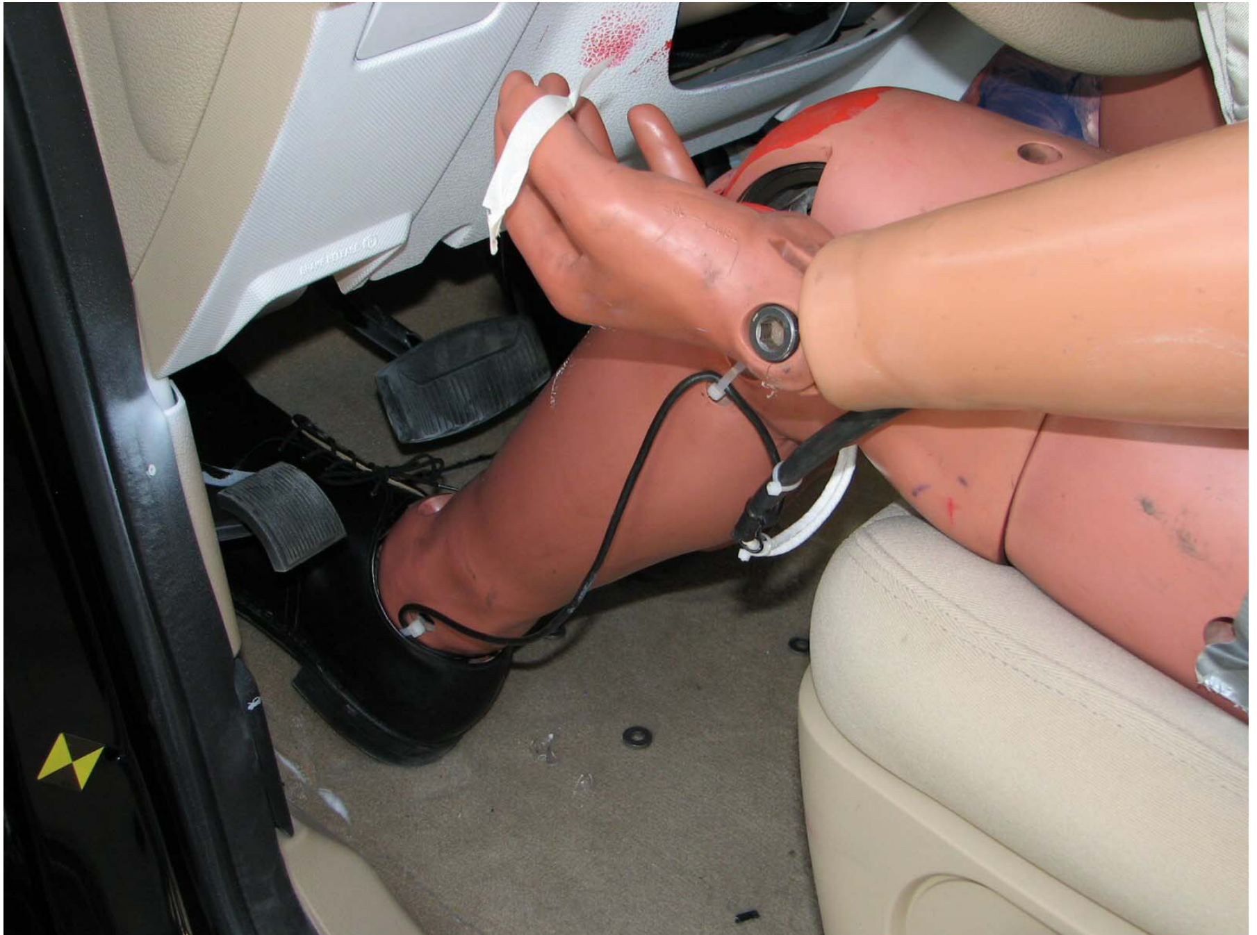
Figure A-37: Post-Test Driver Dummy Feet
