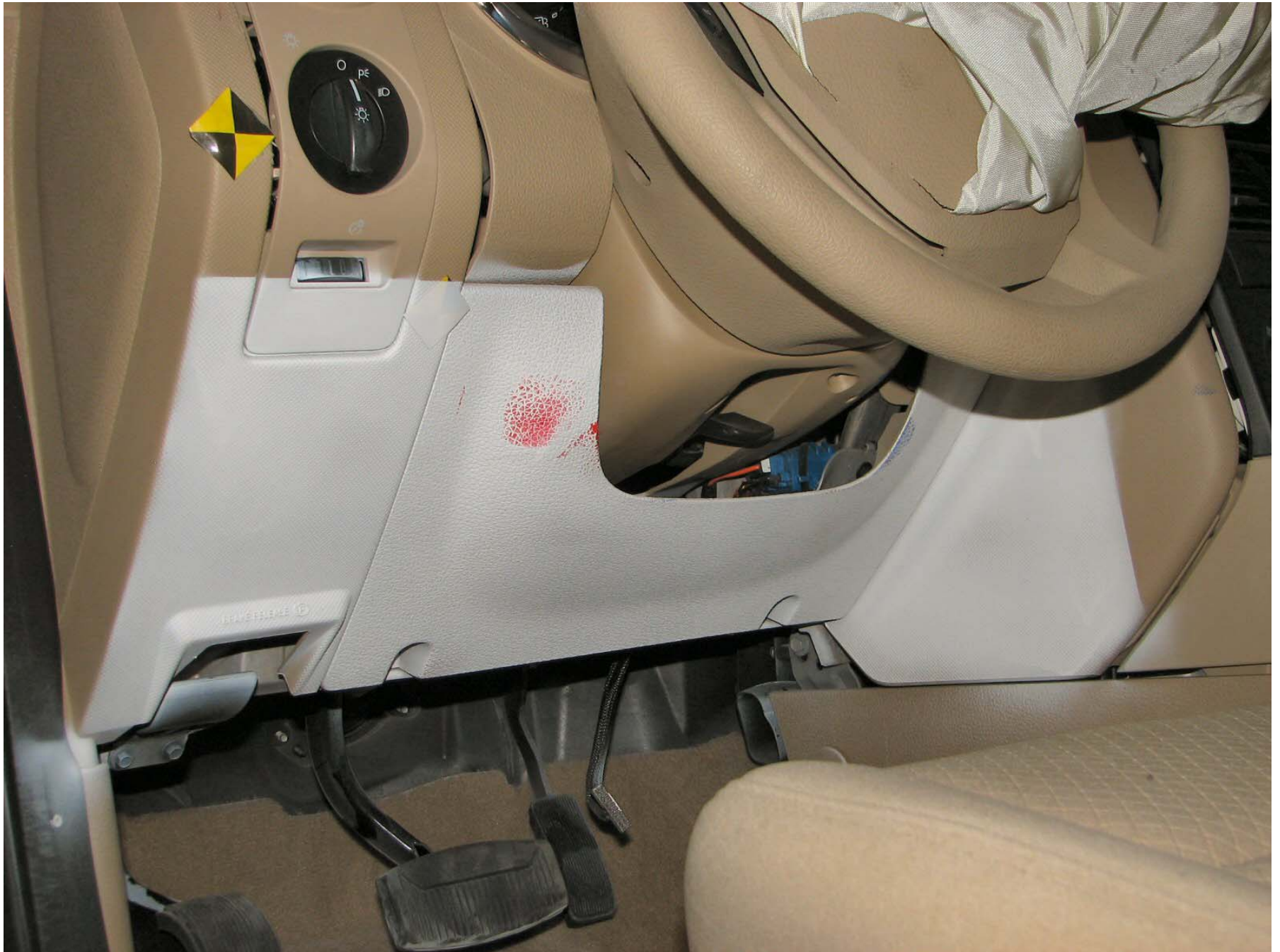
Figure A-39: Post-Test Driver Side Knee Bolster
