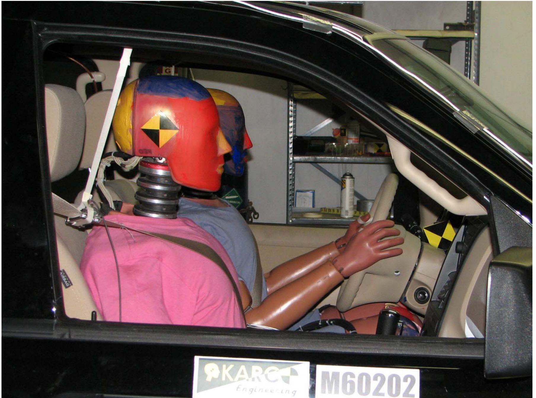
Figure A-46: Pre-Test Passenger Dummy (Through Window)
