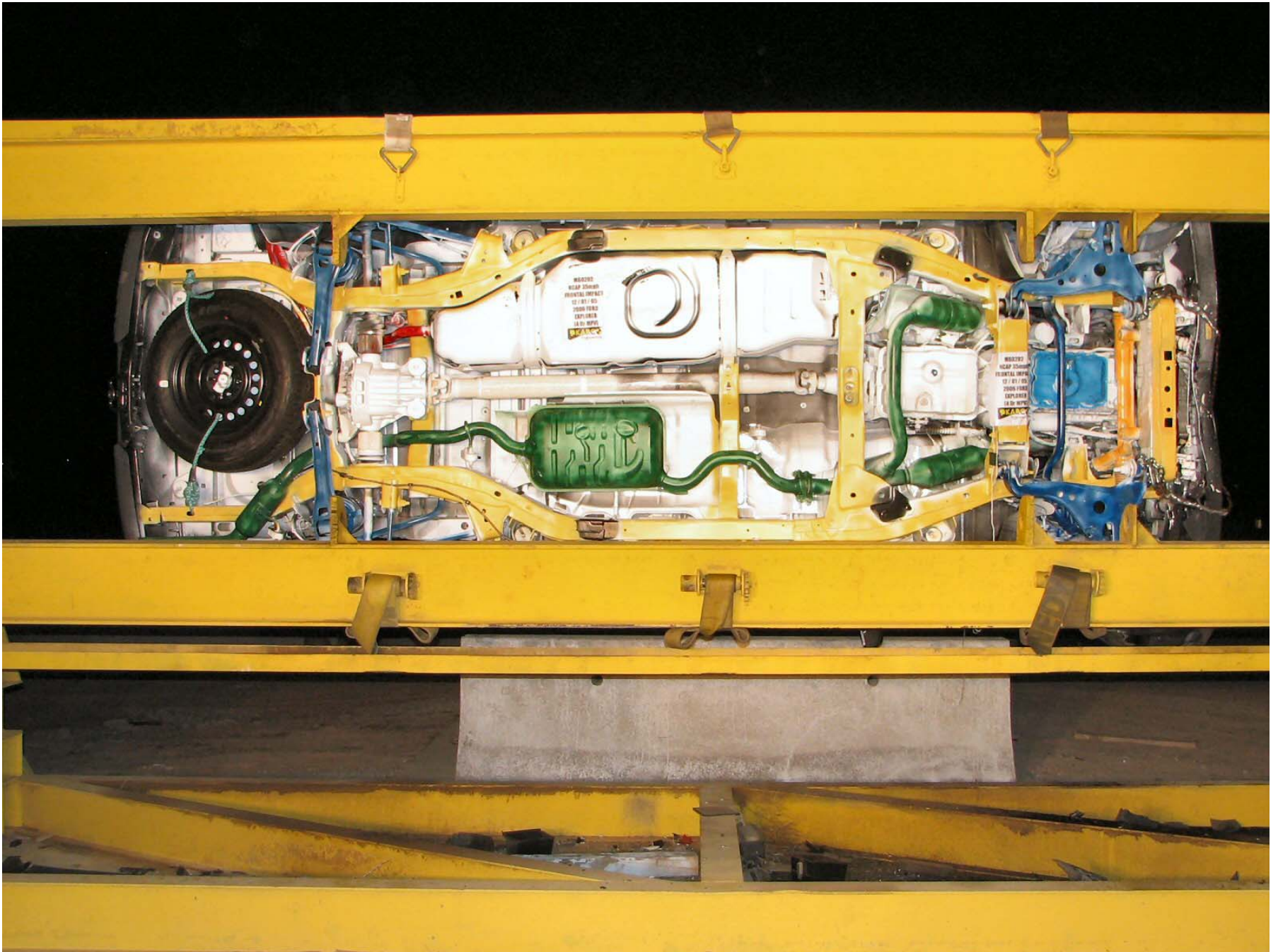
Figure A-61: Vehicle on Rollover Device (270°)
