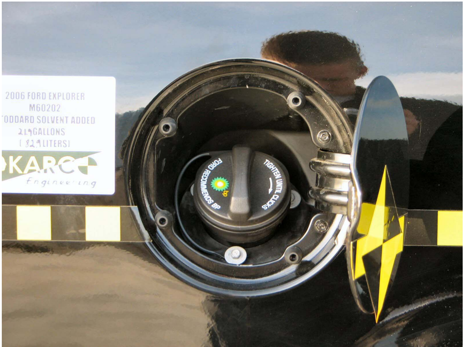
Figure A-23: Post-Test Fuel Cap
