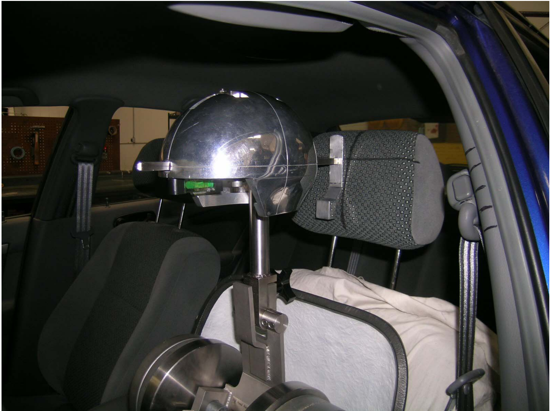
Figure A-29: Pre-Test Driver Seat ICBC Machine
