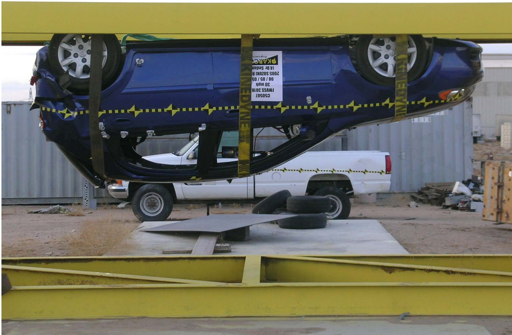
Figure A-45: Vehicle on Rollover Device 180°
