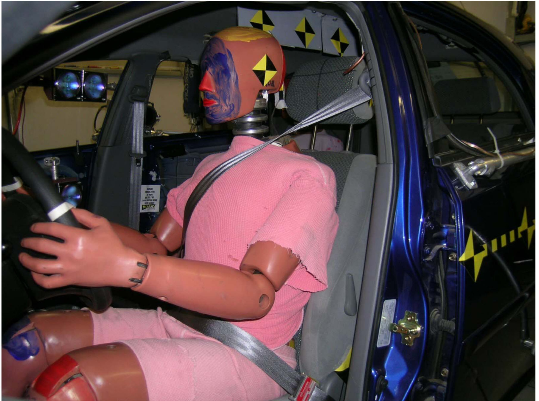
Figure A-35: Pre-Test Driver Dummy \frac{3}{4} View
