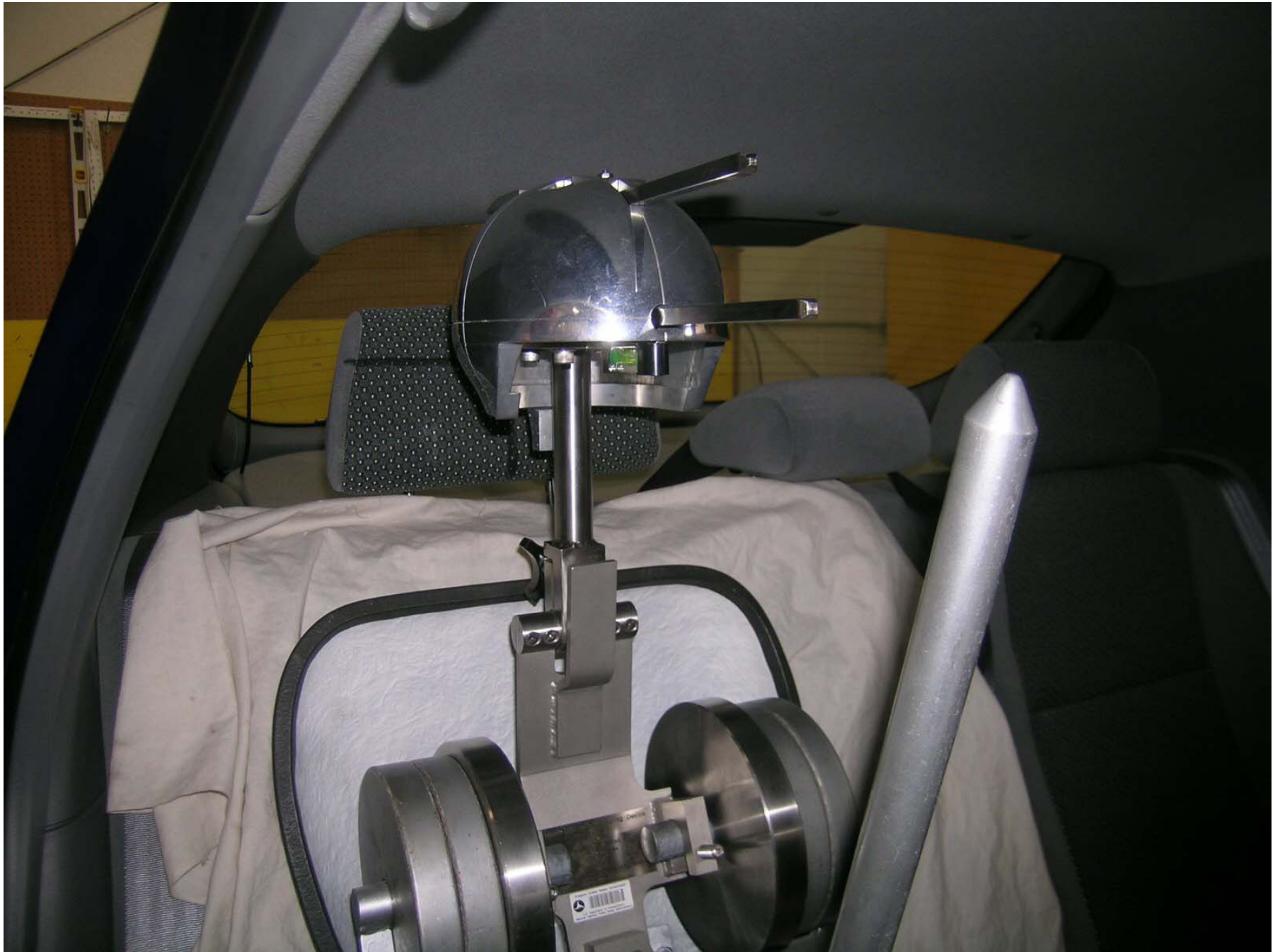
Figure A-30: Pre-Test Passenger Seat ICBC Machine
