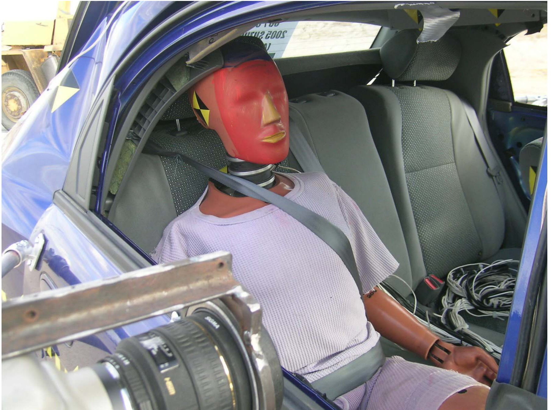
Figure A-42: Post-Test Passenger Dummy ¾ View
