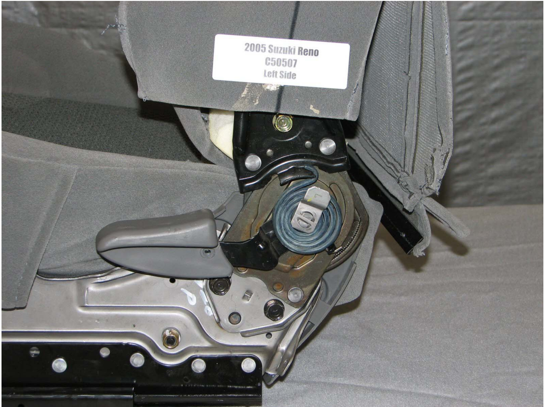
Figure A-48: Post-Test Driver Seat Left Side Reclining Mechanism
