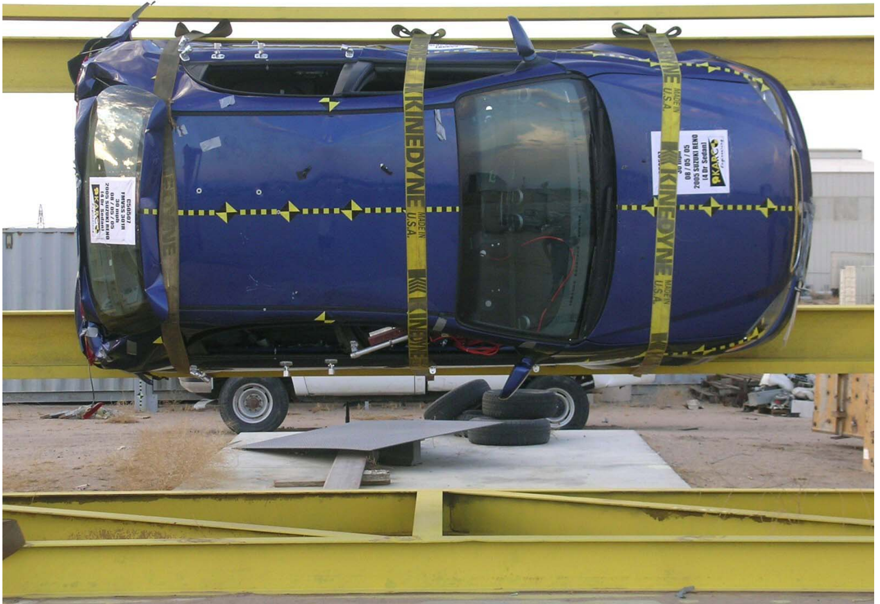
Figure A-44: Vehicle on Rollover Device 90°
