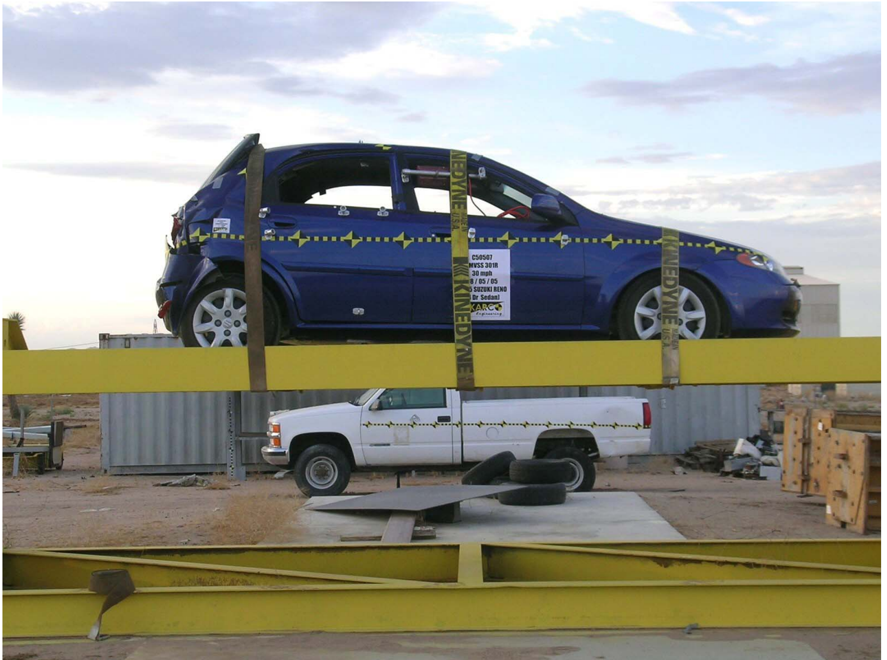
Figure A-43: Vehicle on Rollover Device 0°
