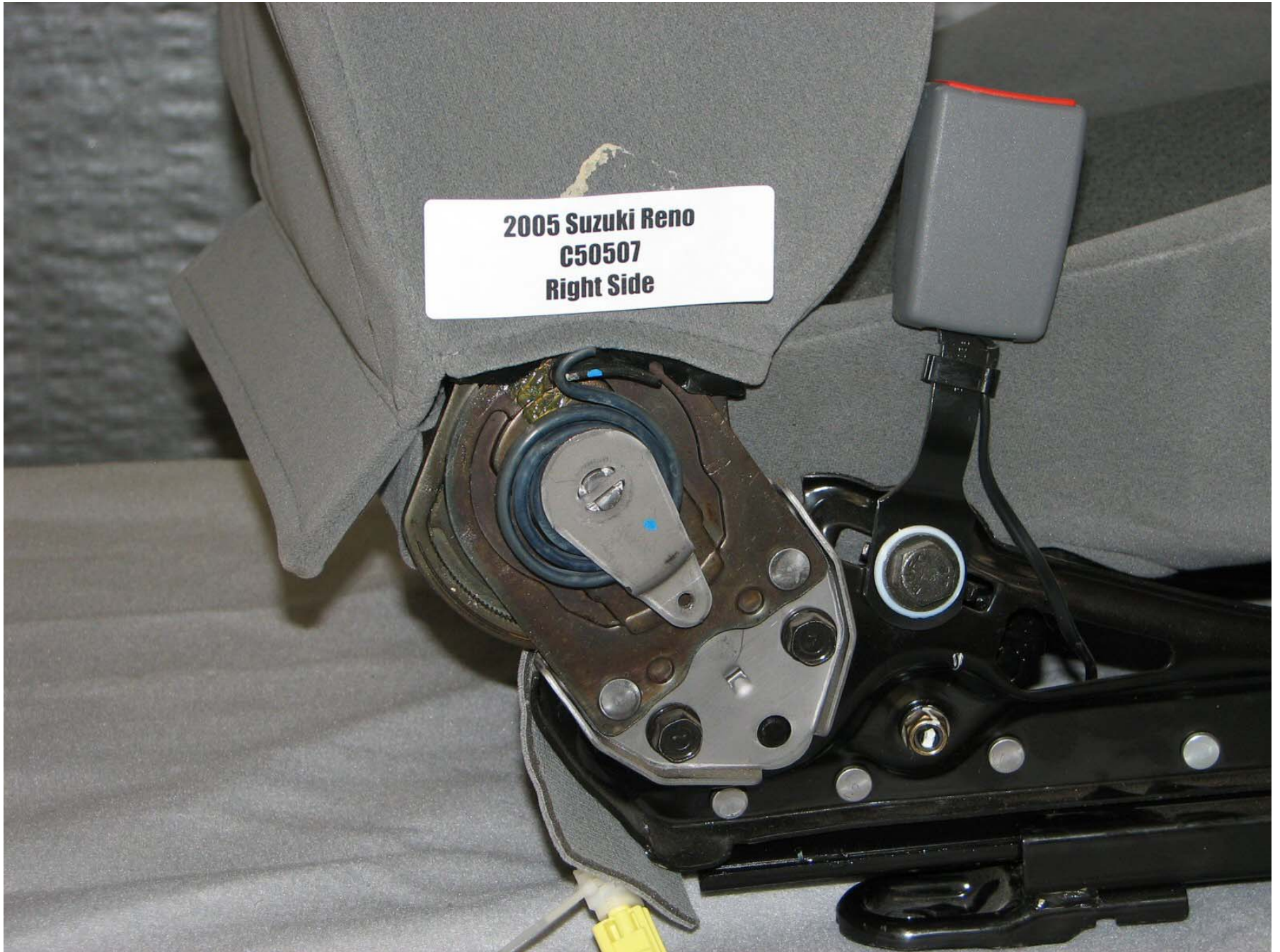
Figure A-49: Post-Test Driver Seat Right Side Reclining Mechanism
