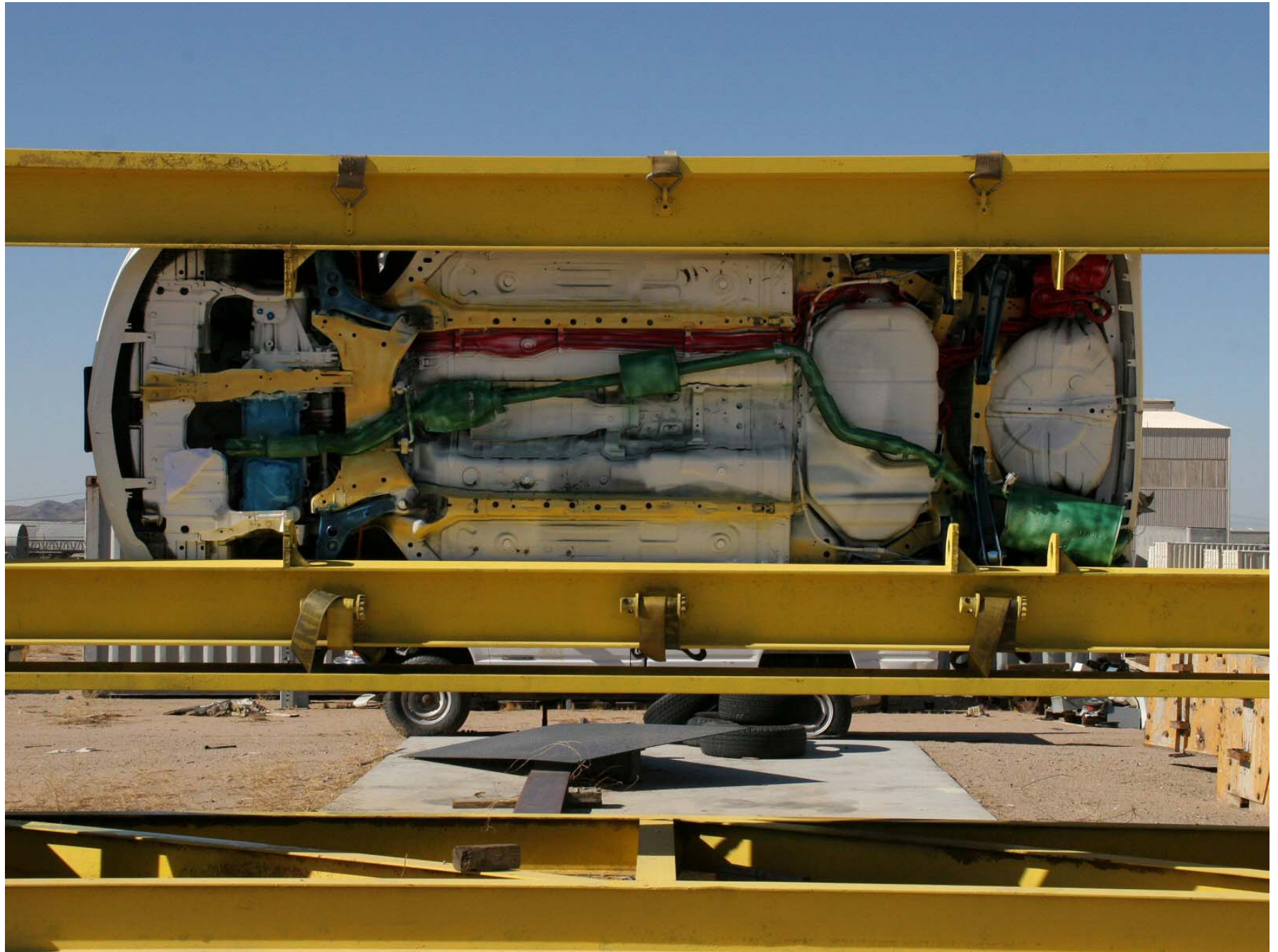
Figure A-24: Vehicle on Rollover Device at 270°
