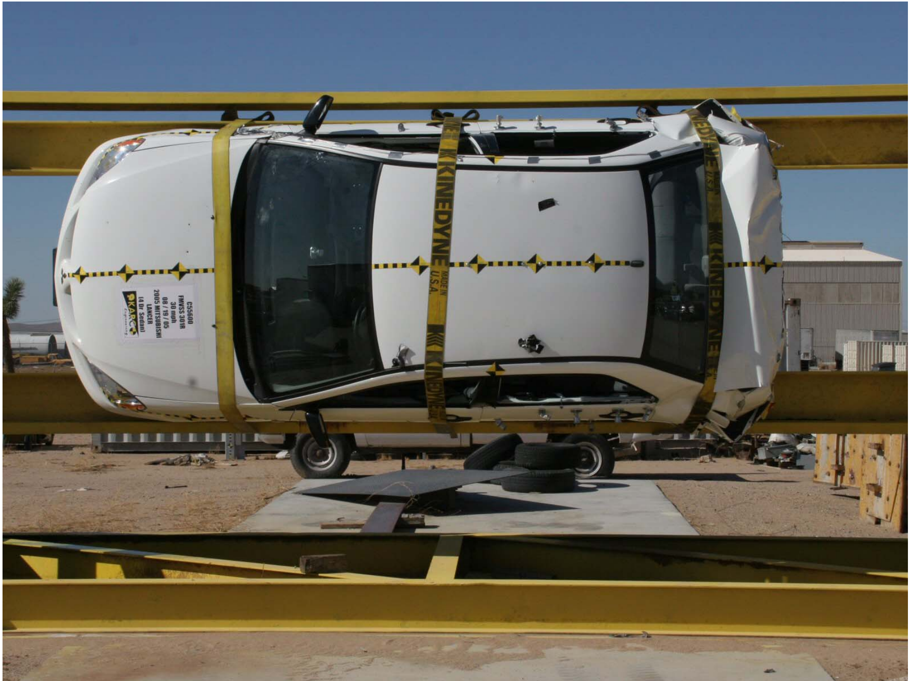
Figure A-22: Vehicle on Rollover Device at 90°
