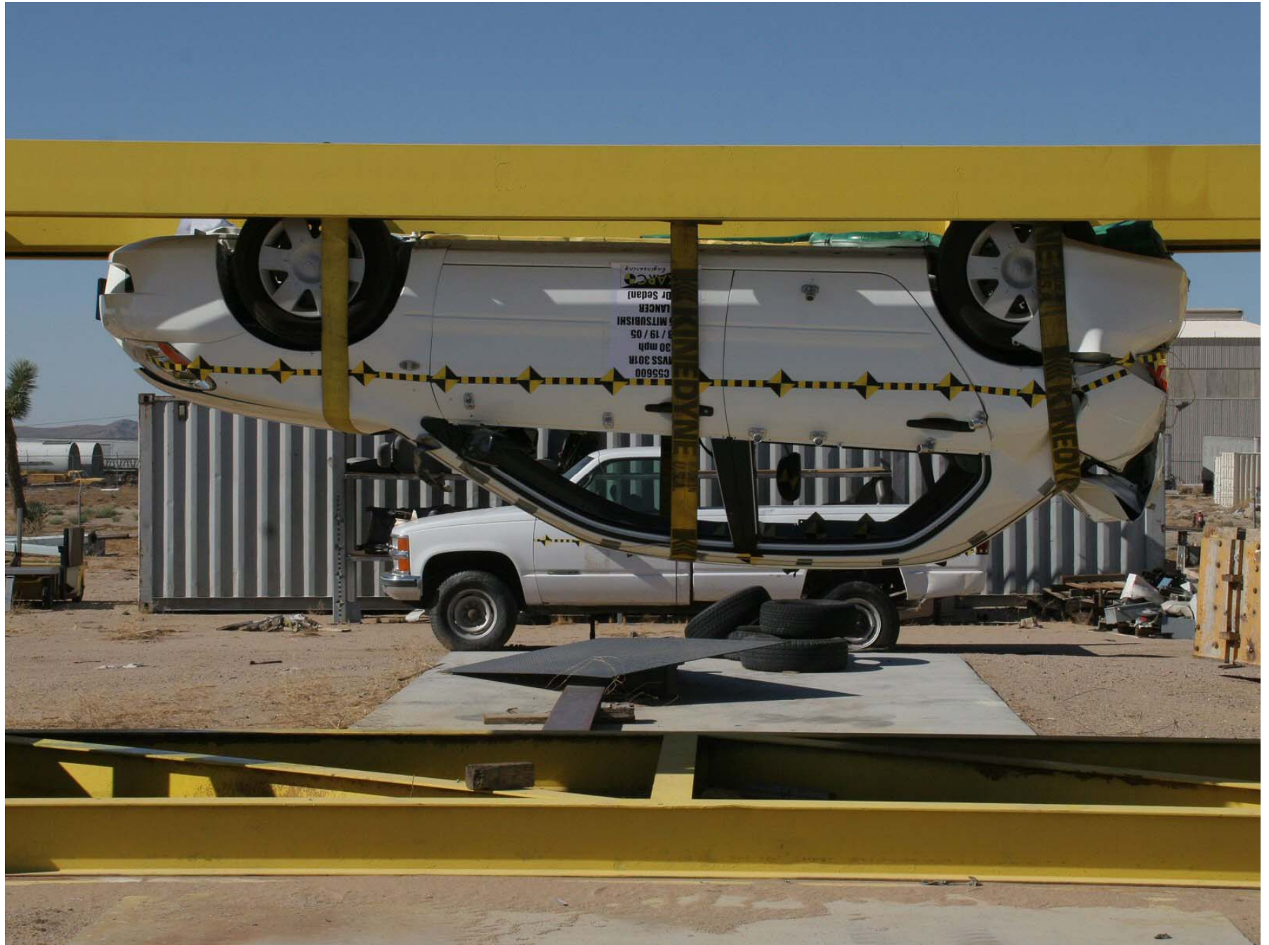
Figure A-23: Vehicle on Rollover Device at 180°
