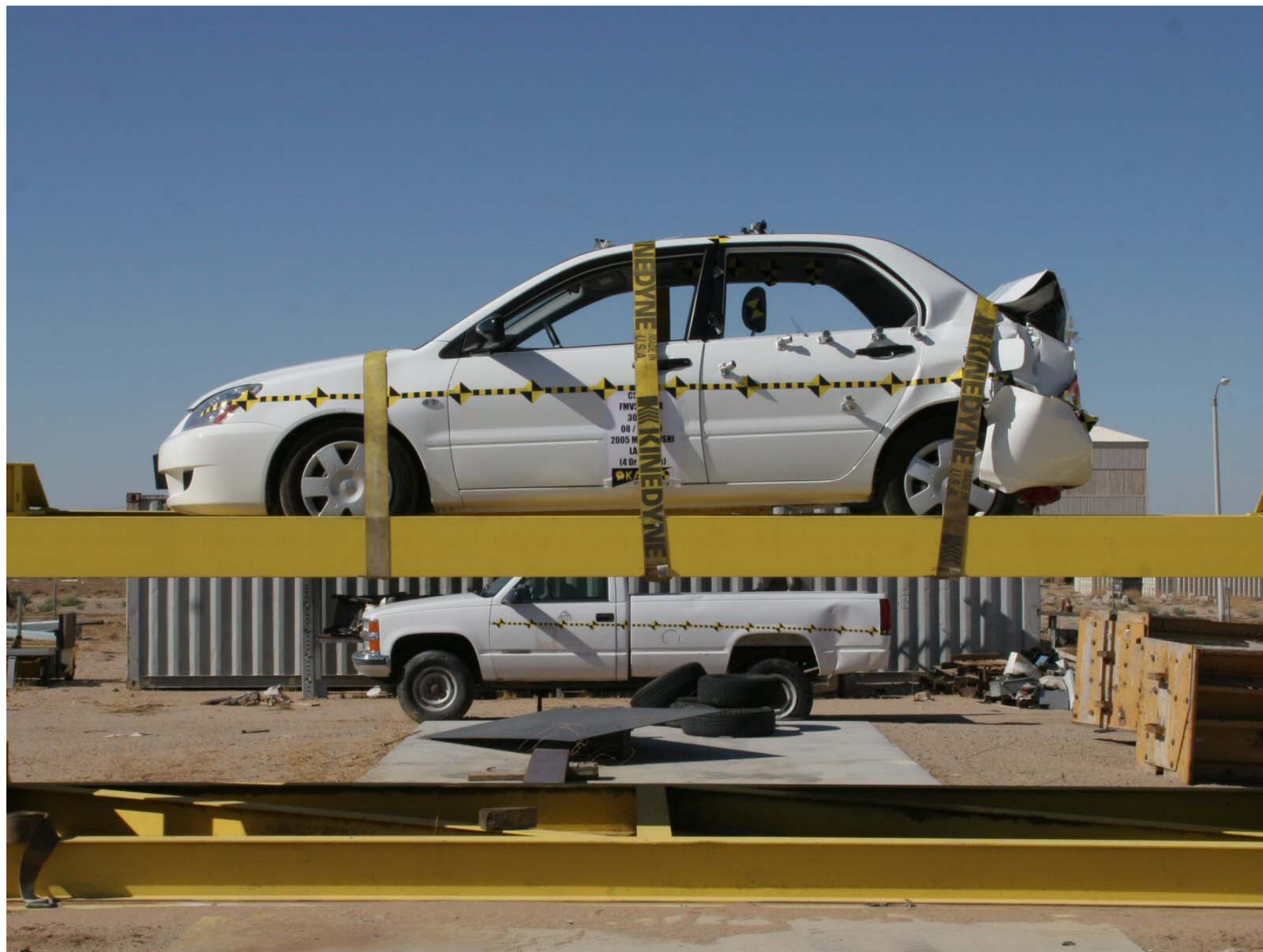
Figure A-21: Vehicle on Rollover Device at 0°
