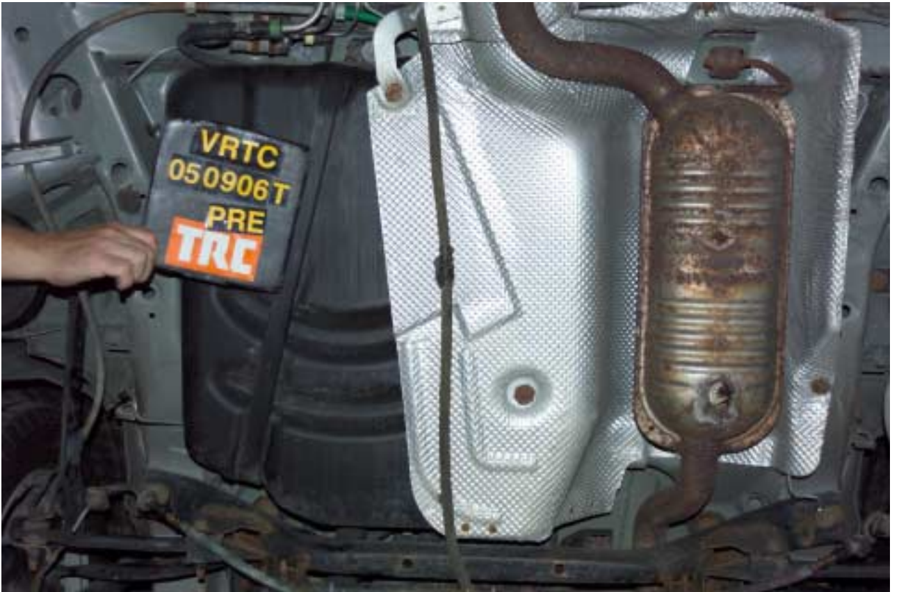
Figure A-39 Pre-Test Target Vehicle Fuel Tank View
