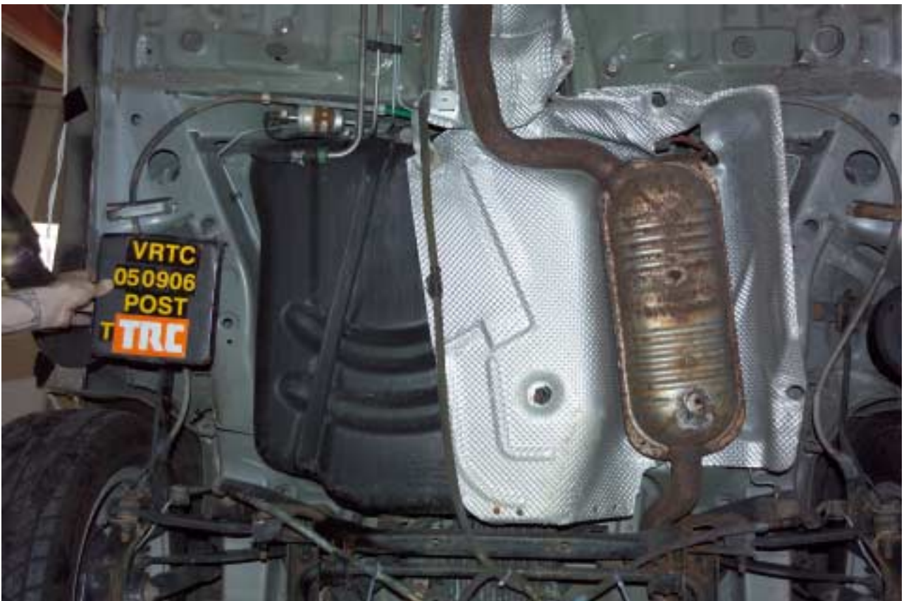
Figure A-40 Post-Test Target Vehicle Fuel Tank View
