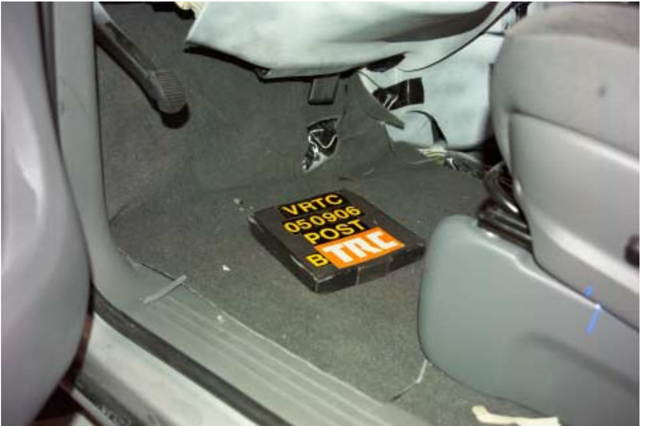
Figure A-140 Post-Test Bullet Vehicle Driver Floorboard Deformation View
