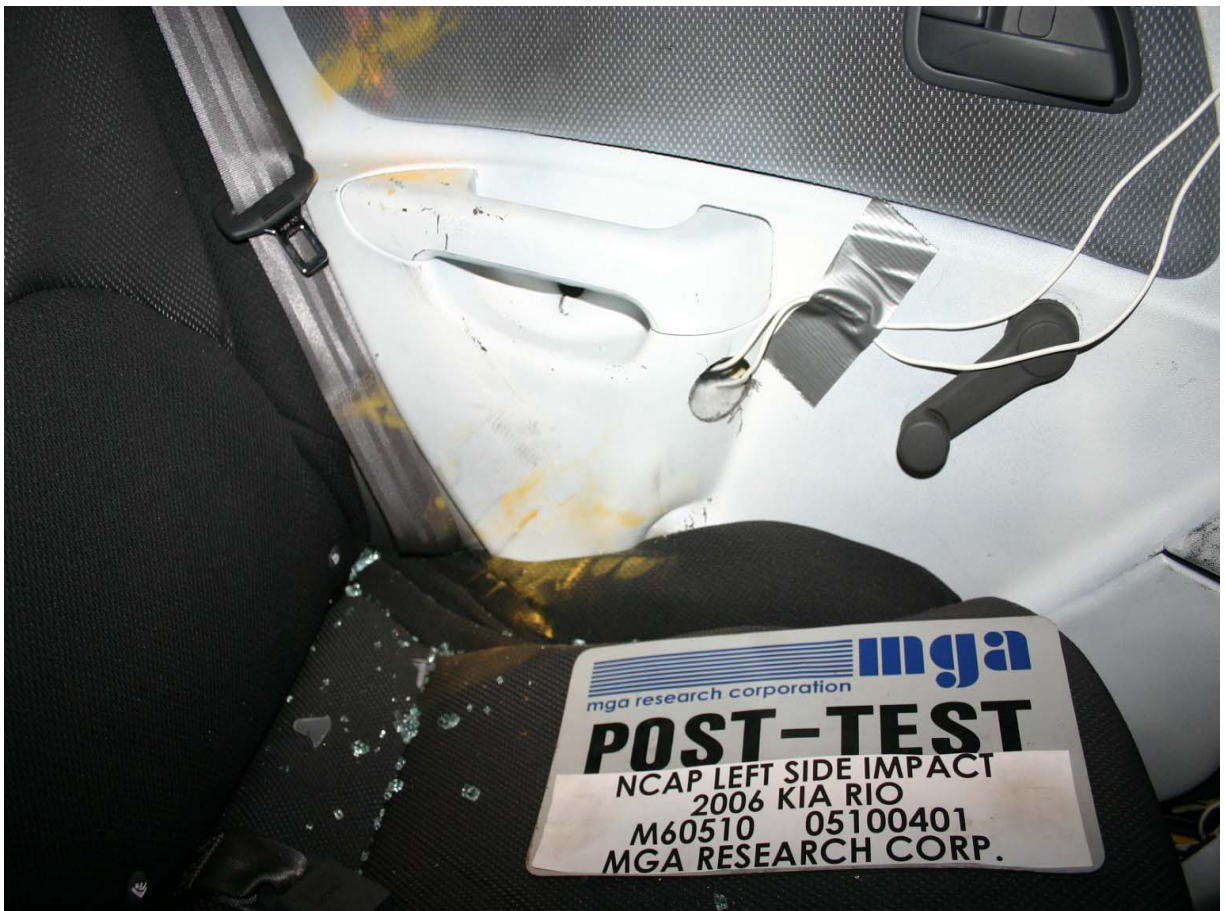
Post-Test Passenger Dummy Lower Torso Contact
