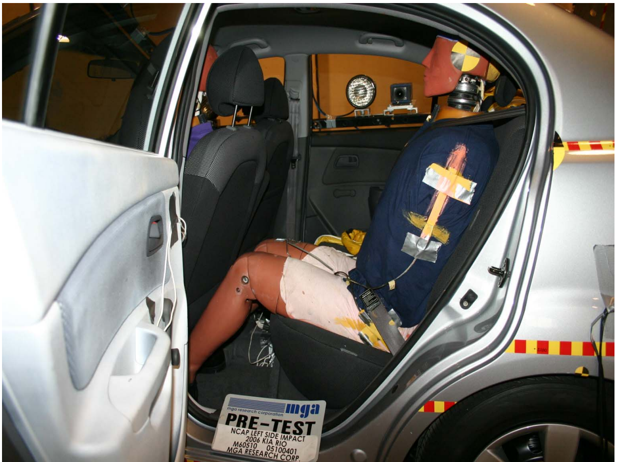
Pre-Test Passenger Dummy (Door Open)
