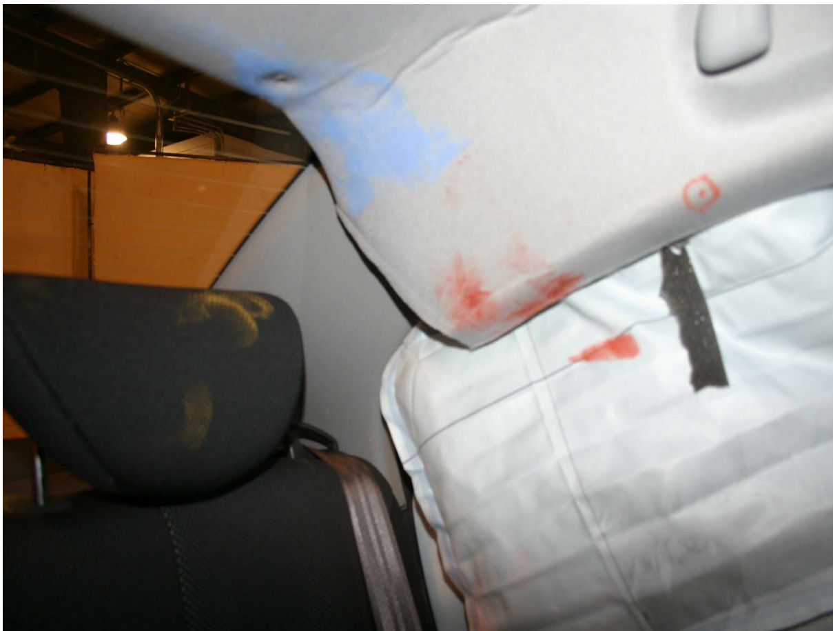
Post-Test Passenger Dummy Head Contact
