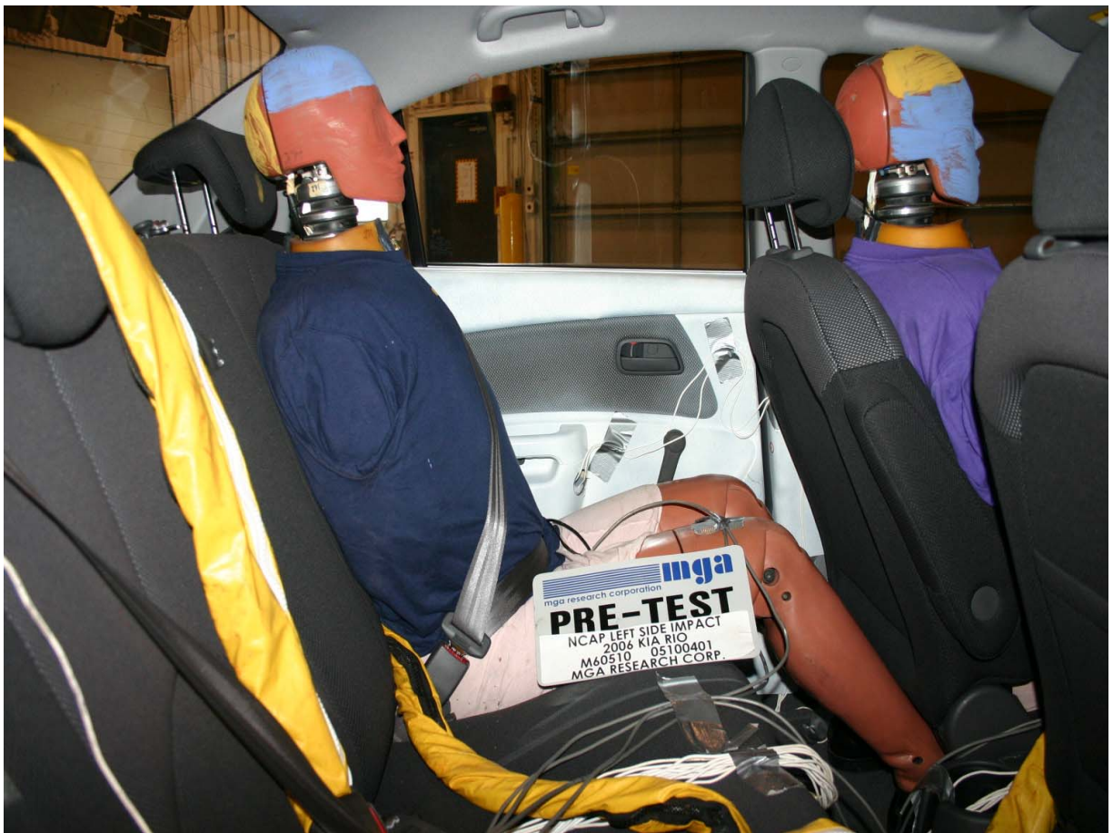
Pre-Test Passenger Dummy Right Side View
