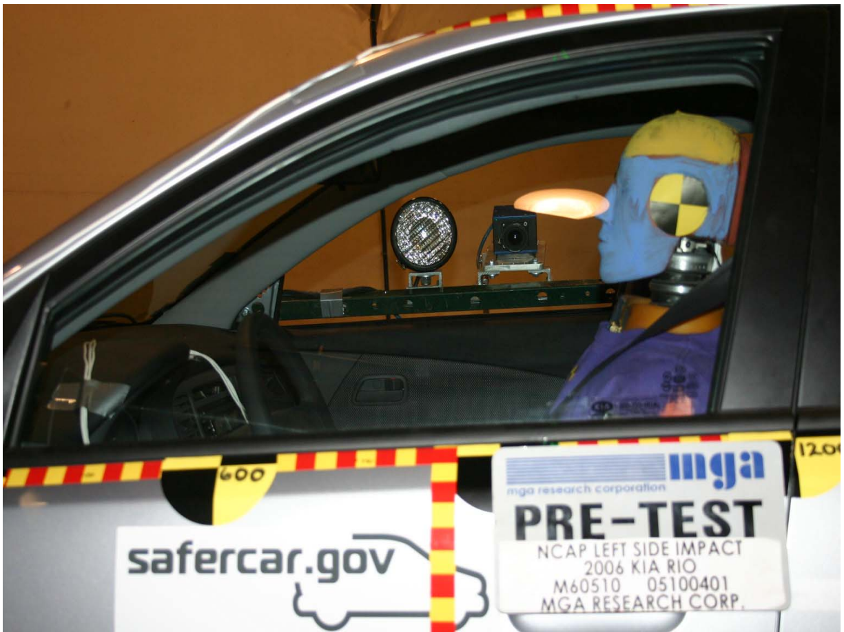
Pre-Test Driver Dummy (Through Window)
