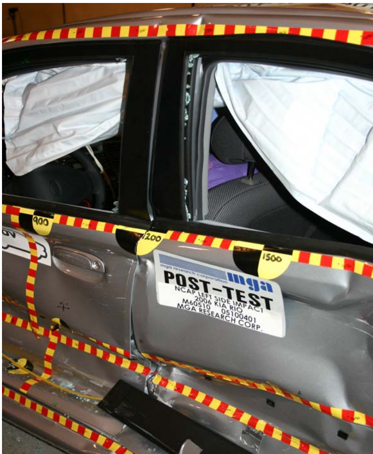
Post-Test Left Front Door
