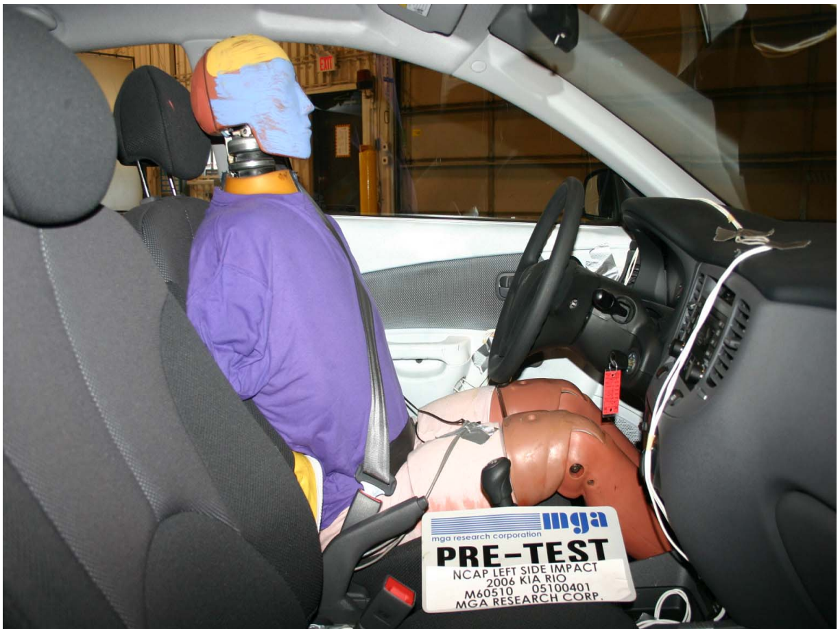
Pre-Test Driver Dummy Right Side View
