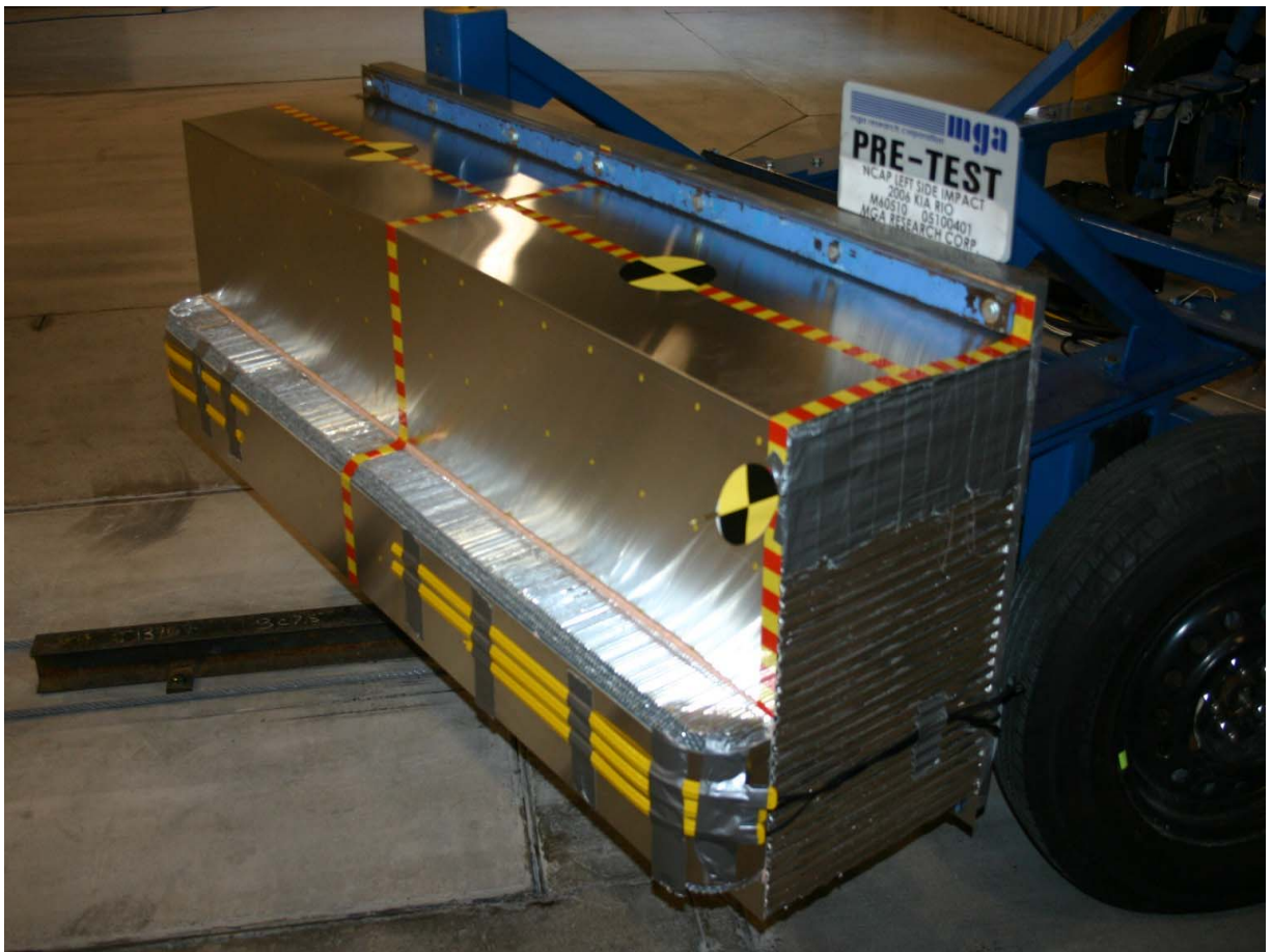
Pre-Test Left Side View of Deformable Barrier
