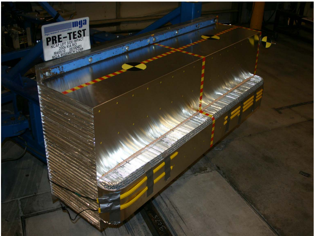
Pre-Test Right Side View of Deformable Barrier
