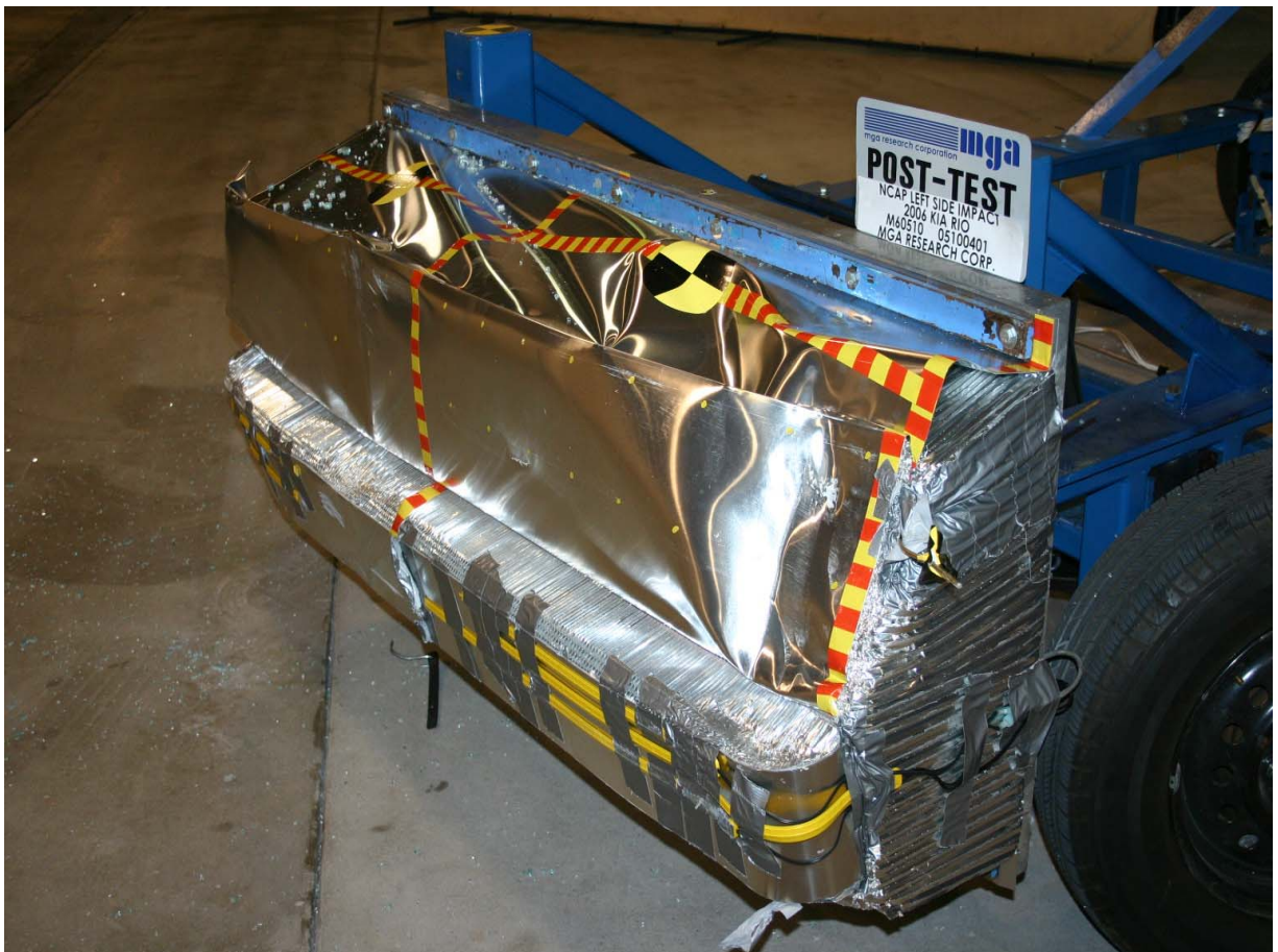
Post-Test Left Side View of Deformable Barrier
