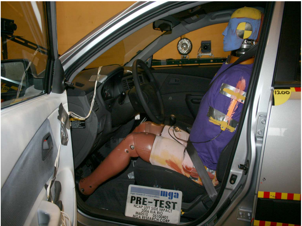
Pre-Test Driver Dummy (Door Open)
