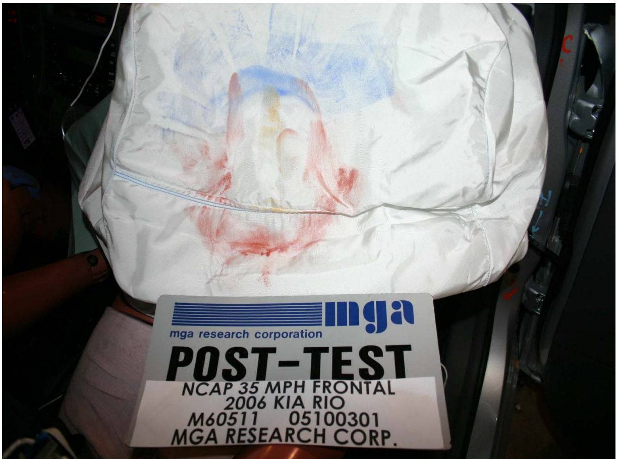
Post-Test Passenger Dummy Airbag Contact
