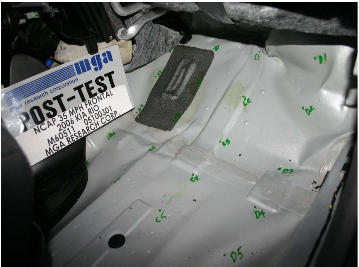
Post-Test Passenger Side Floor Pan
