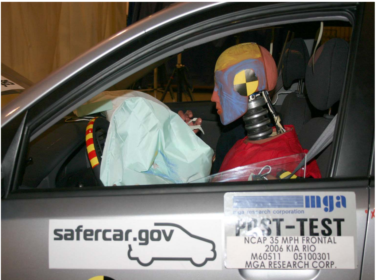
Post-Test Driver Dummy (Through Window)
