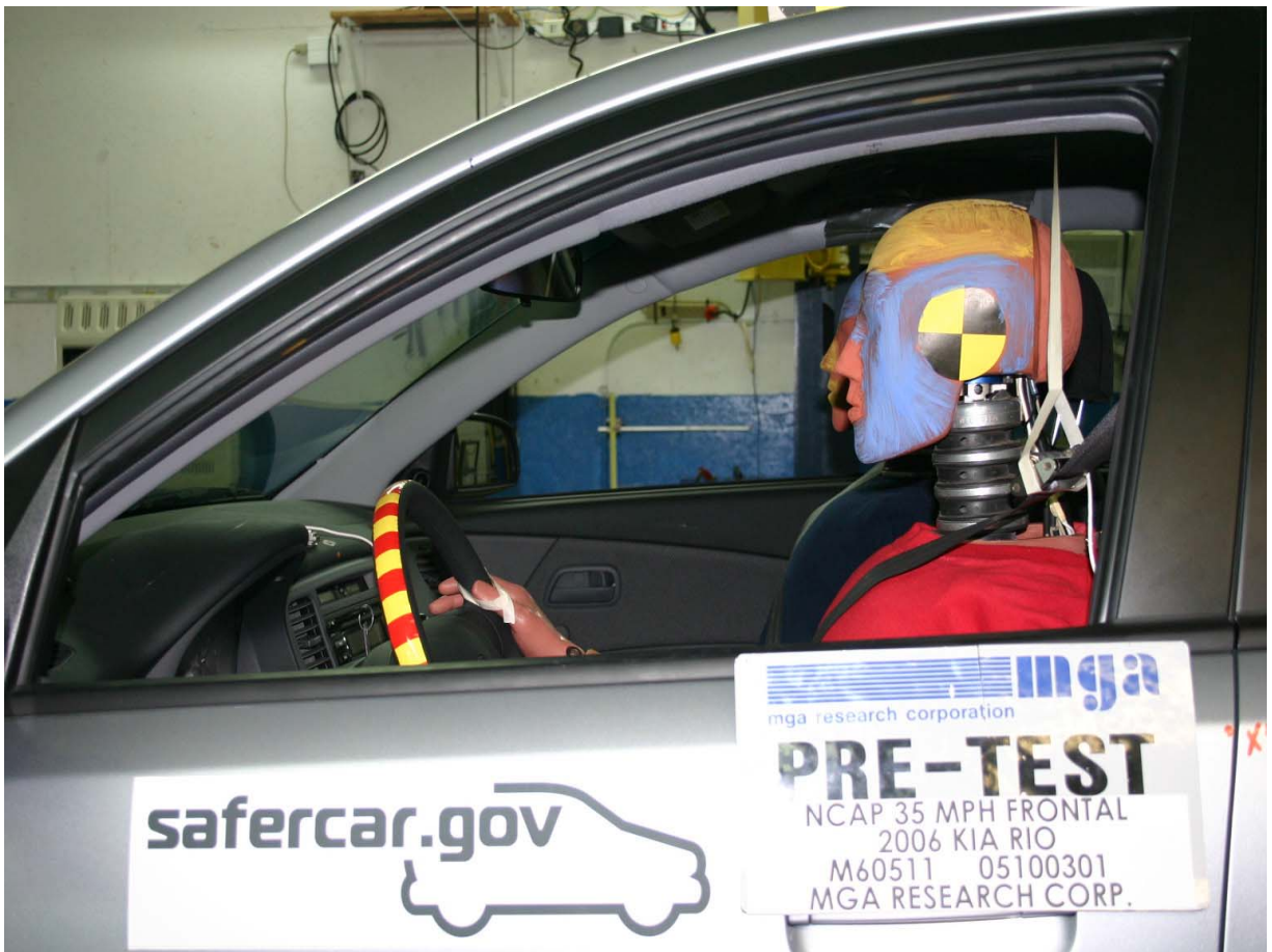
Pre-Test Driver Dummy (Through Window)
