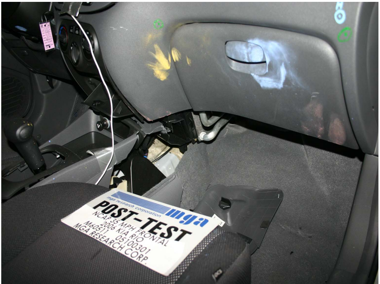
Post-Test Passenger Dummy Knee Contact
