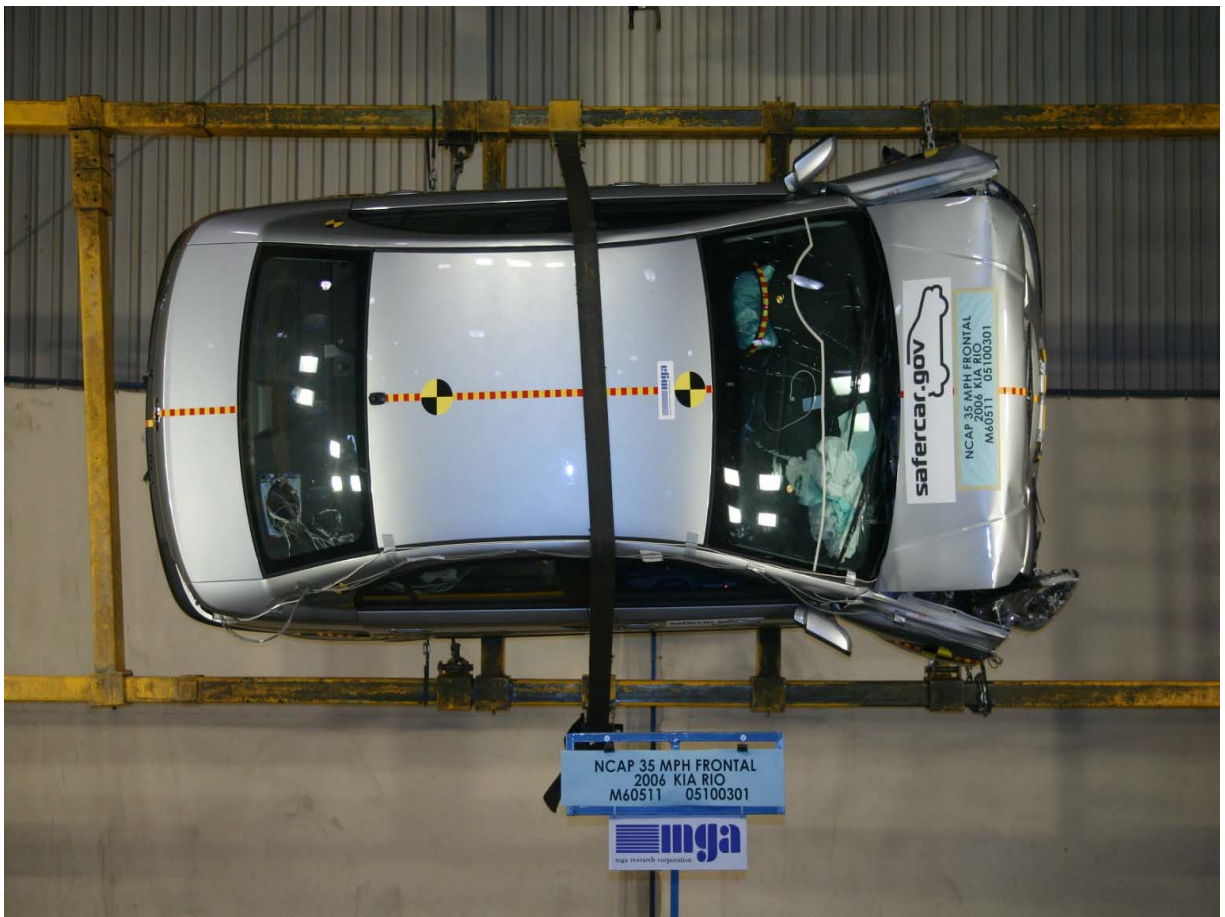
Vehicle on Rollover Device at 270 Degrees
