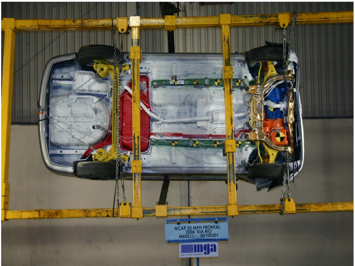
Vehicle on Rollover Device at 90 Degrees
