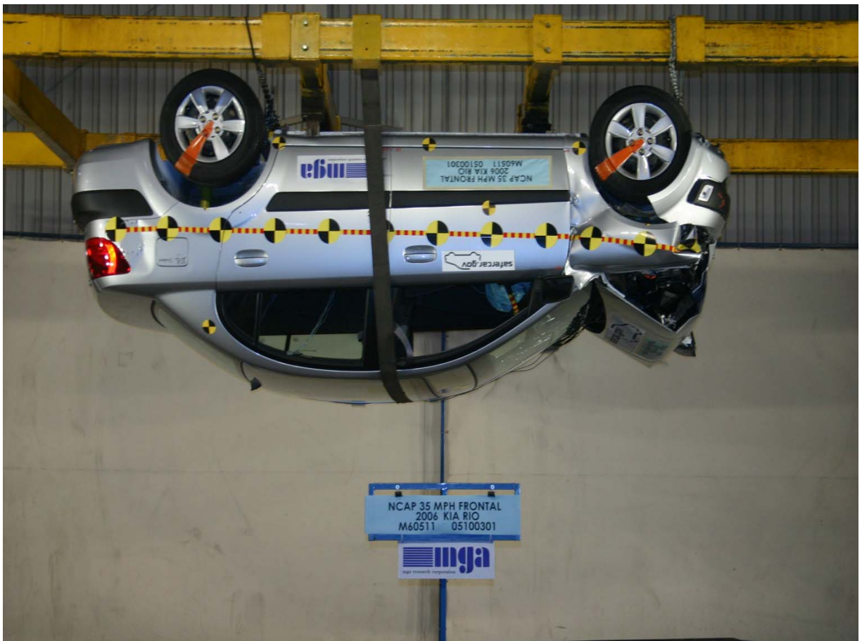
Vehicle on Rollover Device at 180 Degrees
