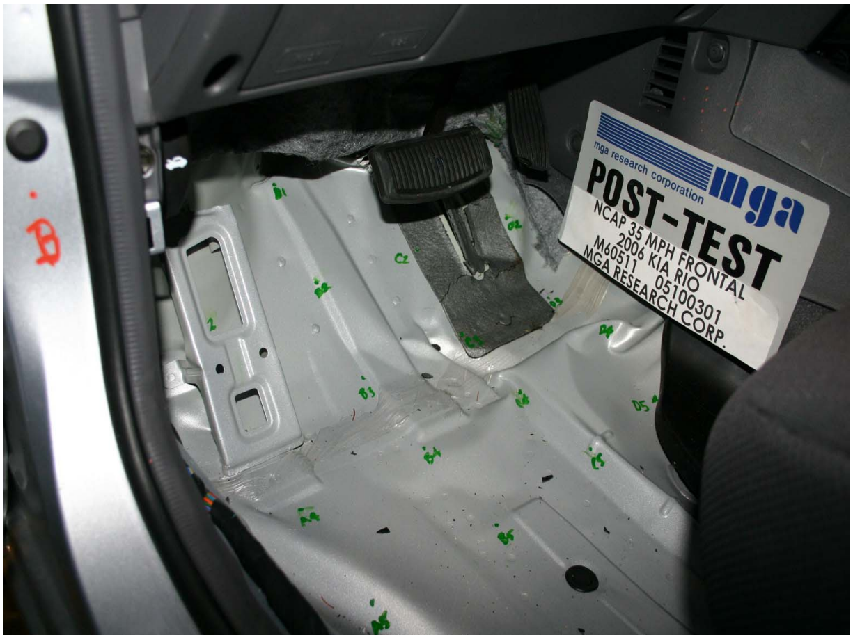
Post-Test Driver Side Floor Pan
