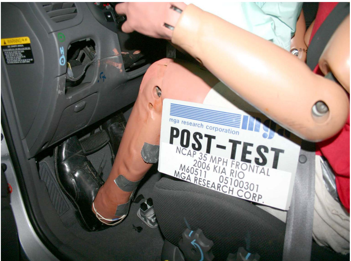
Post-Test Driver Side Knee Bolster
