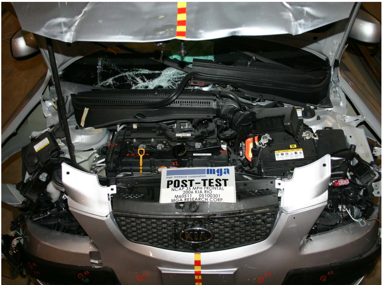
Post-Test Engine Compartment View
