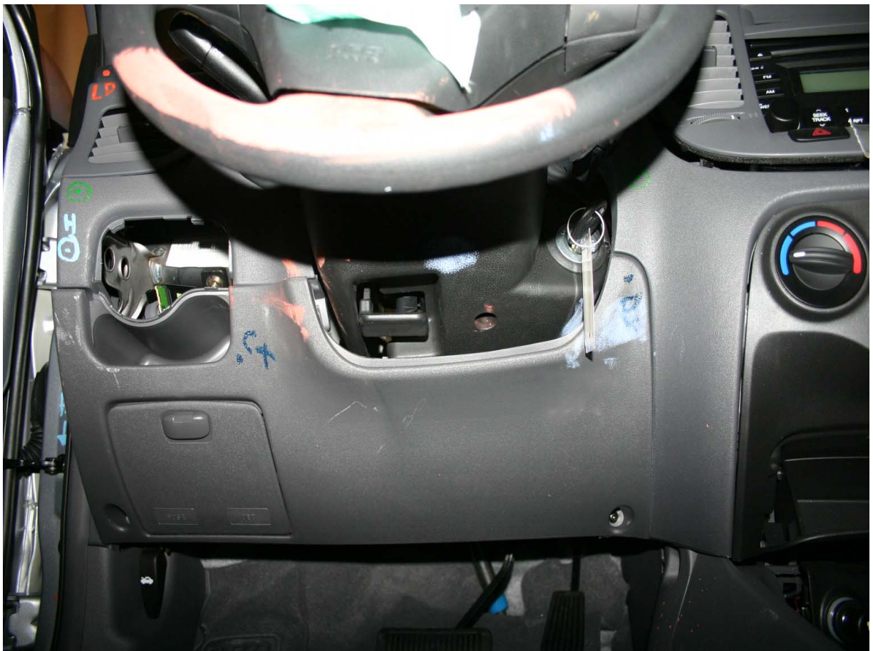
Post-Test Driver Dummy Knee Contact
