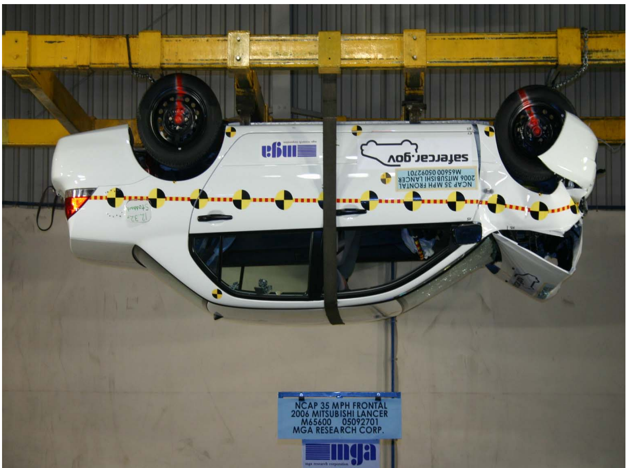
Vehicle on Rollover Device at 180 Degrees
