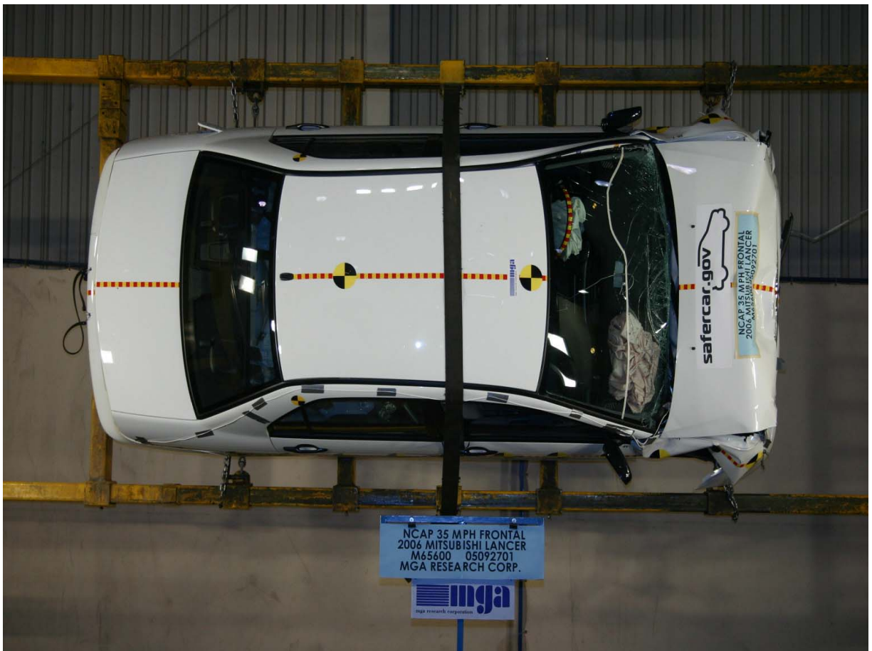
Vehicle on Rollover Device at 270 Degrees
