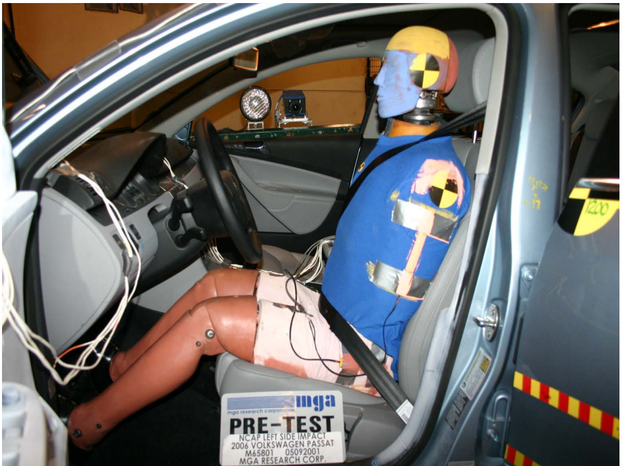
Pre-Test Driver Dummy (Door Open)
