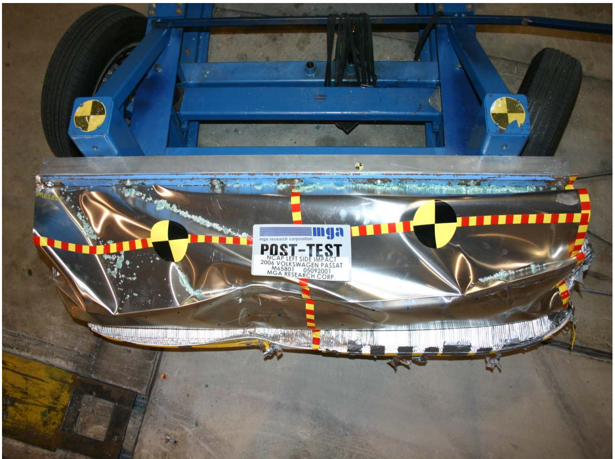
Post-Test Top View of Deformable Barrier
