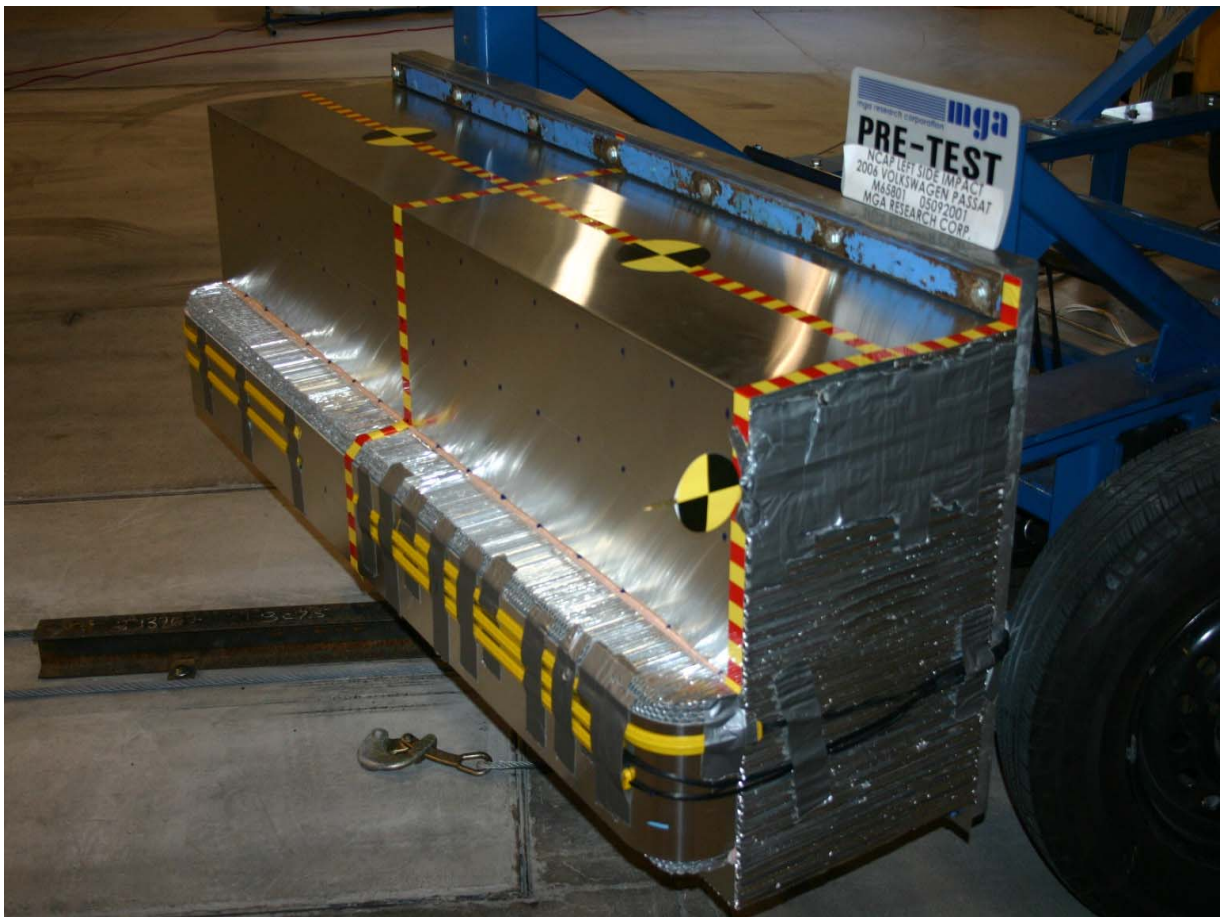
Pre-Test Left Side View of Deformable Barrier
