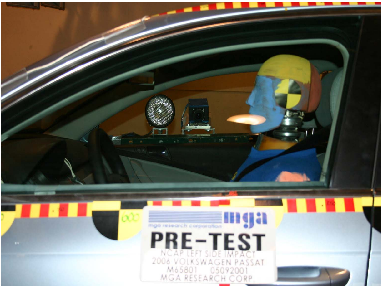
Pre-Test Driver Dummy (Through Window)
