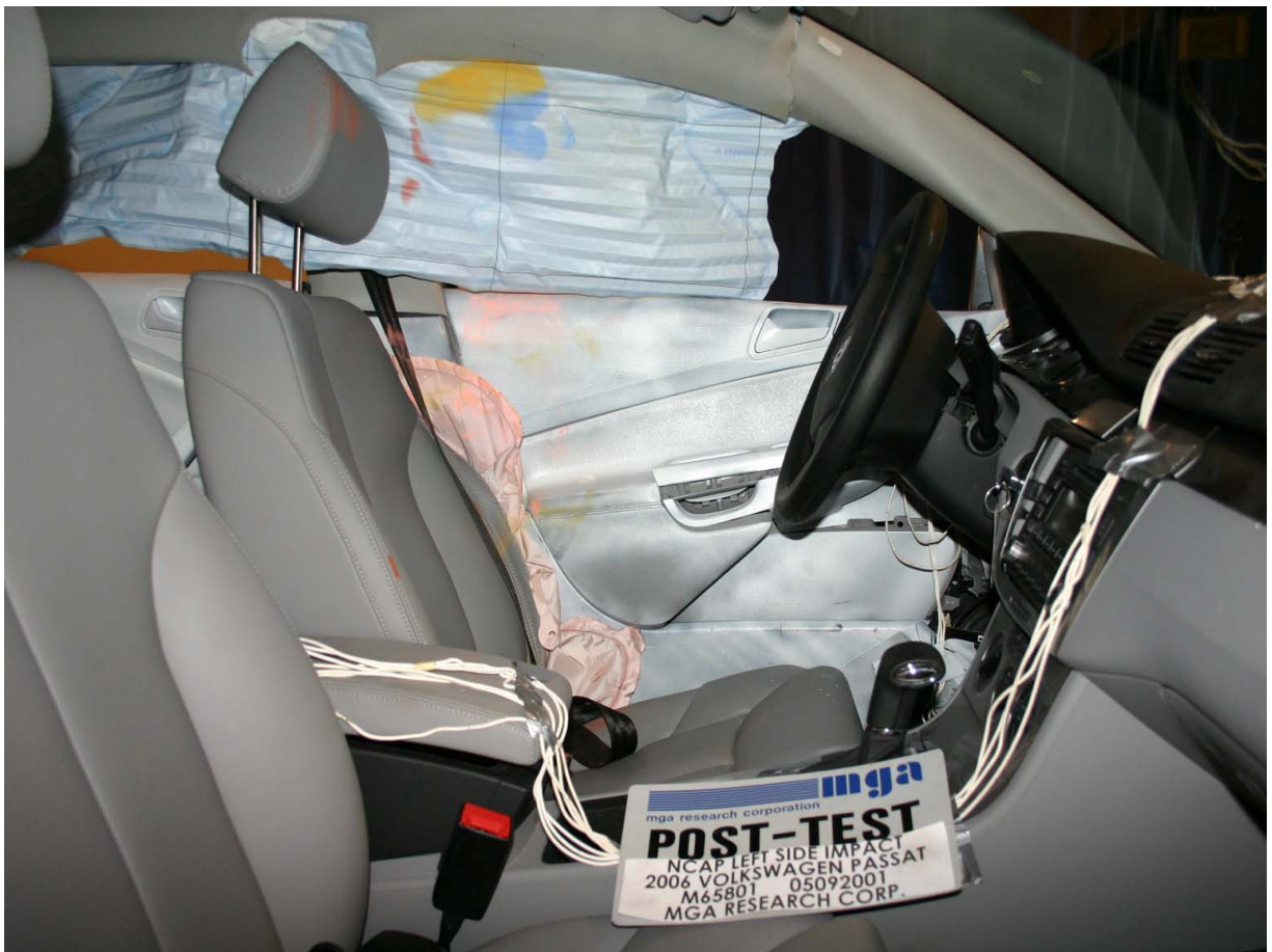
Post-Test Front Door Panel (Interior)
