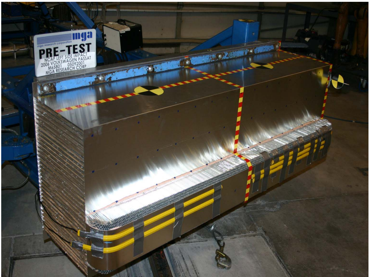
Pre-Test Right Side View of Deformable Barrier
