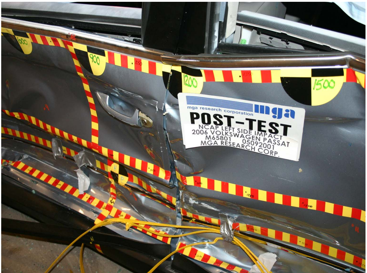
Post-Test Left Front Door
