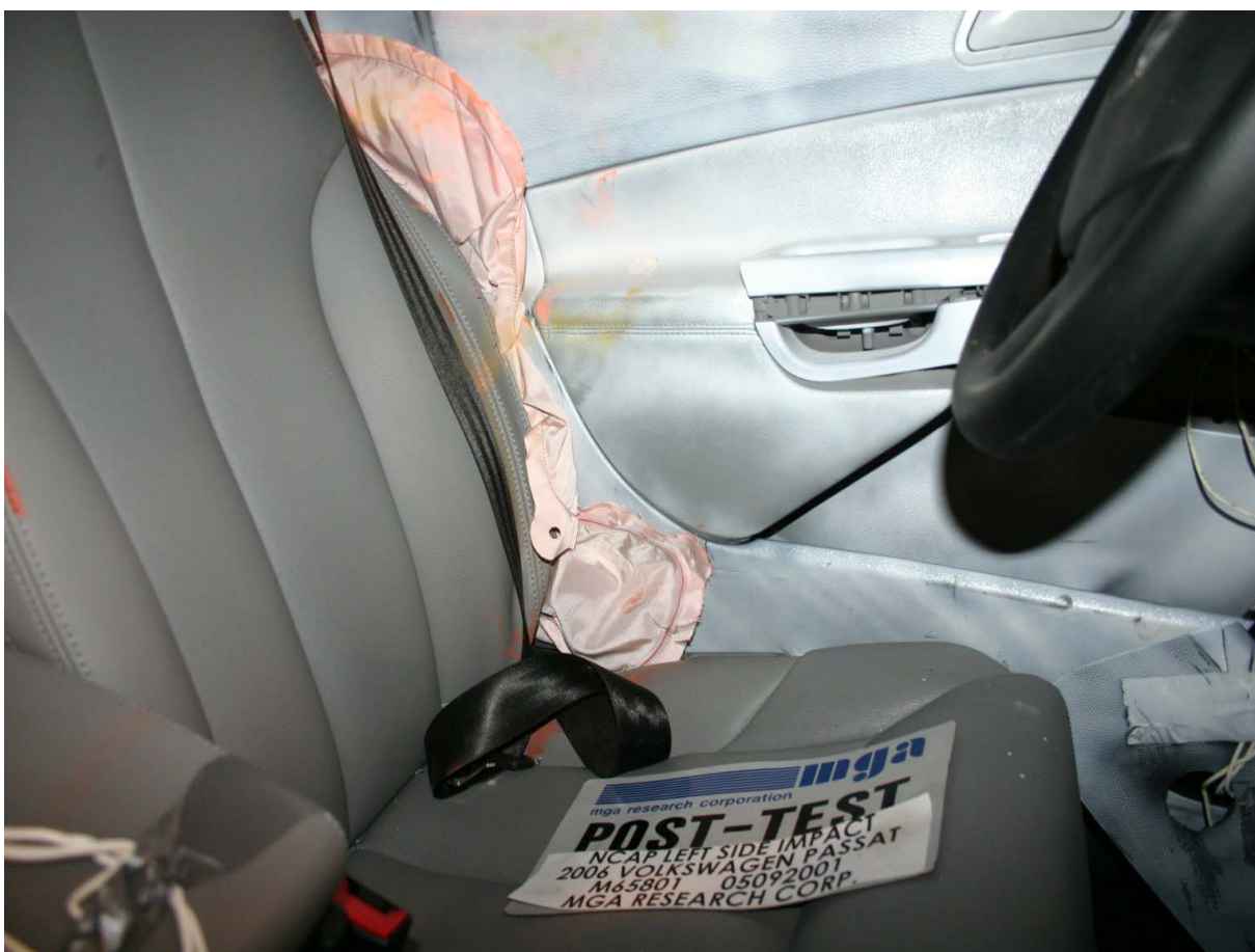
Post-Test Driver Dummy Lower Torso Contact
