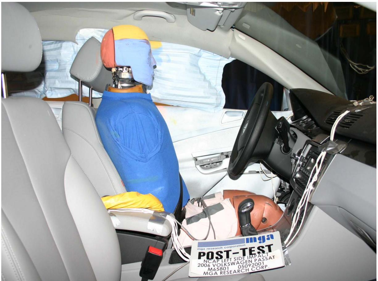
Post-Test Driver Dummy Right Side View
