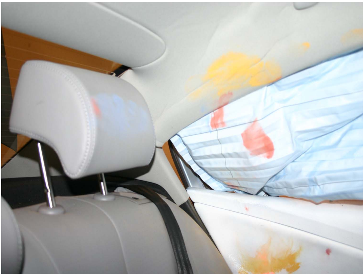
Post-Test Passenger Dummy Head Contact
