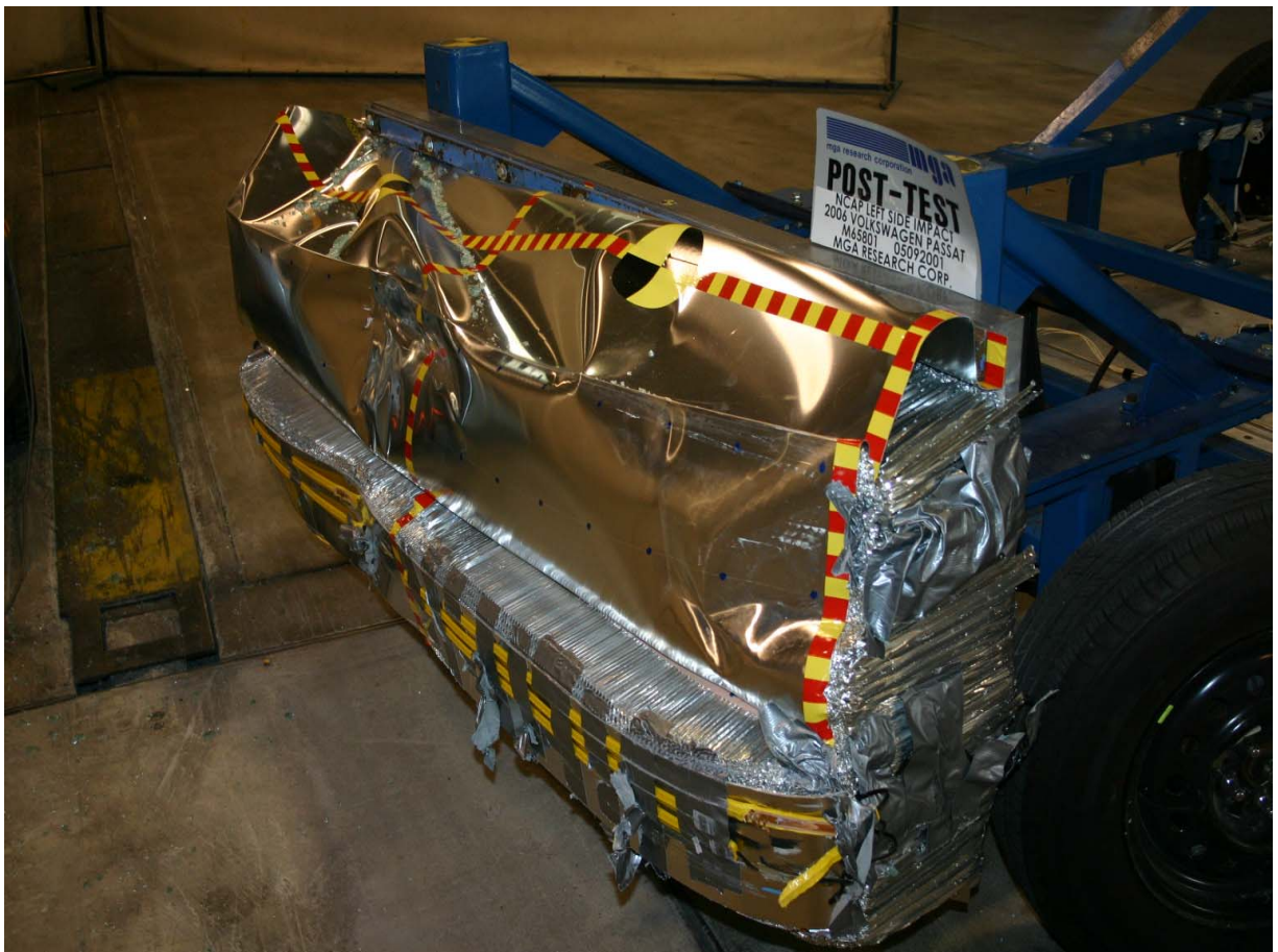
Post-Test Left Side View of Deformable Barrier
