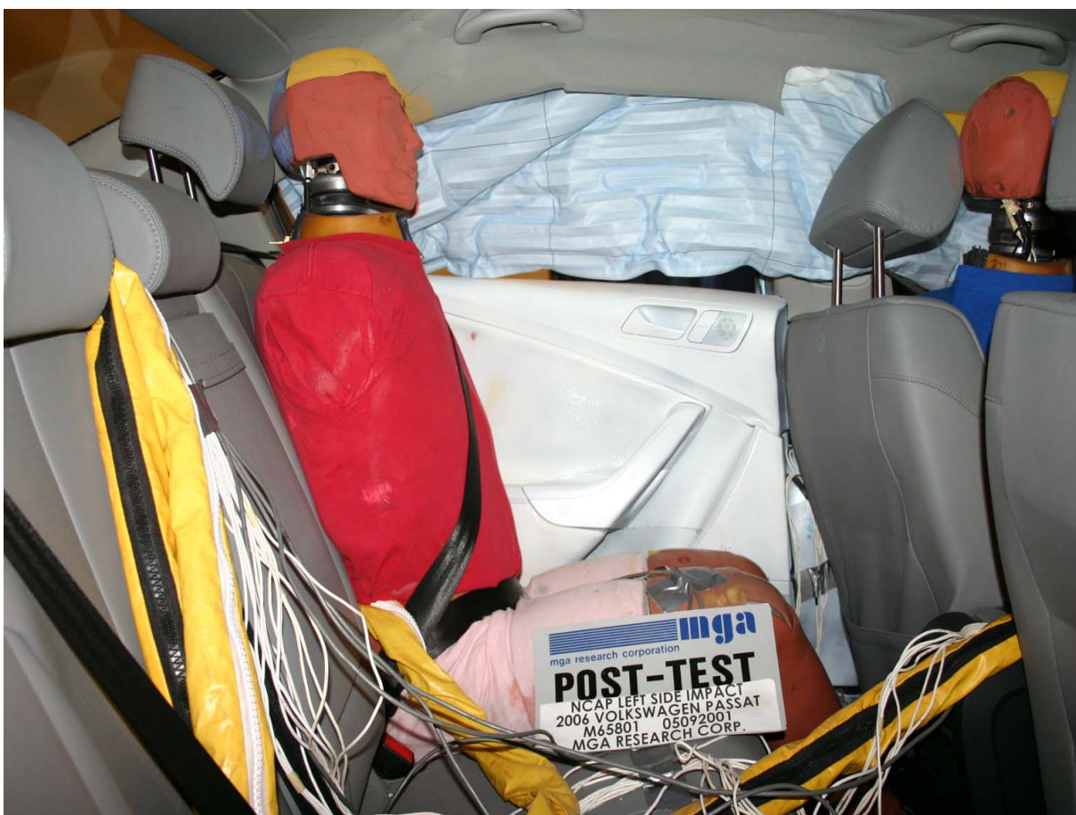
Post-Test Passenger Dummy Right Side View
