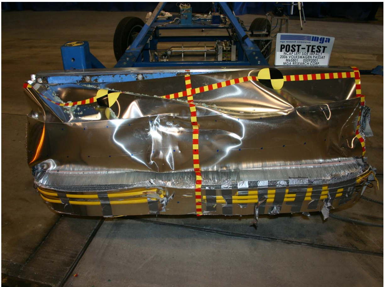
Post-Test Front View of Deformable Barrier
