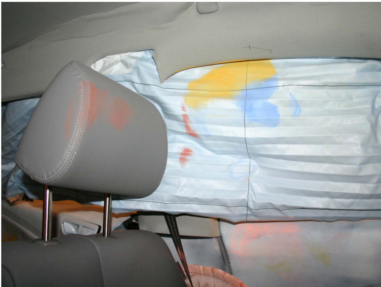
Post-Test Driver Dummy Head Contact
