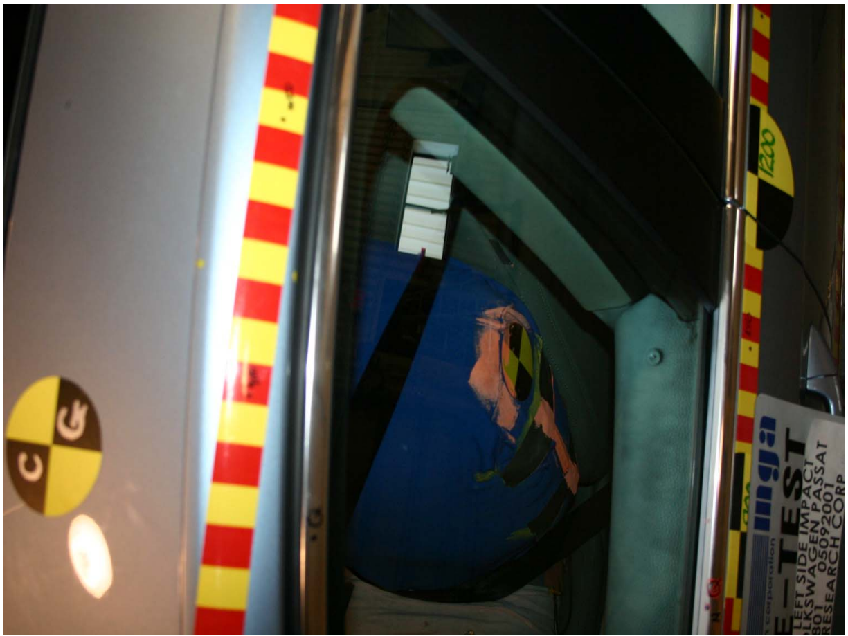
Pre-Test Driver Dummy Clearance From Door
