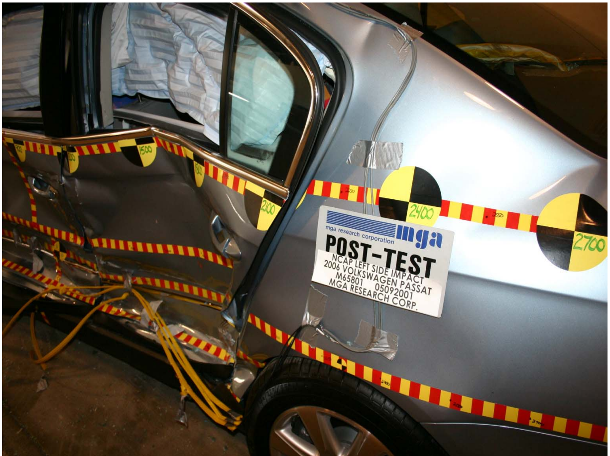
Post-Test Left Rear Door
