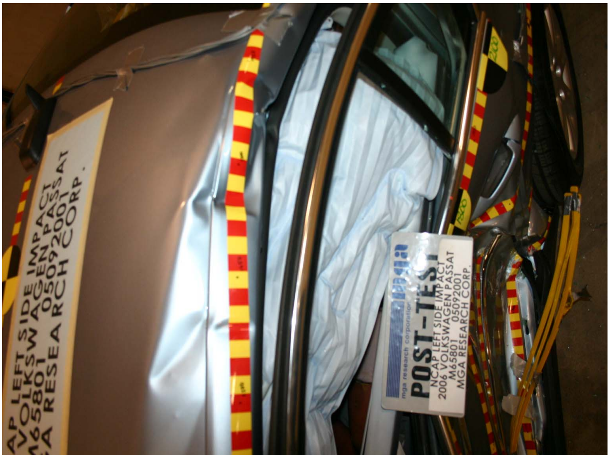
Post-Test Passenger Dummy Clearance From Door
