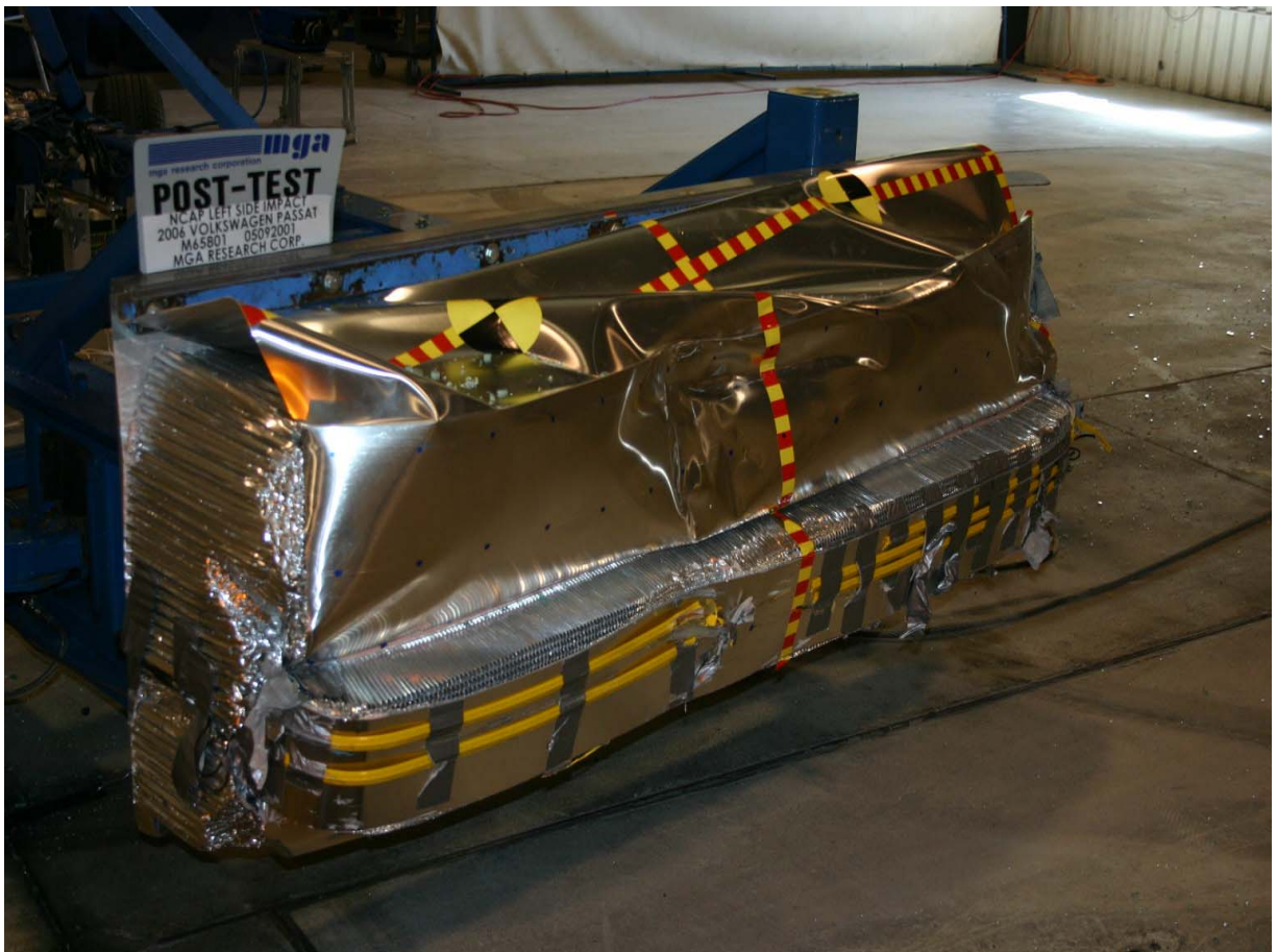
Post-Test Right Side View of Deformable Barrier
