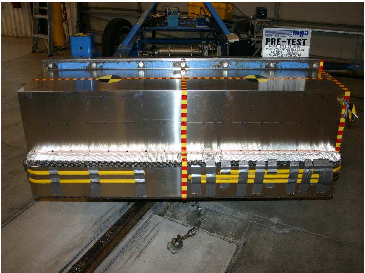
Pre-Test Front View of Deformable Barrier
