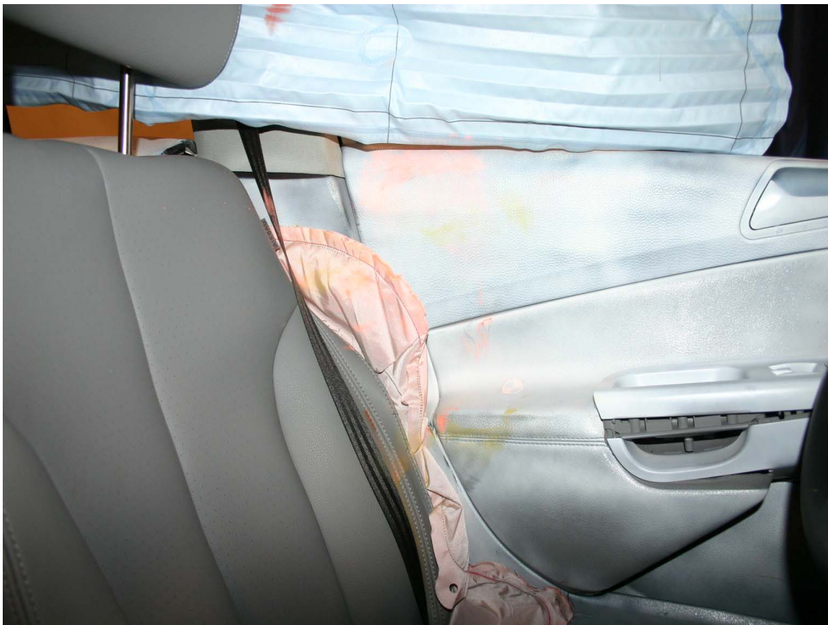
Post-Test Driver Dummy Upper Torso Contact
