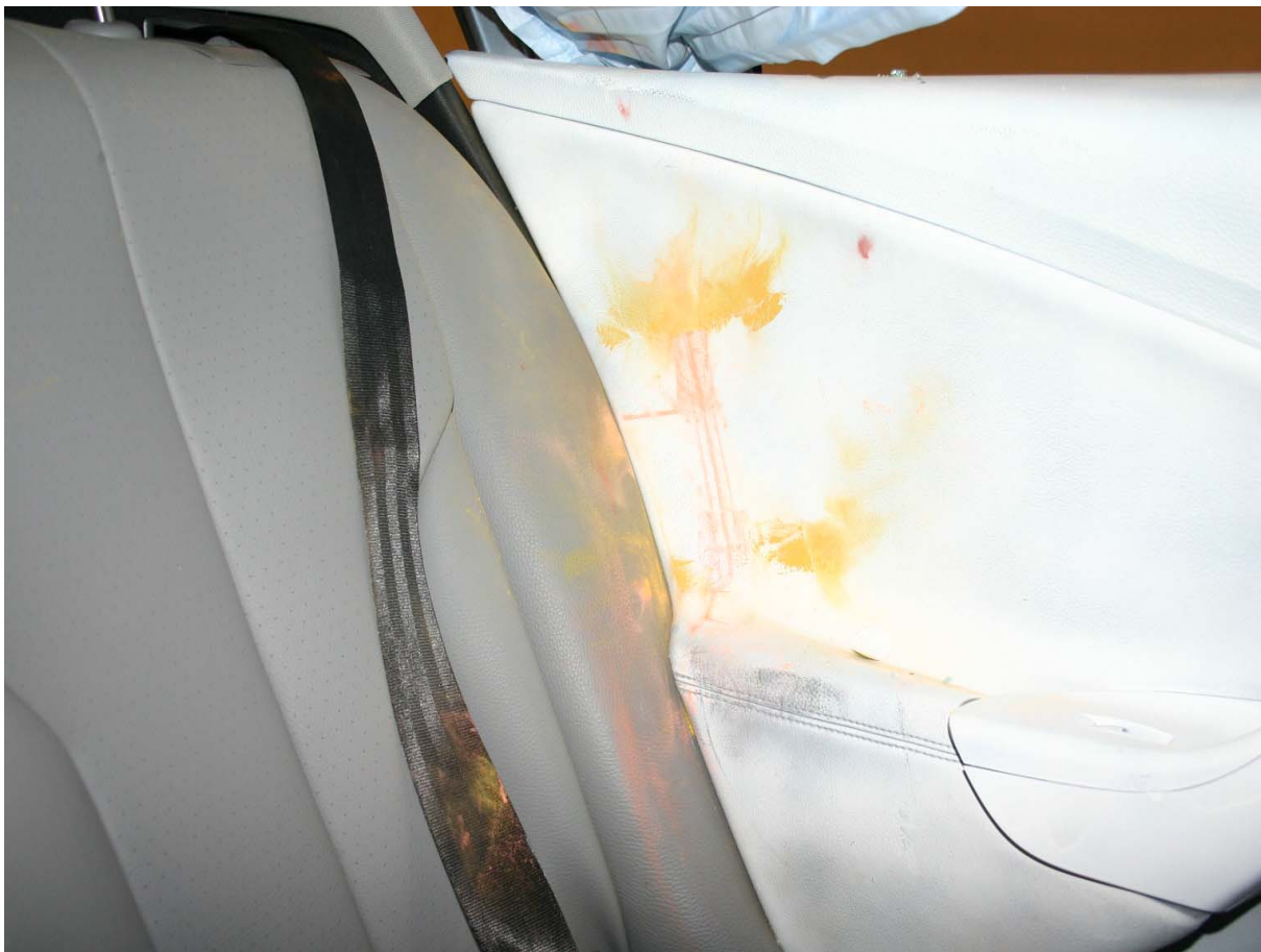
Post-Test Passenger Dummy Upper Torso Contact
