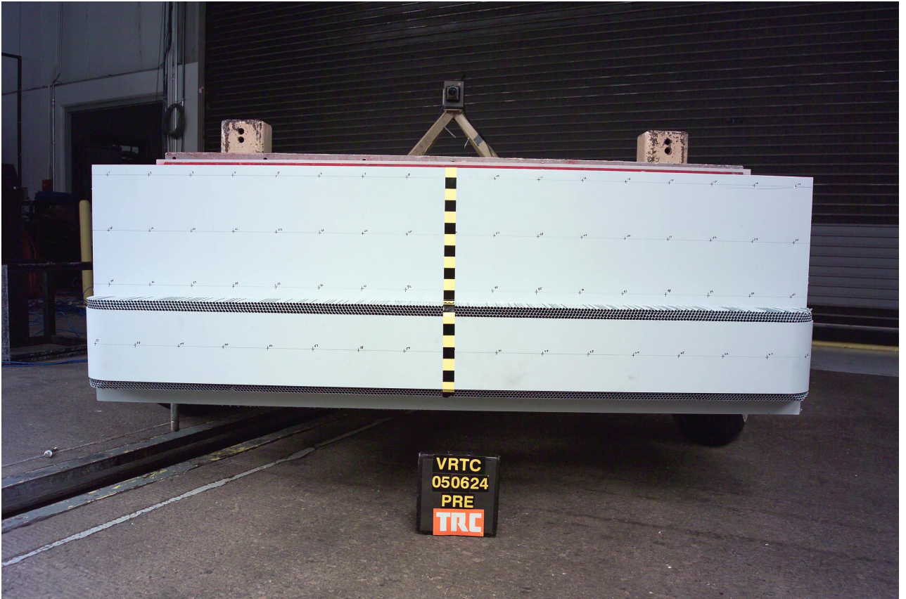
Figure A-77 Pre-Test Barrier Face Front View
