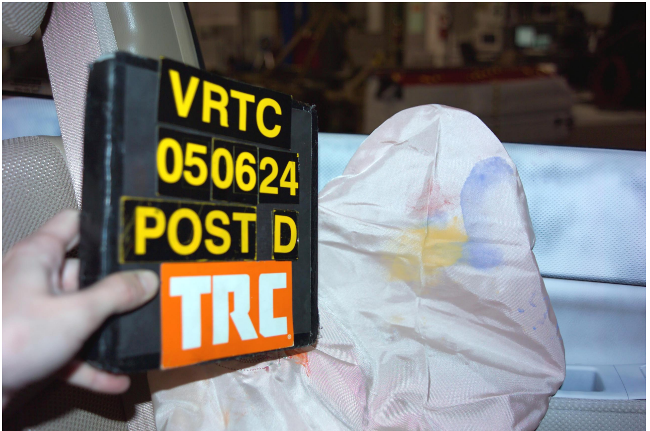
Figure A-60 Post-Test Front ES-2re Contact - View 1
