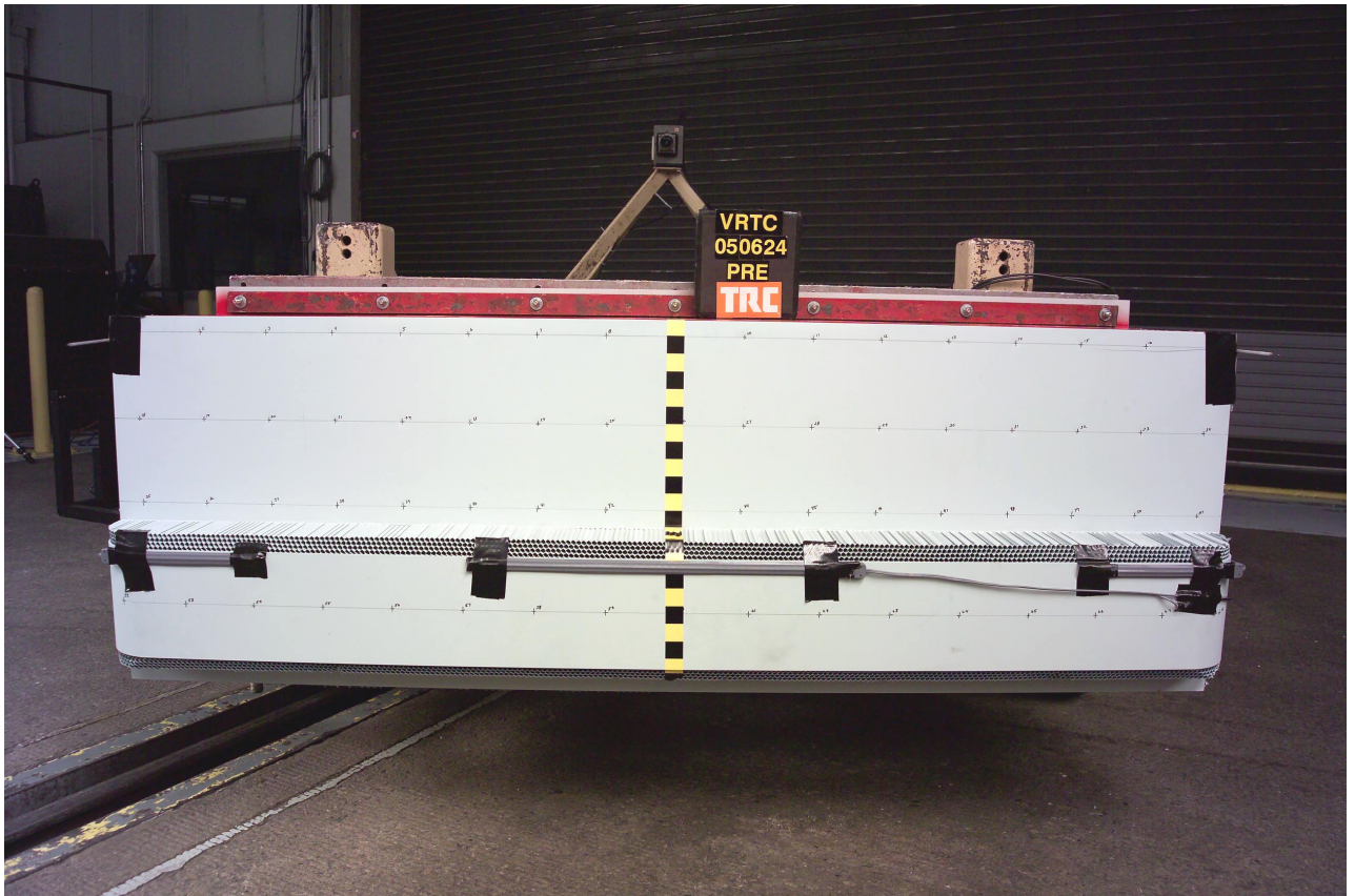
Figure A-36 Pre-Test View of MDB Showing Contact Switches in Place
