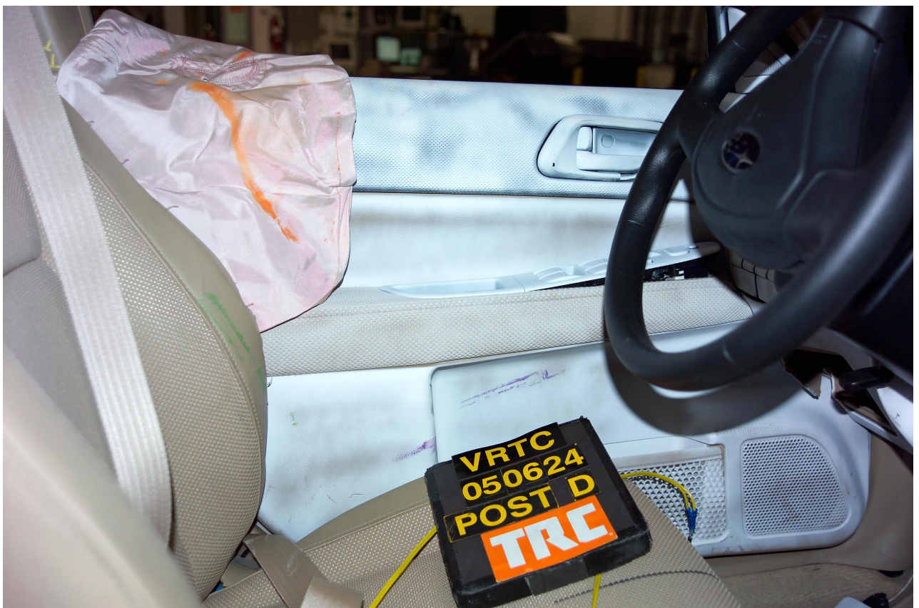
Figure A-59 Post-Test Interior of Front Door Showing ES-2re Impact Locations
