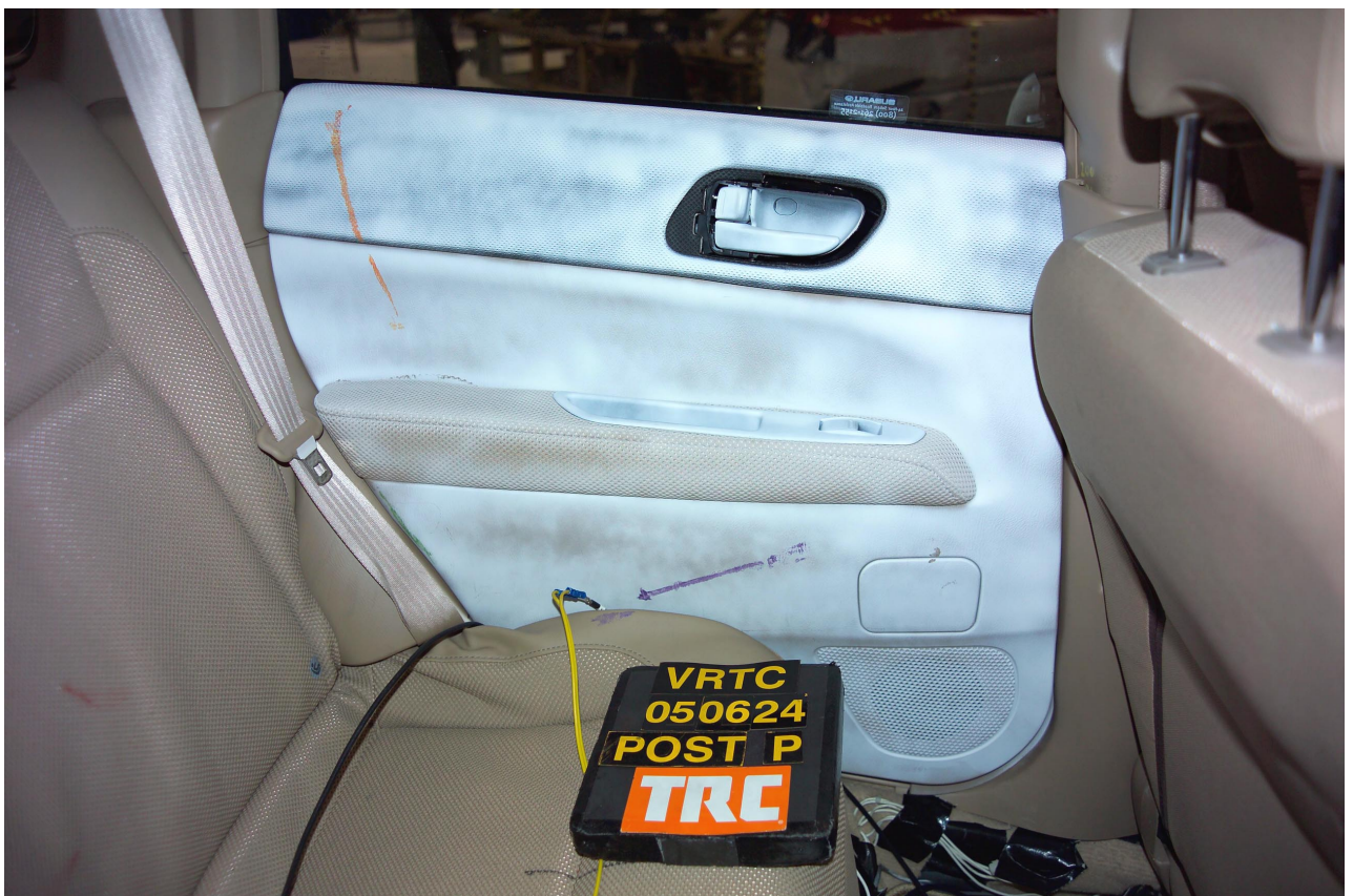
Figure A-66 Post-Test Interior of Rear Door Showing ES-2re Impact Locations
