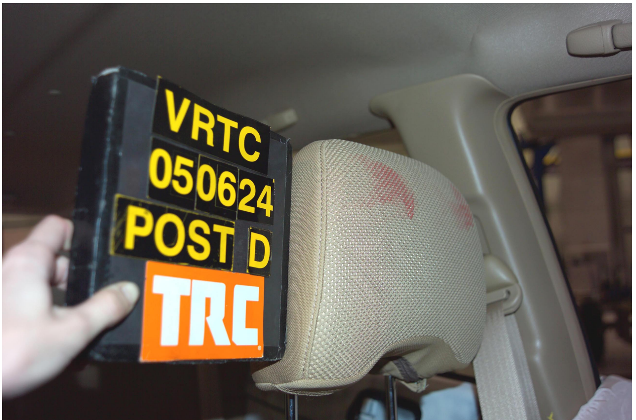
Figure A-61 Post-Test Front ES-2re Contact - View 2
