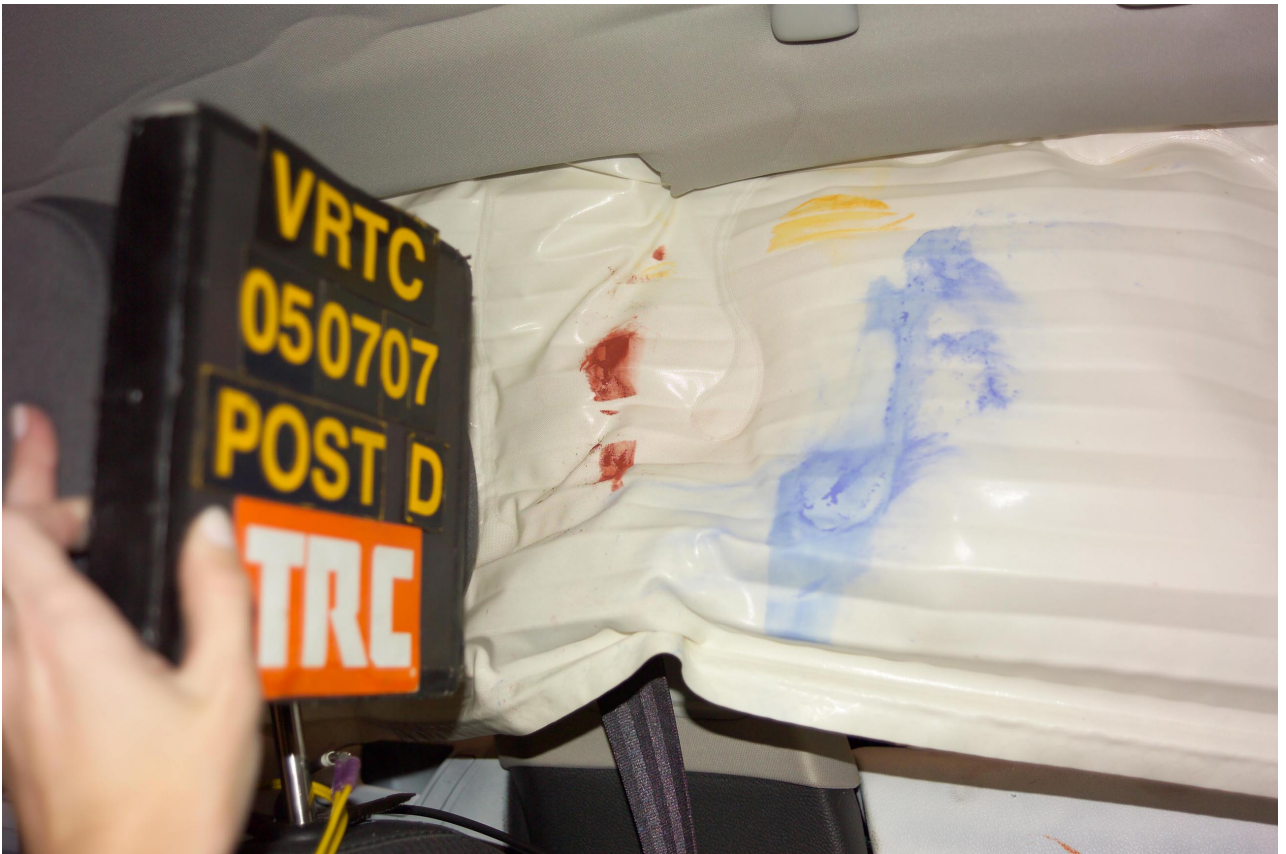
Figure A-60 Post-Test Front ES-2re Contact - View 1
