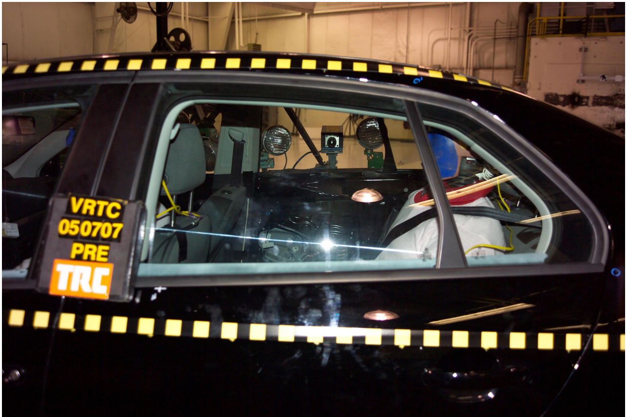
Figure A-53 Pre-Test Left View of Rear ES-2re - View 1
