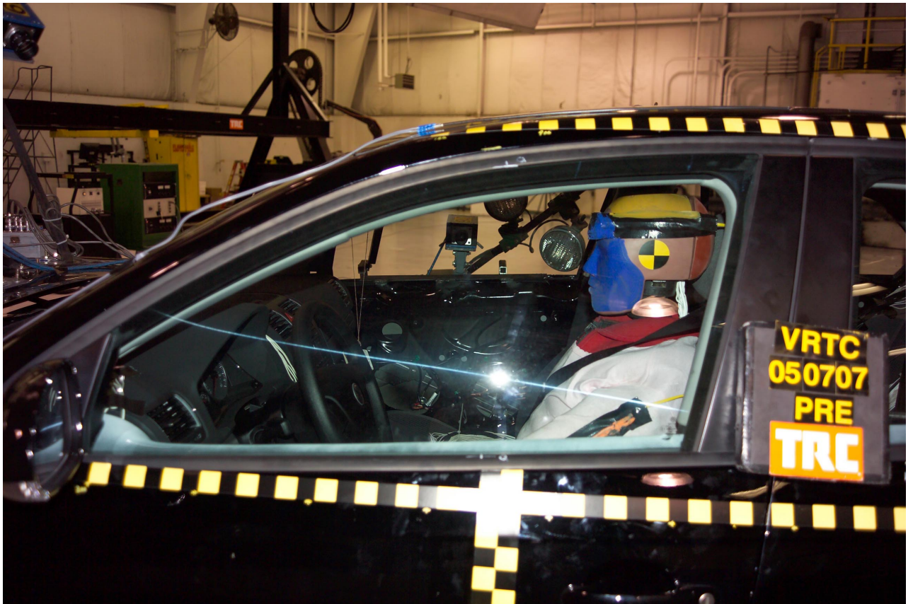
Figure A-48 Pre-Test Left View of Front ES-2re - View 1
