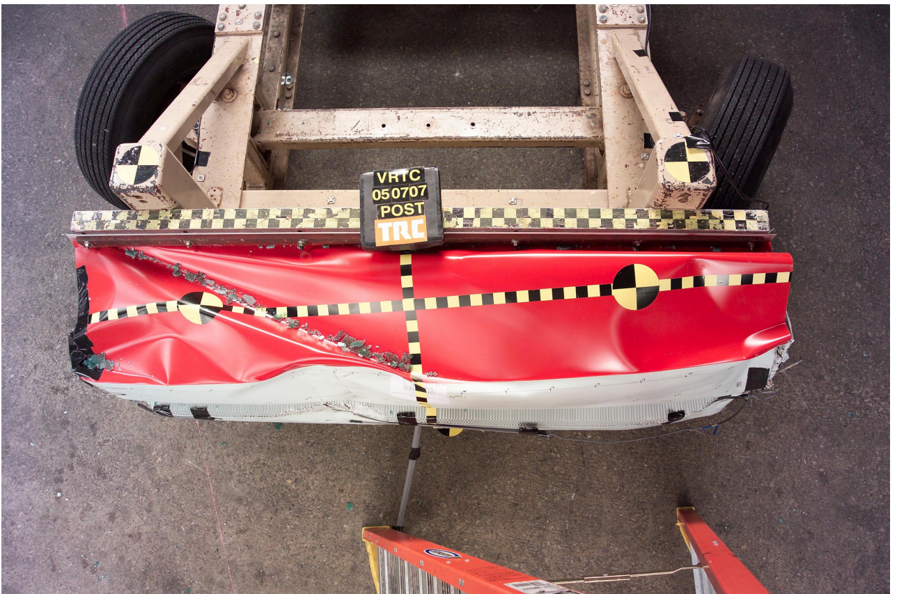
Figure A-79 Post-Test Barrier Face Overhead View
