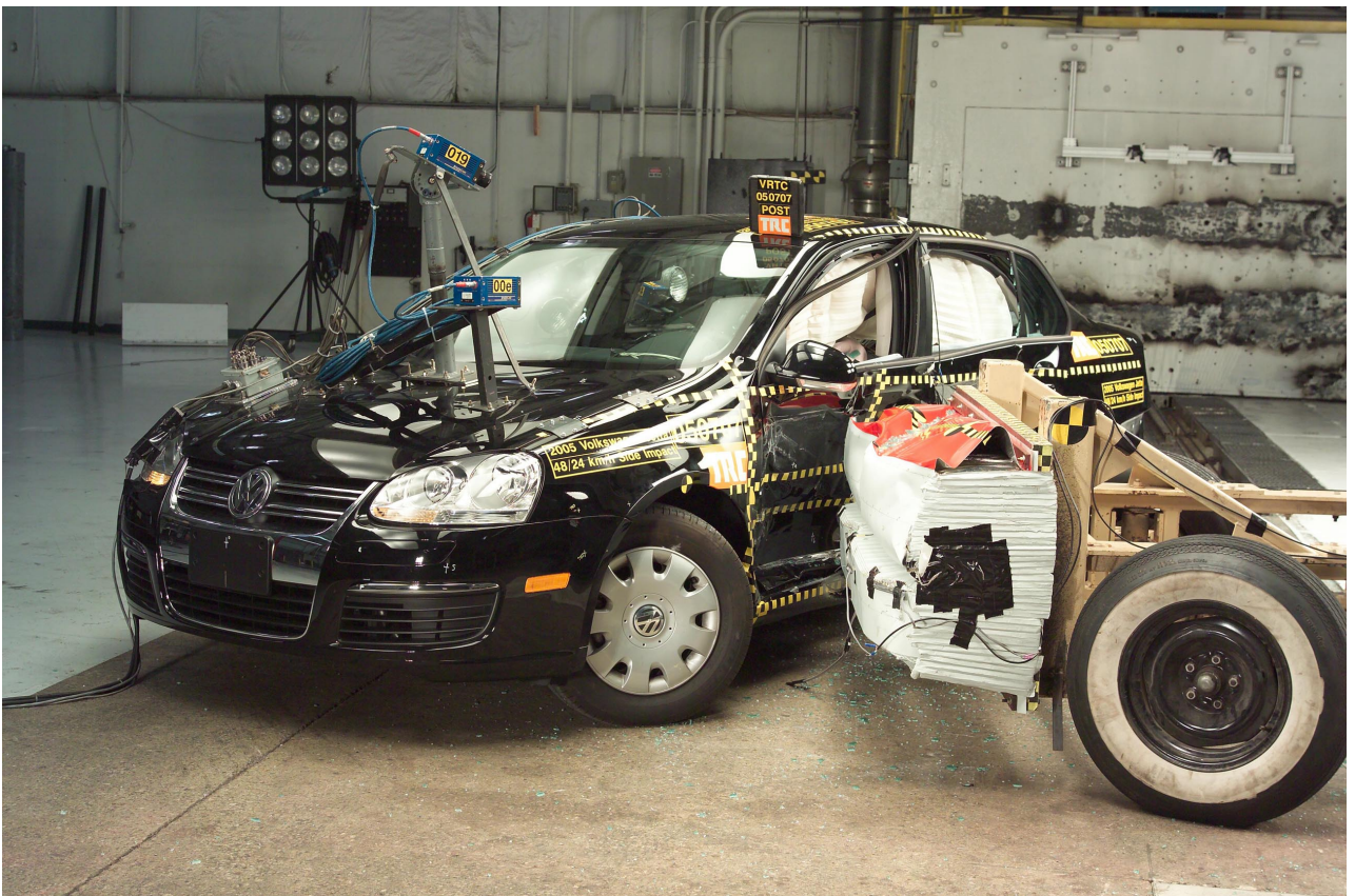
Figure A-22 Post-Test Left Front View of MDB with Impactor Face in Position
