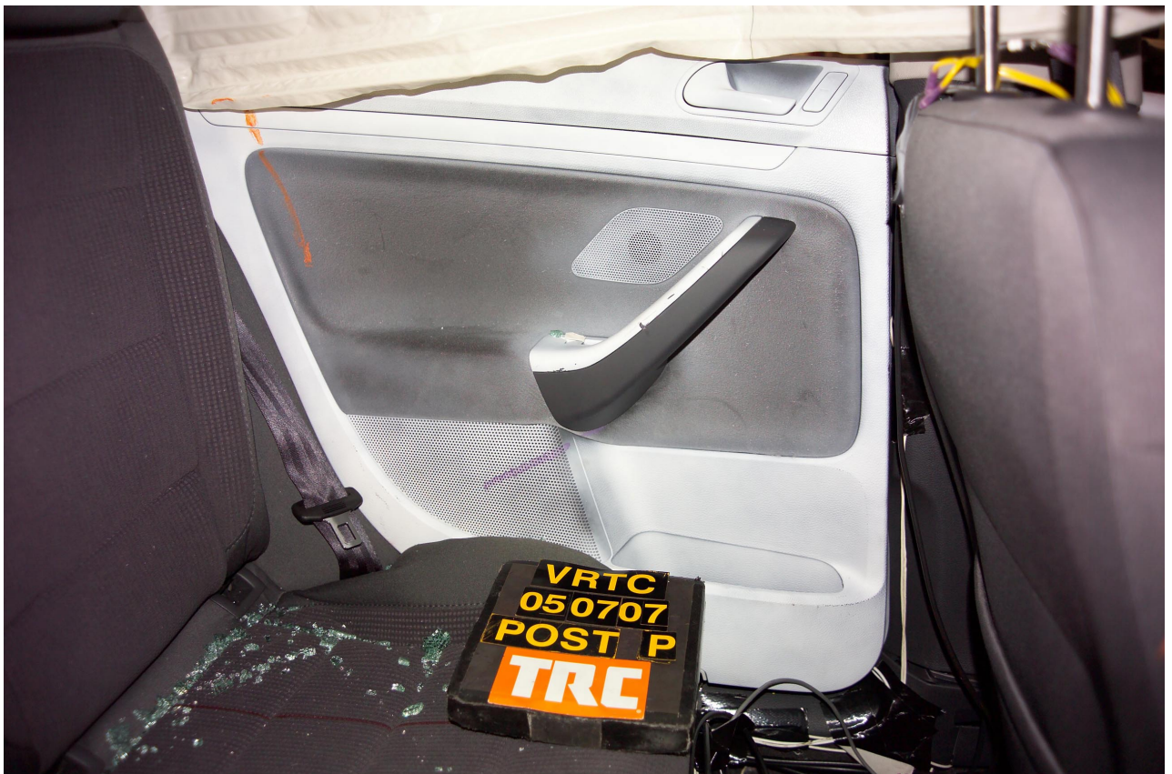
Figure A-64 Post-Test Interior of Rear Door Showing ES-2re Impact Locations
