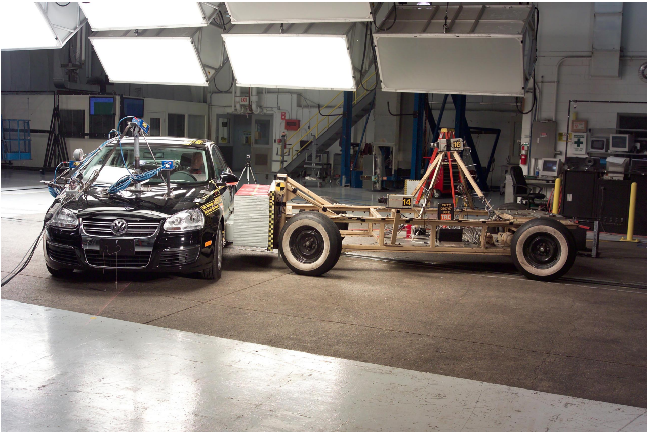
Figure A-17 Pre-Test Front View with MDB in Position
