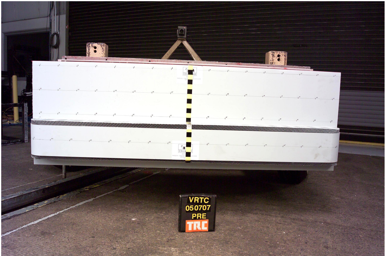
Figure A-73 Pre-Test Barrier Face Front View
