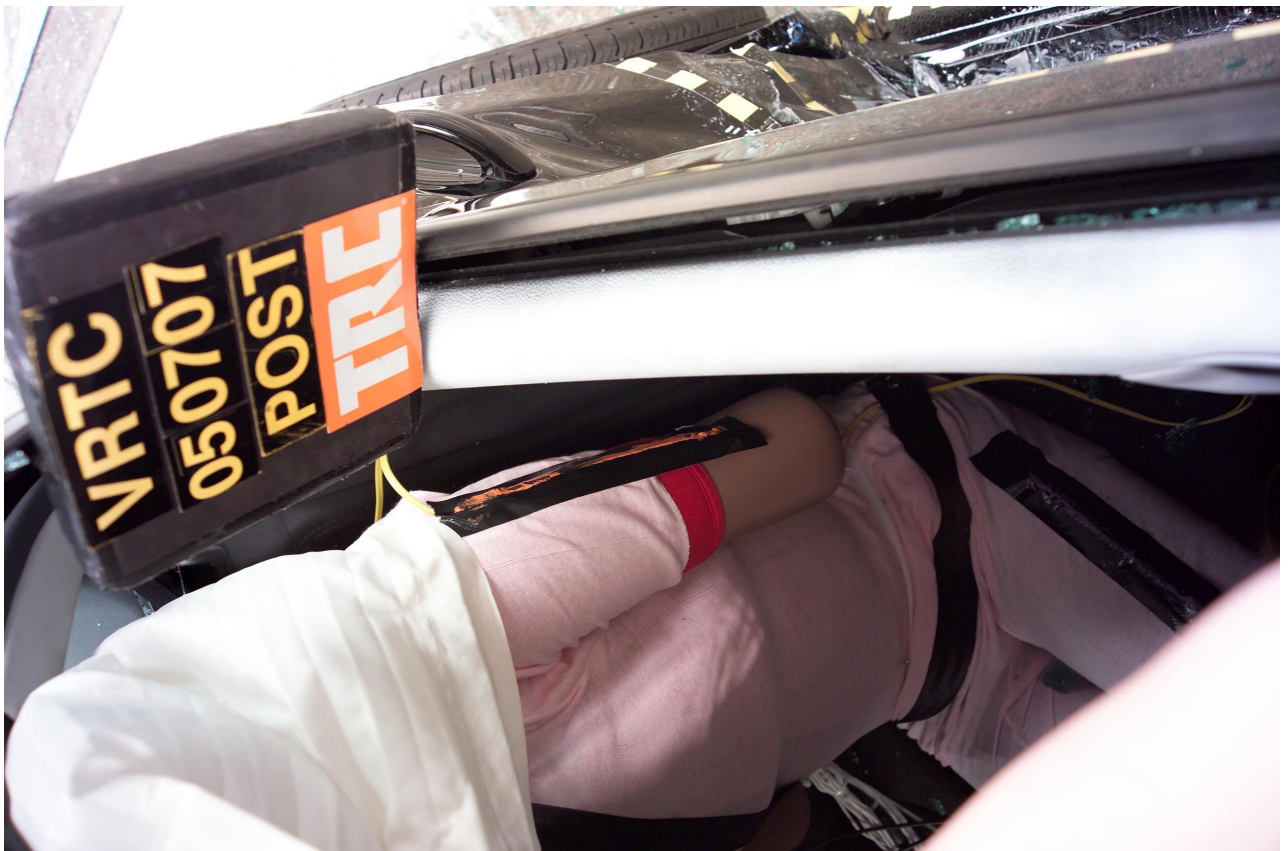
Figure A-57 Post-Test Left View of Rear ES-2re and Door Clearance
