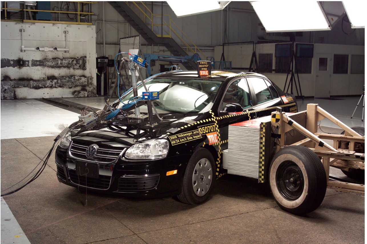
Figure A-21 Pre-Test Left Front View of MDB with Impactor Face in Position
