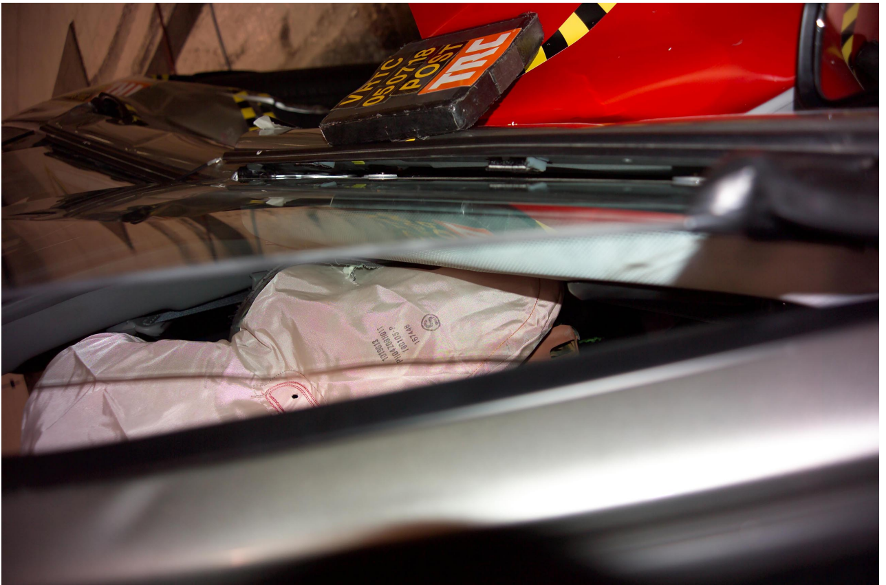
Figure A-57 Post-Test Left View of Rear SID-IIs and Door Clearance
