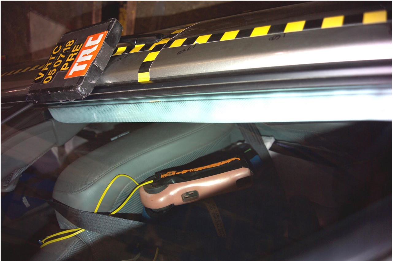
Figure A-51 Pre-Test Left View of Front SID-IIs and Door Clearance
