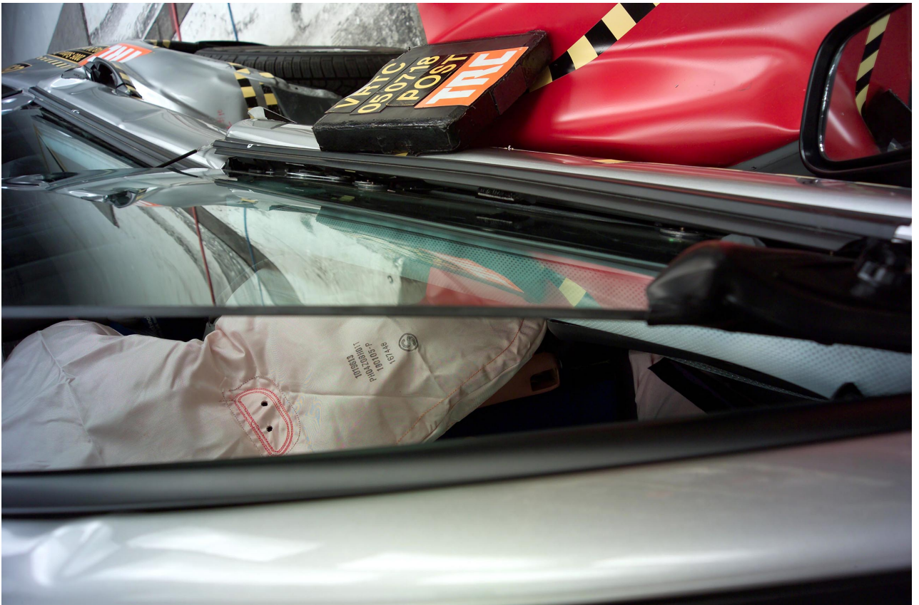
Figure A-52 Post-Test Left View of Front SID-IIs and Door Clearance
