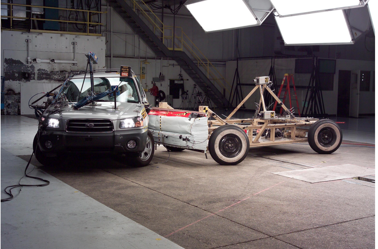
Figure A-17 Post-Test Front View with MDB in Position
