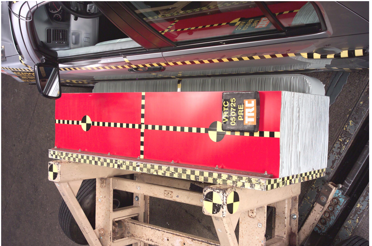
Figure A-27 Pre-Test Overhead View of MDB Aligned with Vehicle
