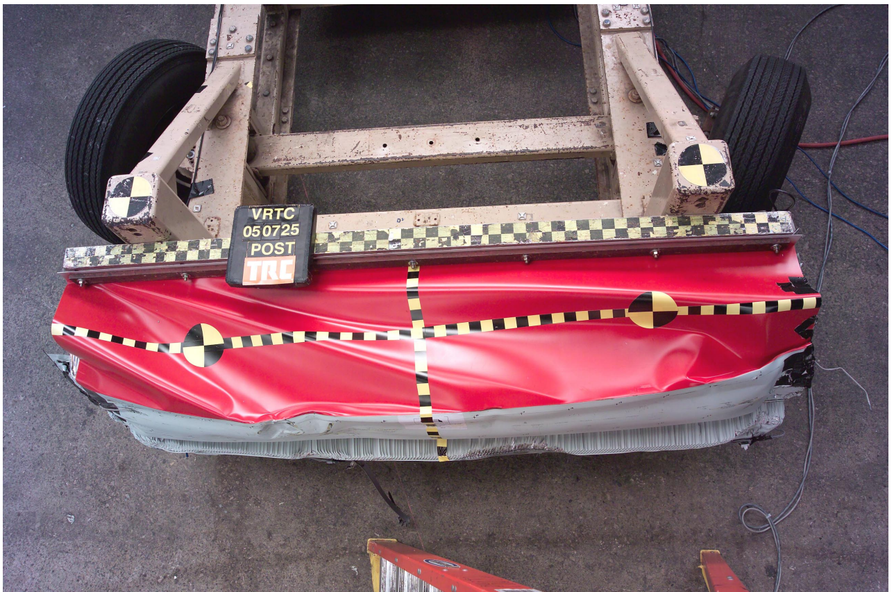
Figure A-74 Post-Test Barrier Face Overhead View
