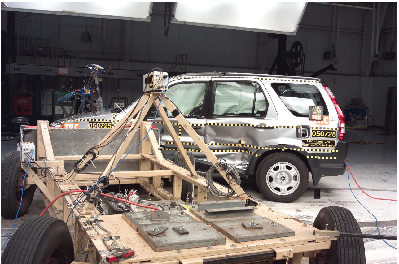
Figure A-24 Post-Test Rear View of MDB with Impactor Face in Position
