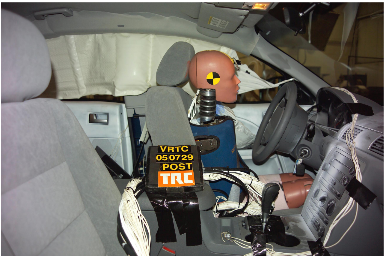
Figure A-46 Post-Test Right Occupant Compartment View of Front SID-IIs
