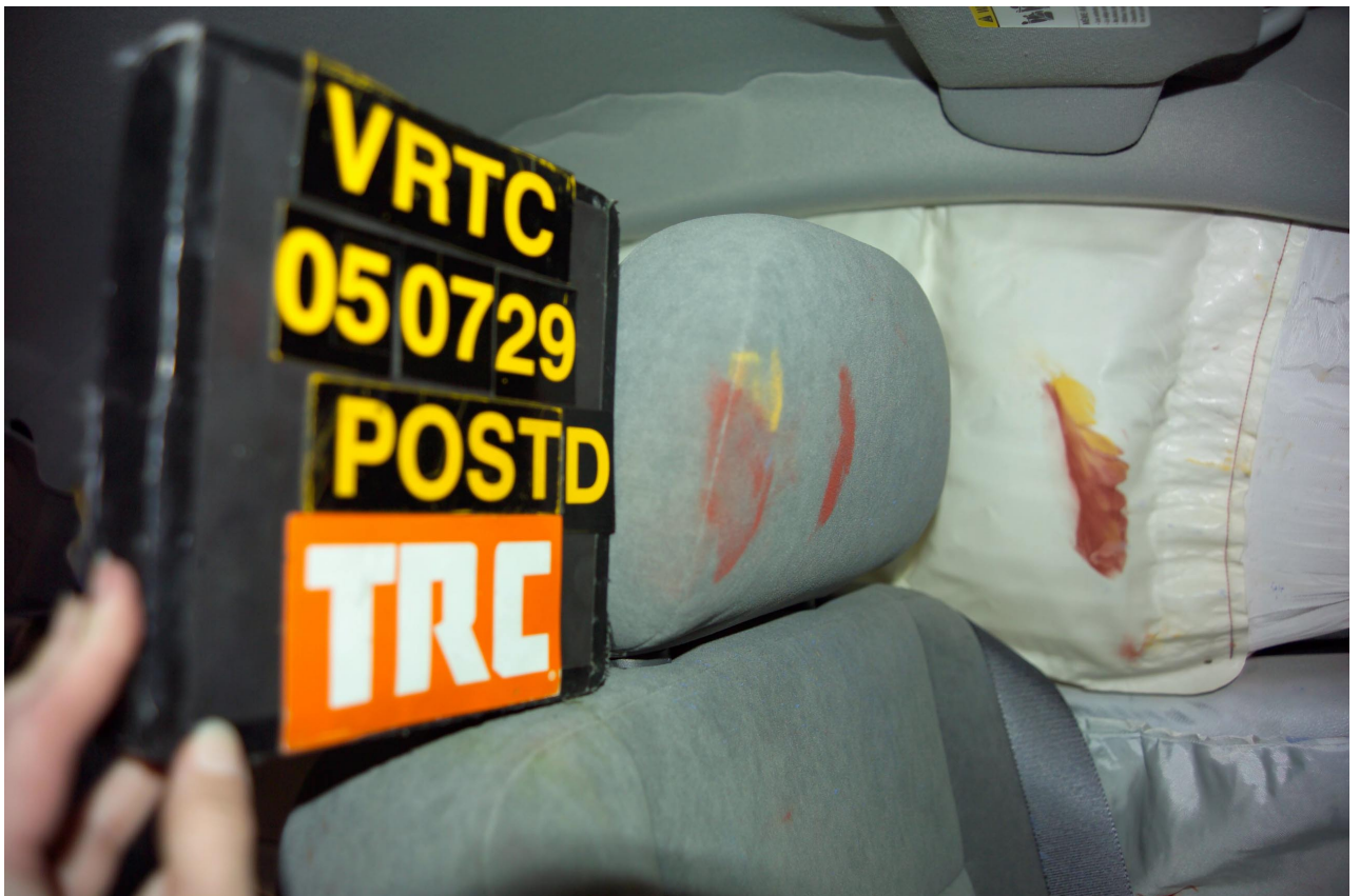
Figure A-62 Post-Test Front SID-II Contact - View 2
