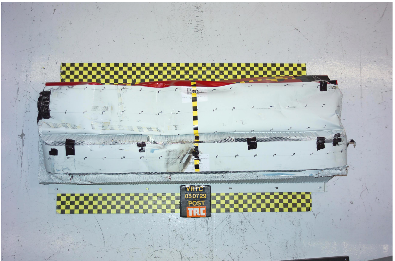
Figure A-30 Post-Test Frontal View of Impactor Face
