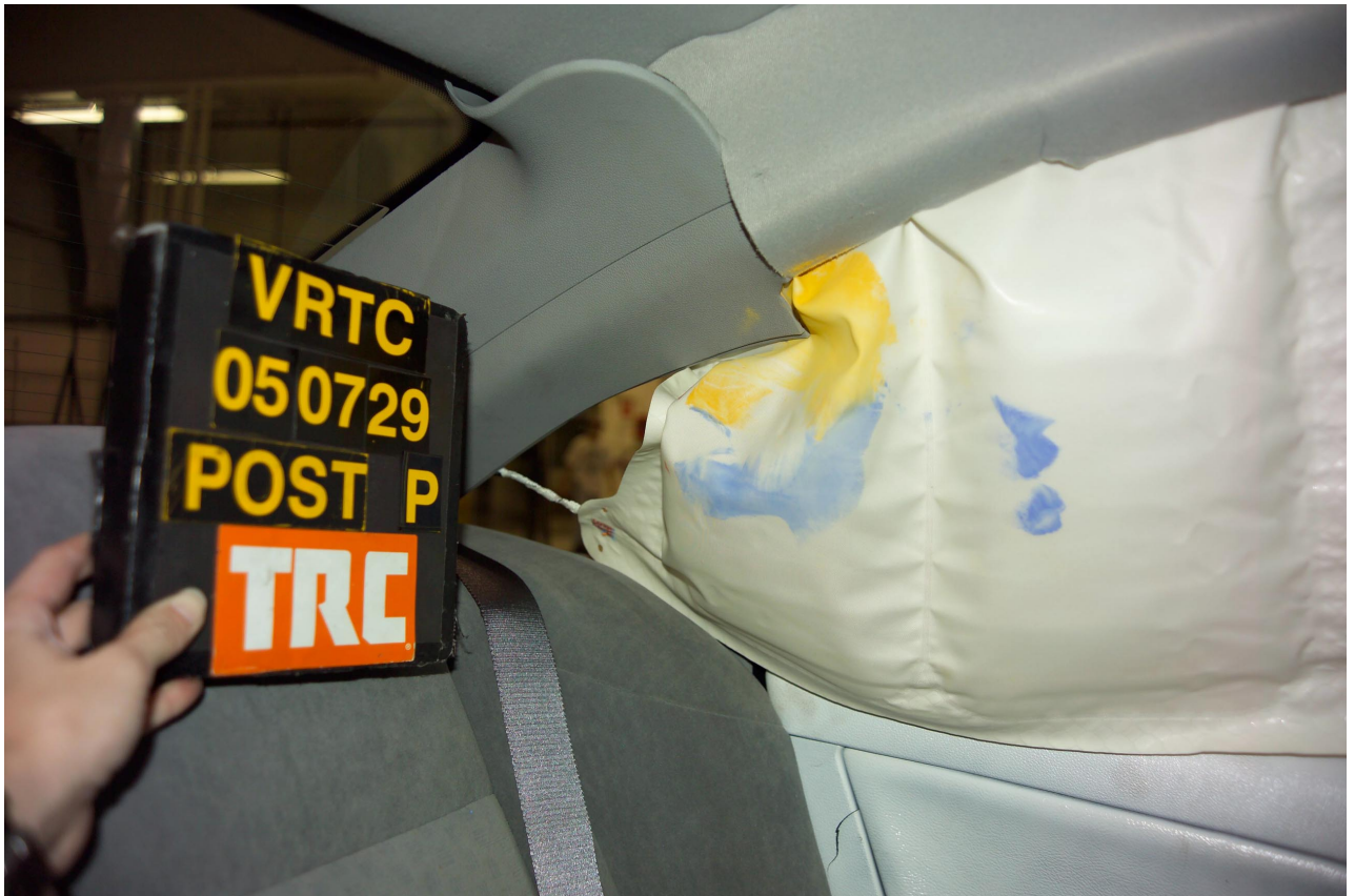
Figure A-66 Post-Test Rear SID-IIs Contact - View 1
