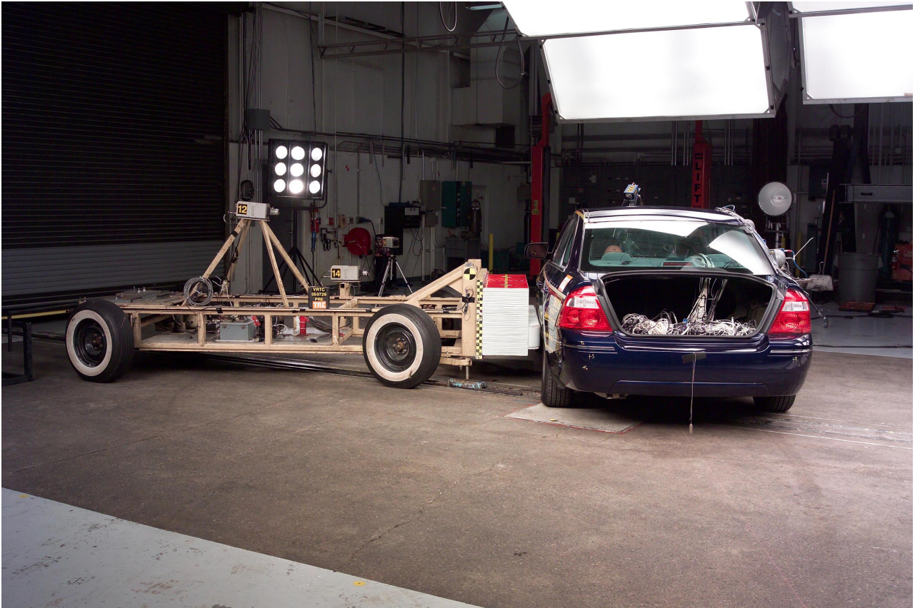
Figure A-19 Pre-Test Rear View with MDB in Position
