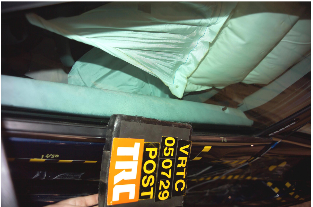
Figure A-53 Post-Test Left View of Front SID-IIs and Door Clearance
