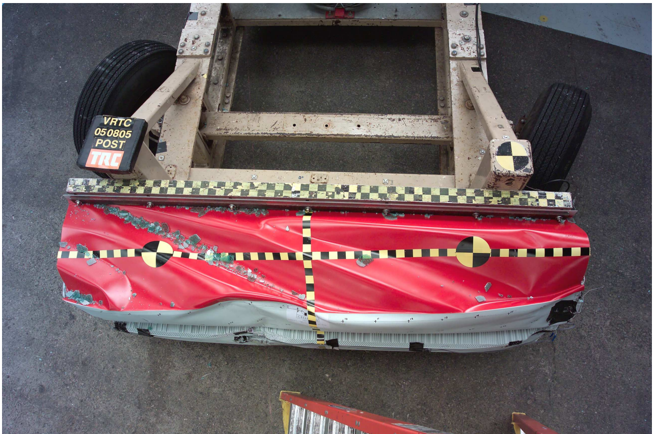
Figure A-75 Post-Test Barrier Face Overhead View
