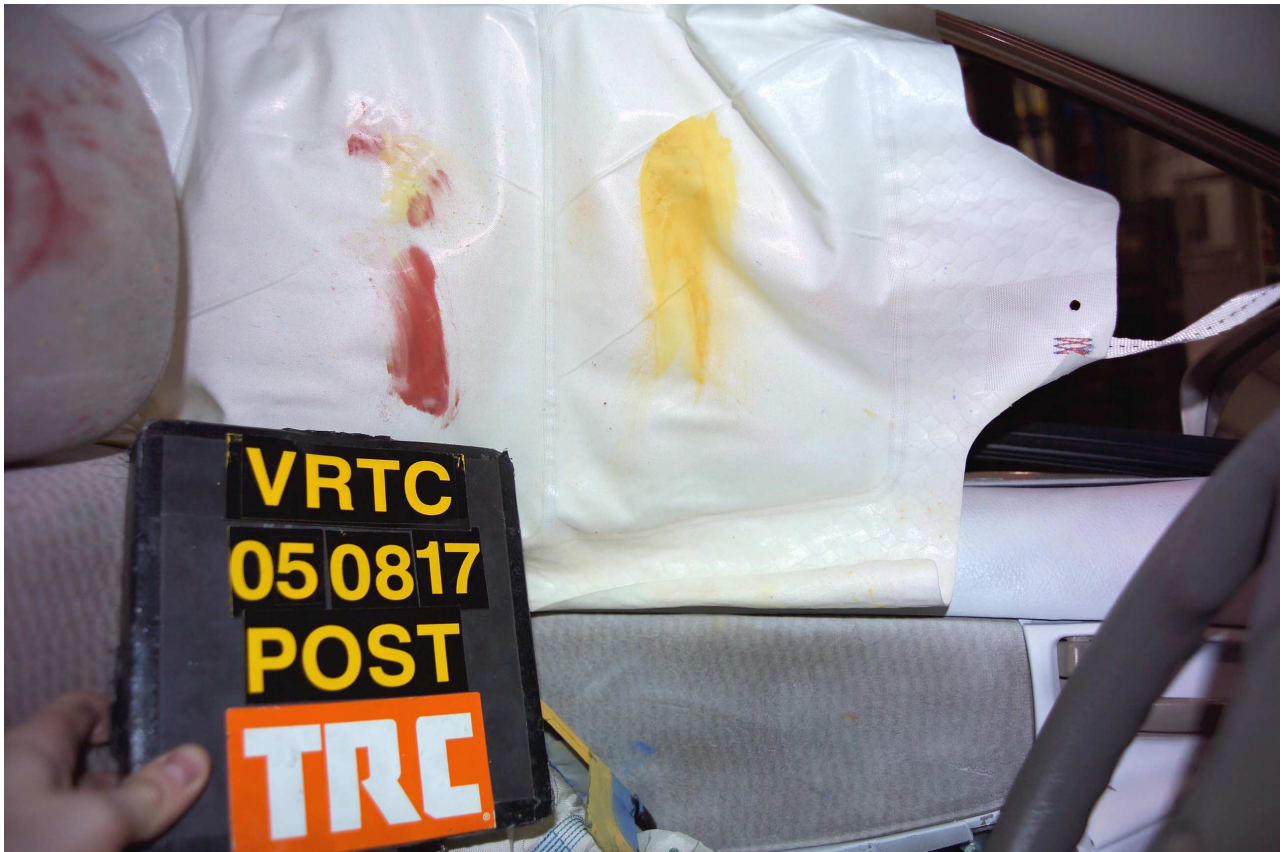
Figure A-61 Post-Test Front SID-II Contact - View 1
