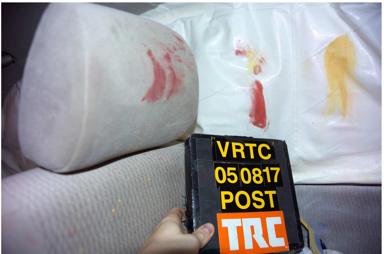
Figure A-62 Post-Test Front SID-II Contact - View 2
