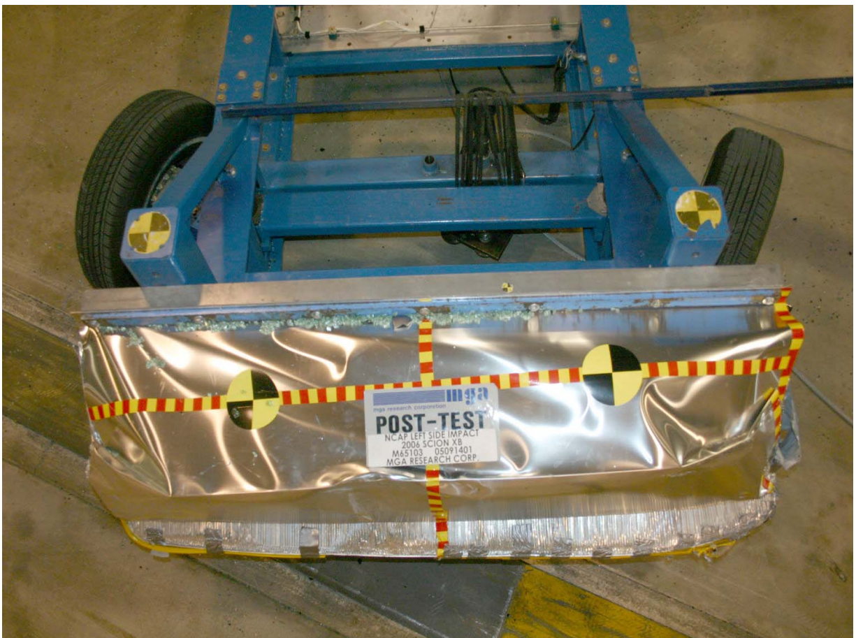
Post-Test Front View of Deformable Barrier
