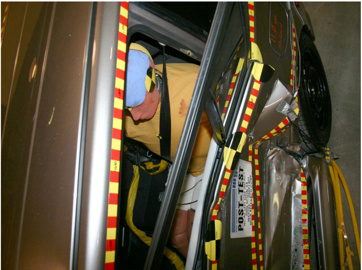
Post-Test Passenger Dummy Clearance From Door
