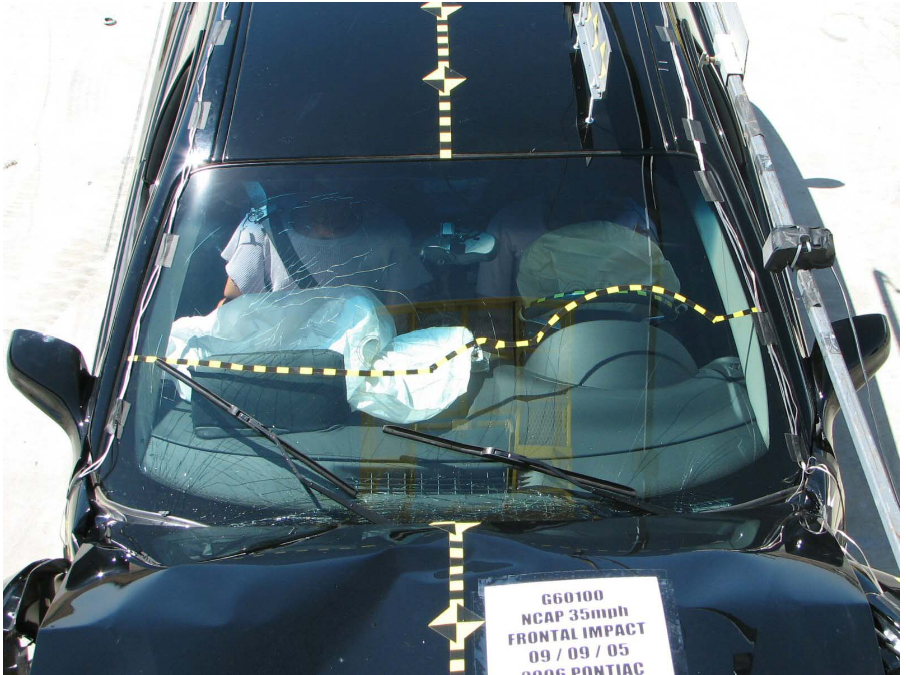
Figure A-19: Post-Test Windshield
