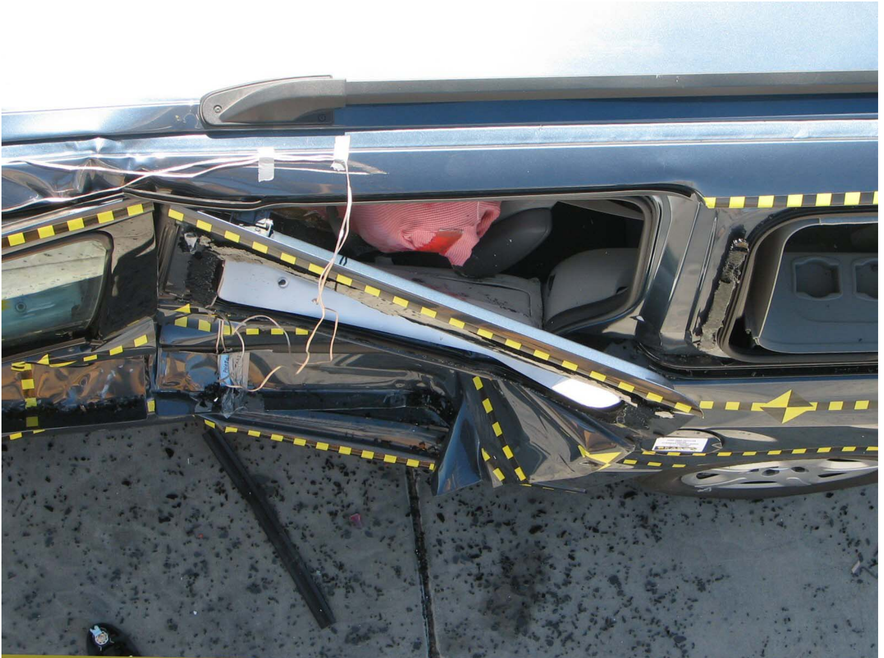
Figure A-48: Post-Test Passenger Dummy Clearance From Door
