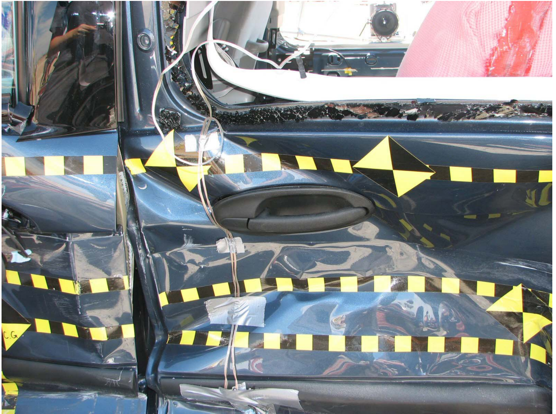
Figure A-34: Post-Test Left Rear Door
