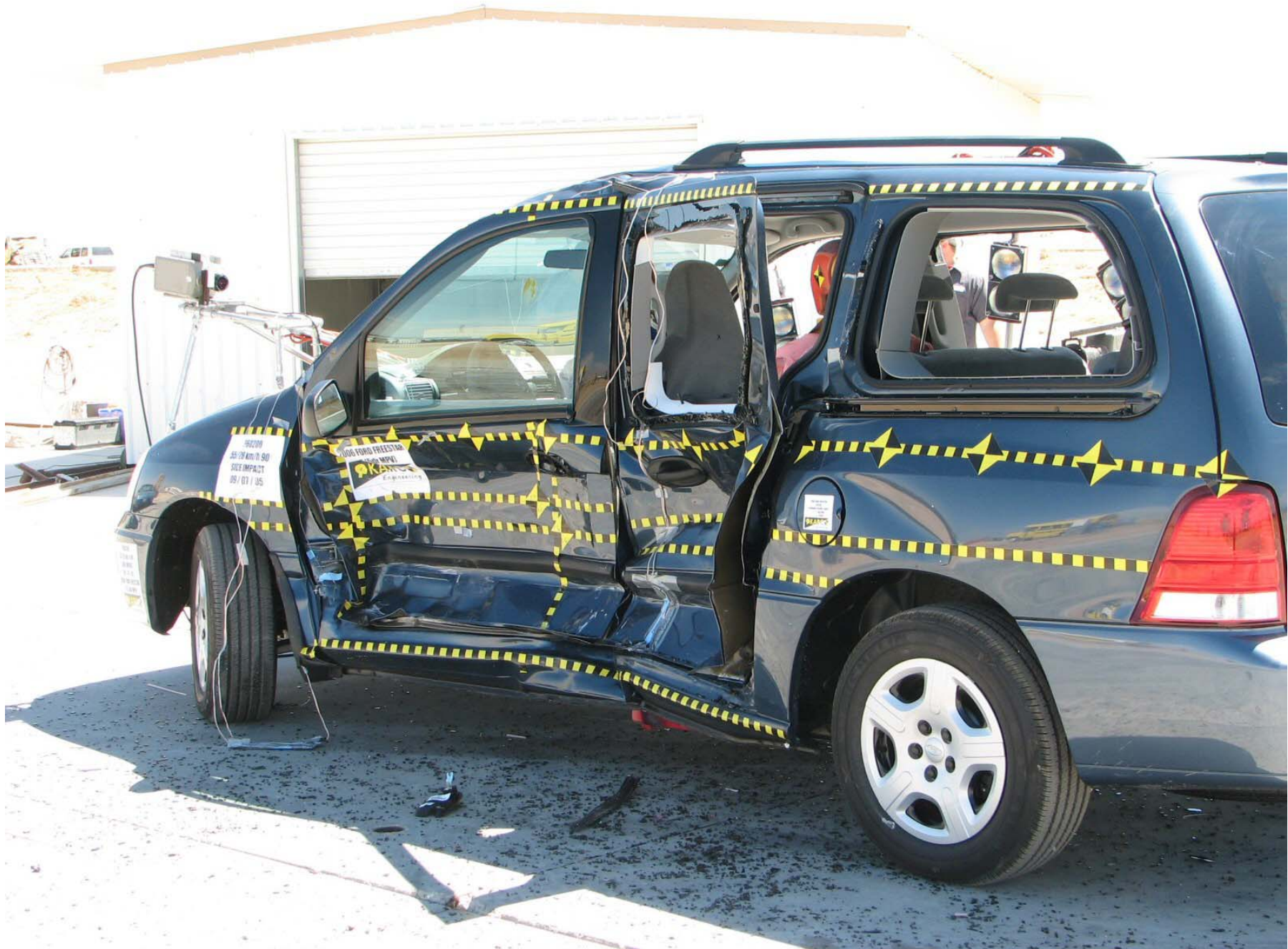
Figure A-30: Post-Test Rear ¾ View of Left Side Doors
