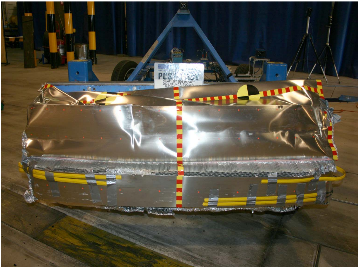
Post-Test Front View of Deformable Barrier
