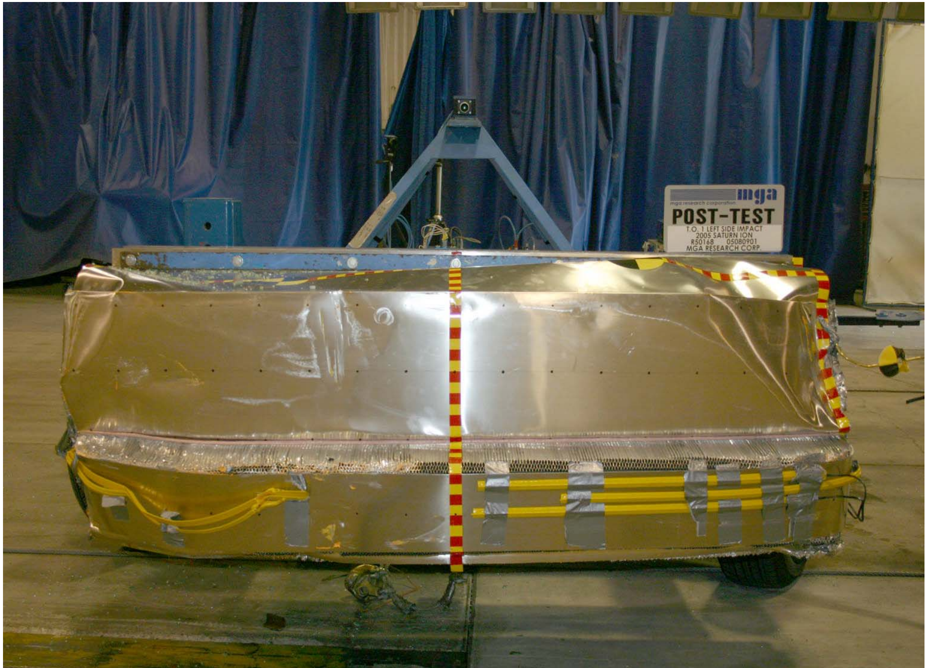
Post-Test MDB Front View
