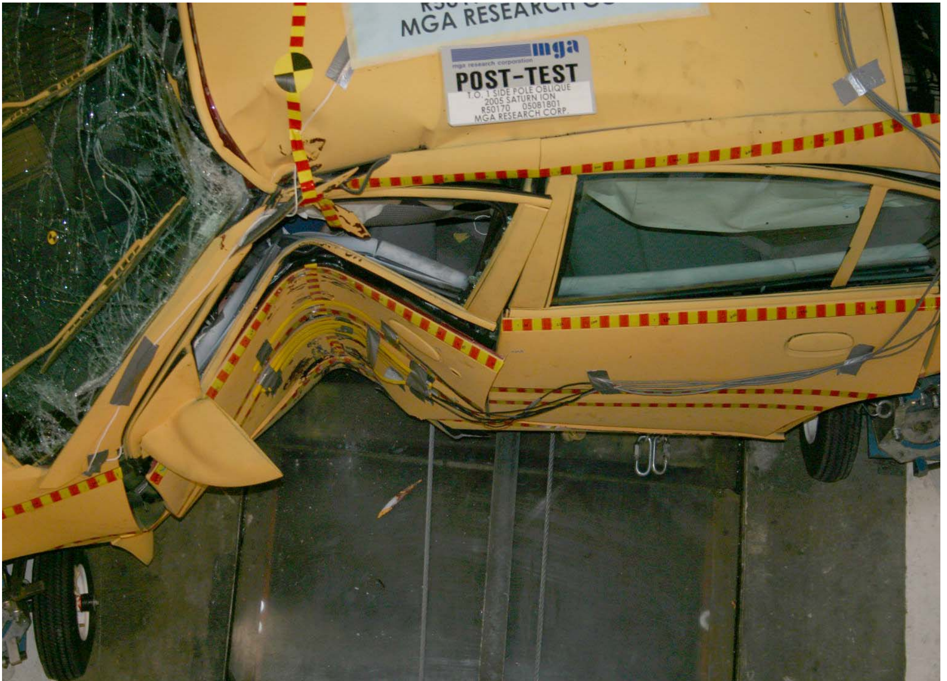
Post-Test Vehicle Overhead View (Close Up)
