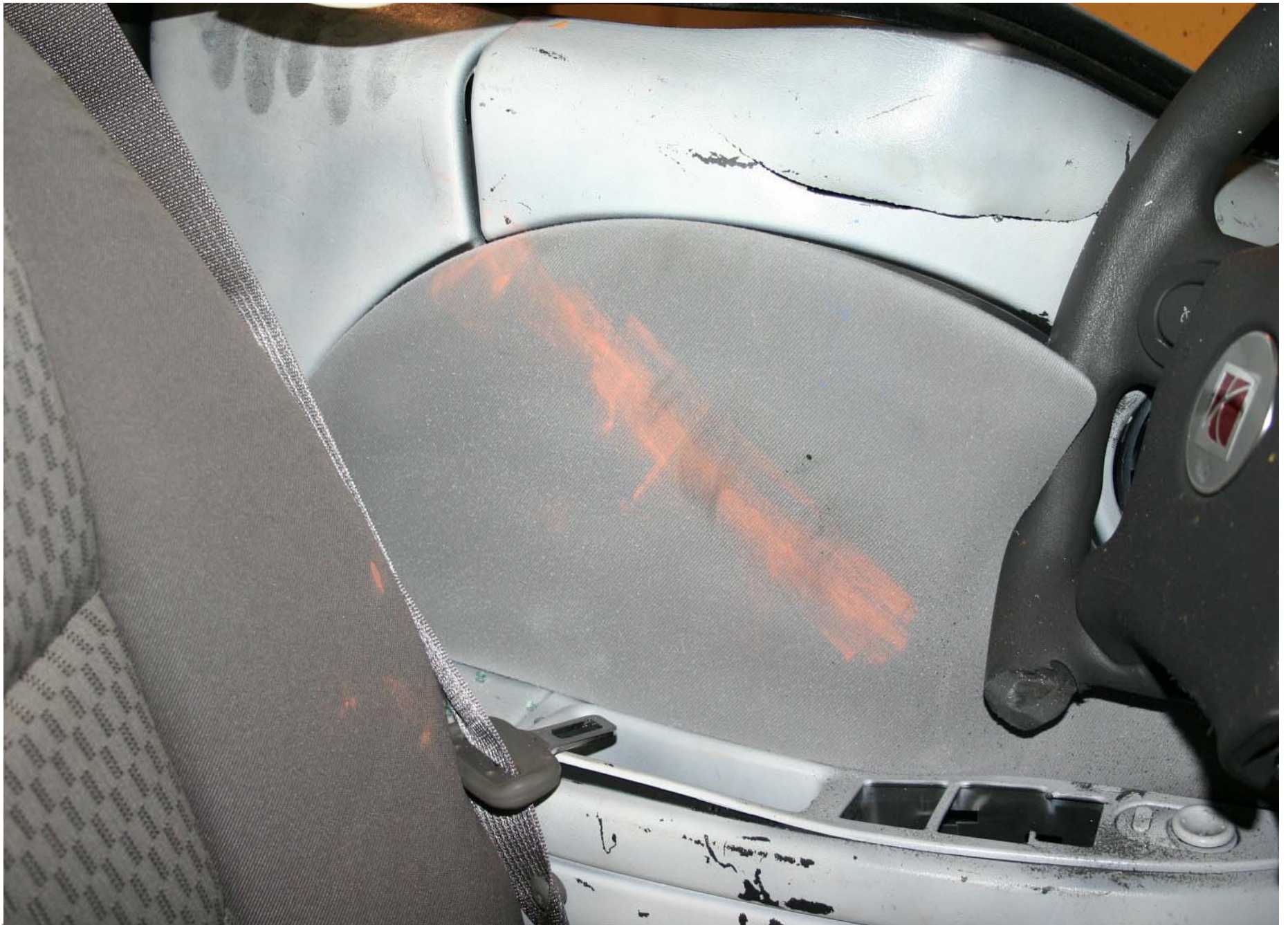
Post-Test Driver Dummy Arm Contact
