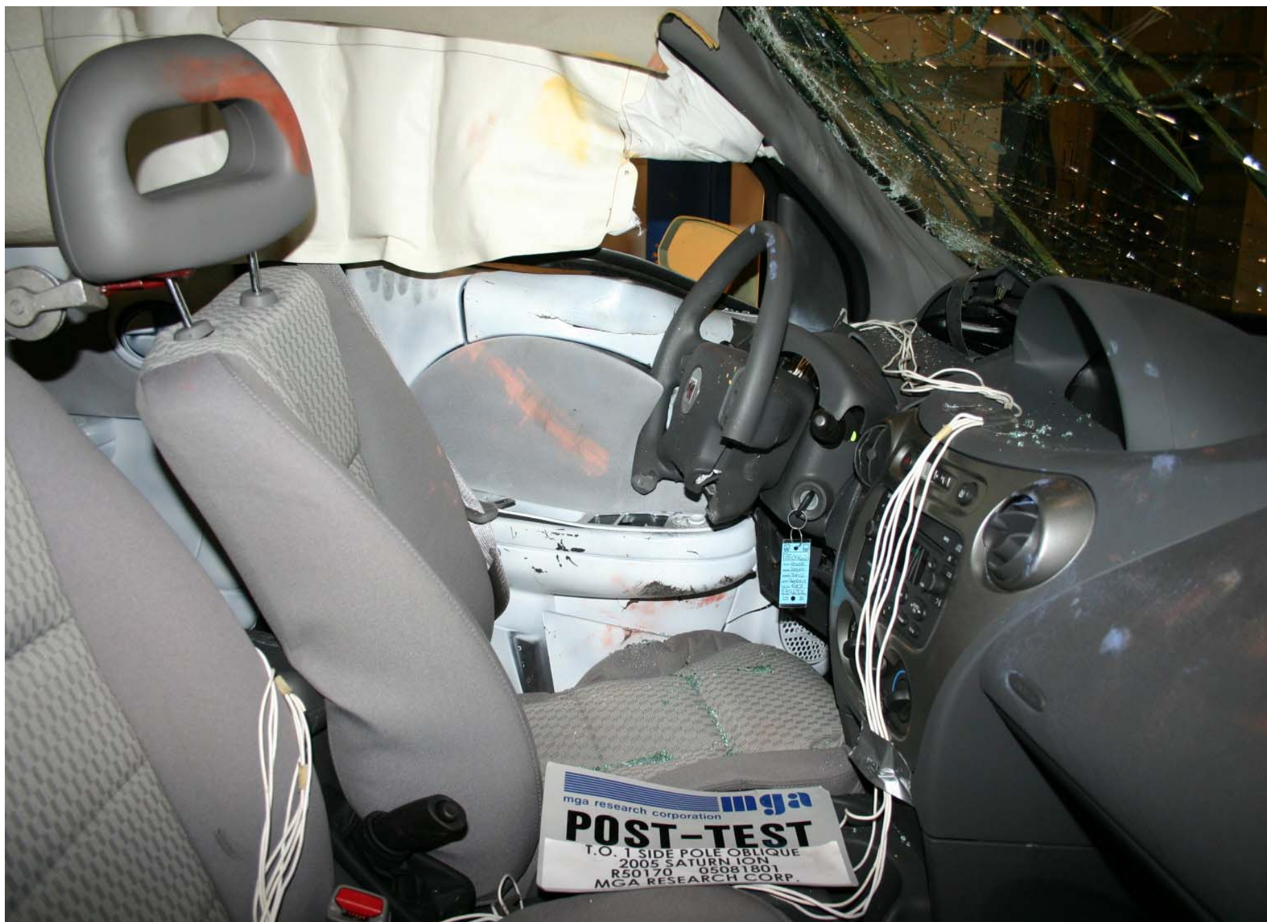
Post-Test Driver Dummy Contact
