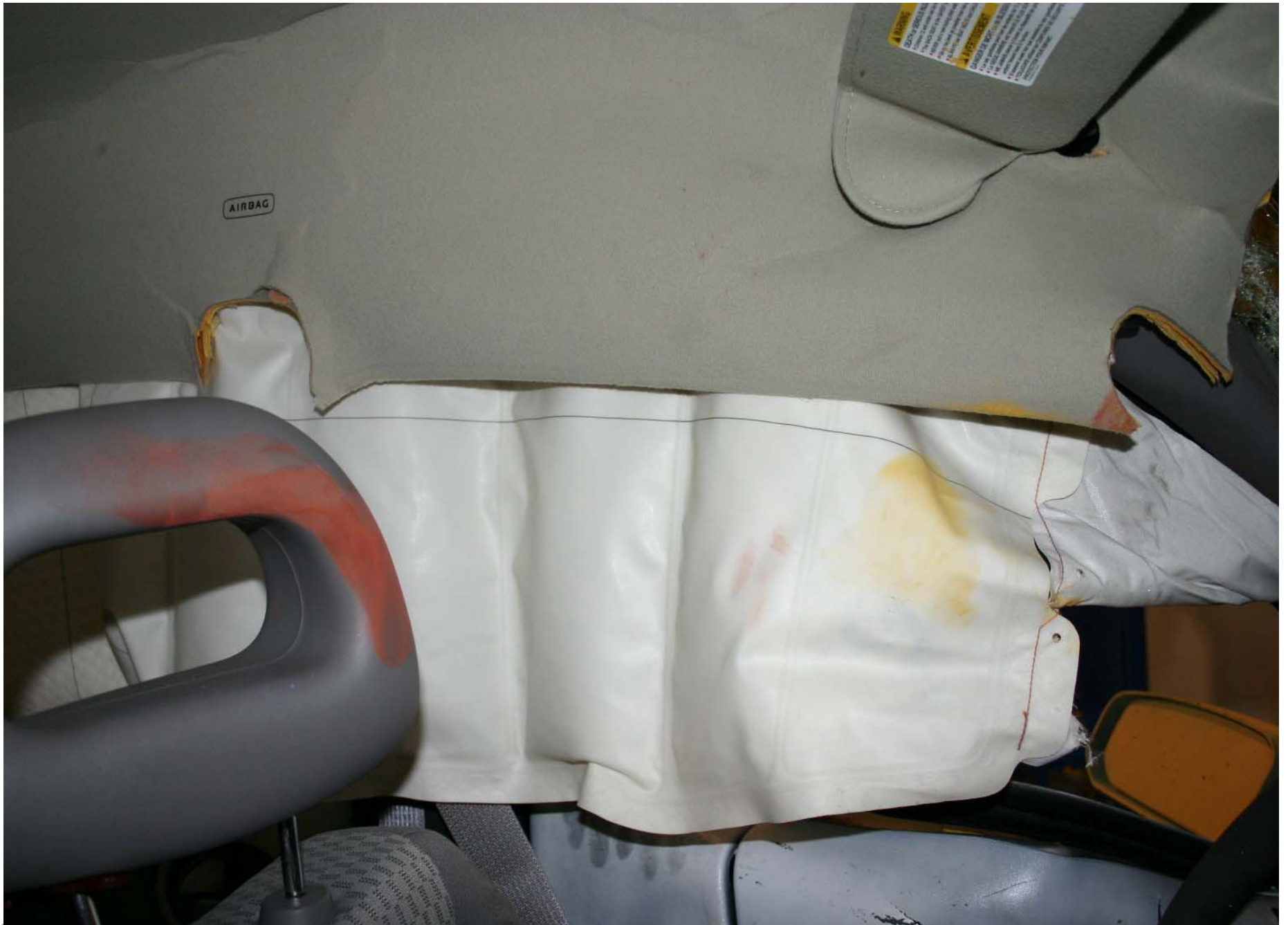
Post-Test Driver Dummy Head Contact
