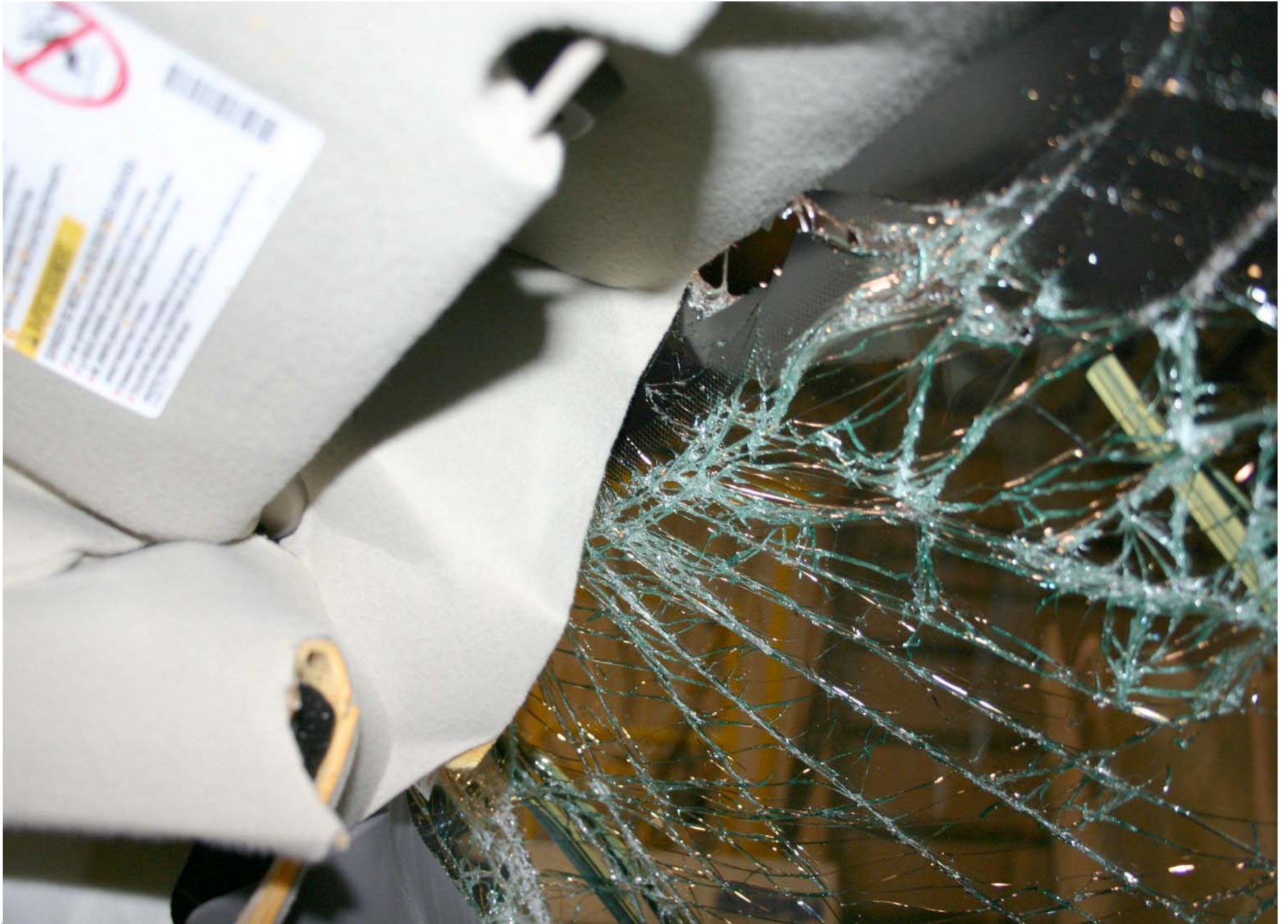
Post-Test Windshield Retention
