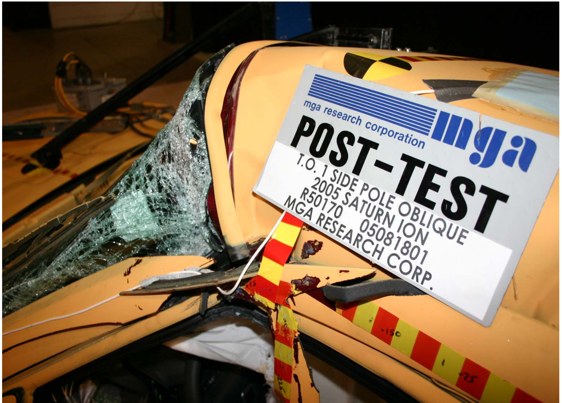
Post-Test Windshield Retention
