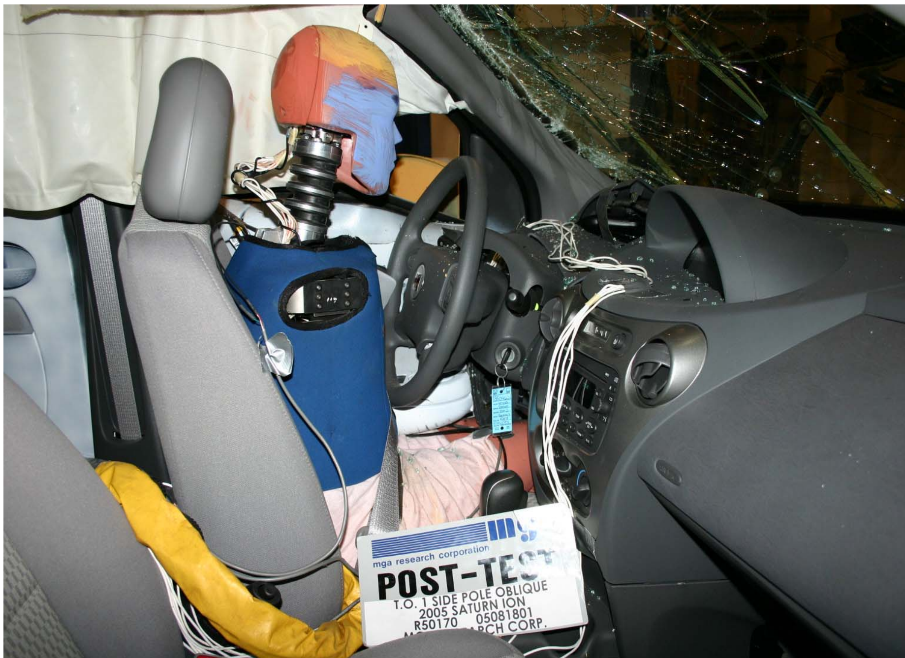
Post-Test Driver Dummy Right Side View
