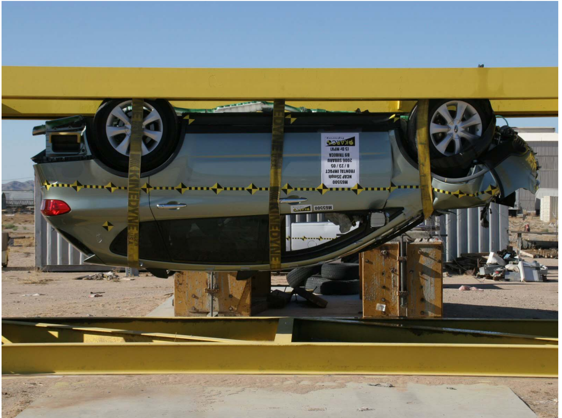
Figure A-60: Vehicle on Rollover Device (180°)
