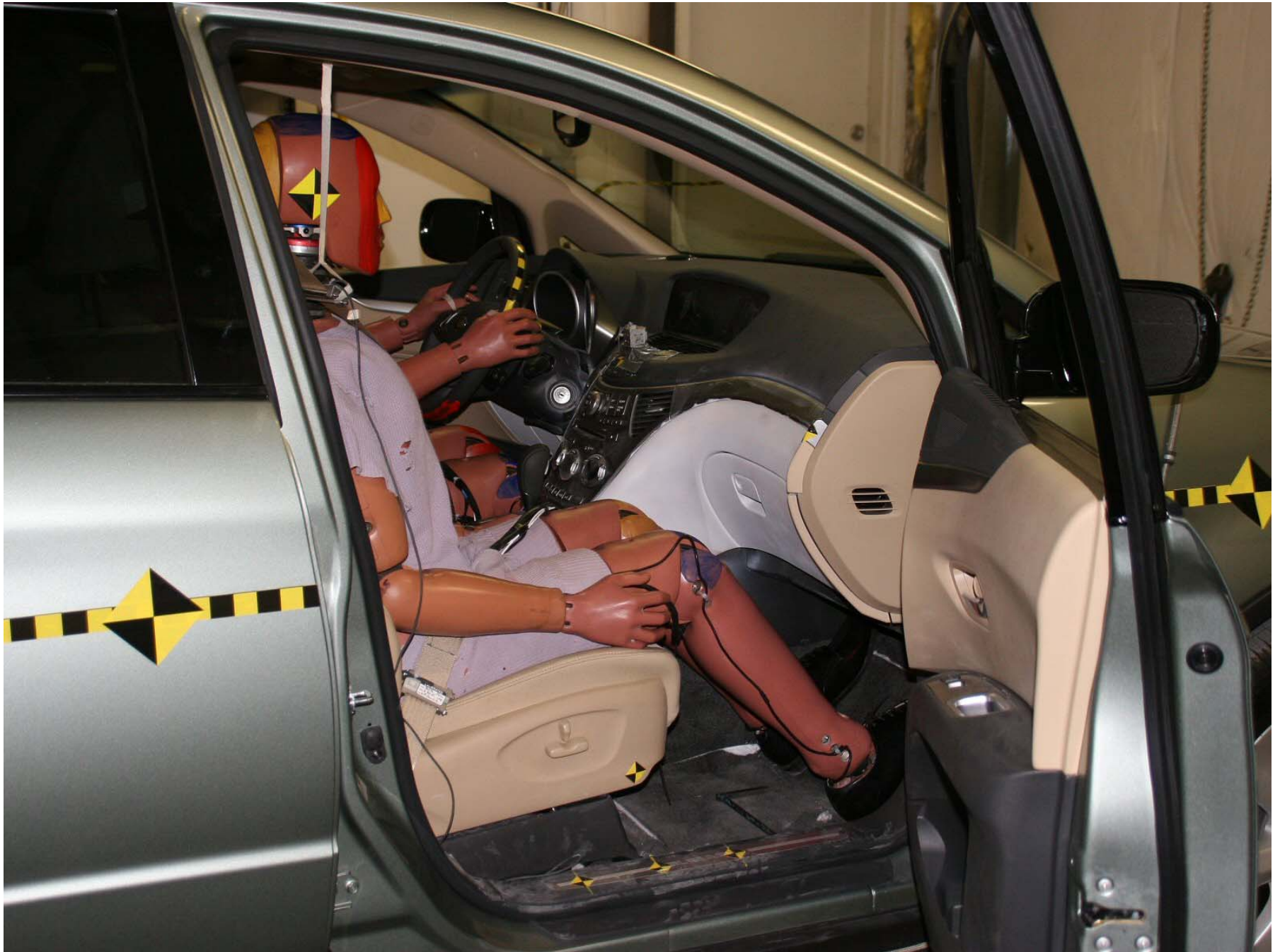
Figure A-48: Pre-Test Passenger Dummy (Door Open)
