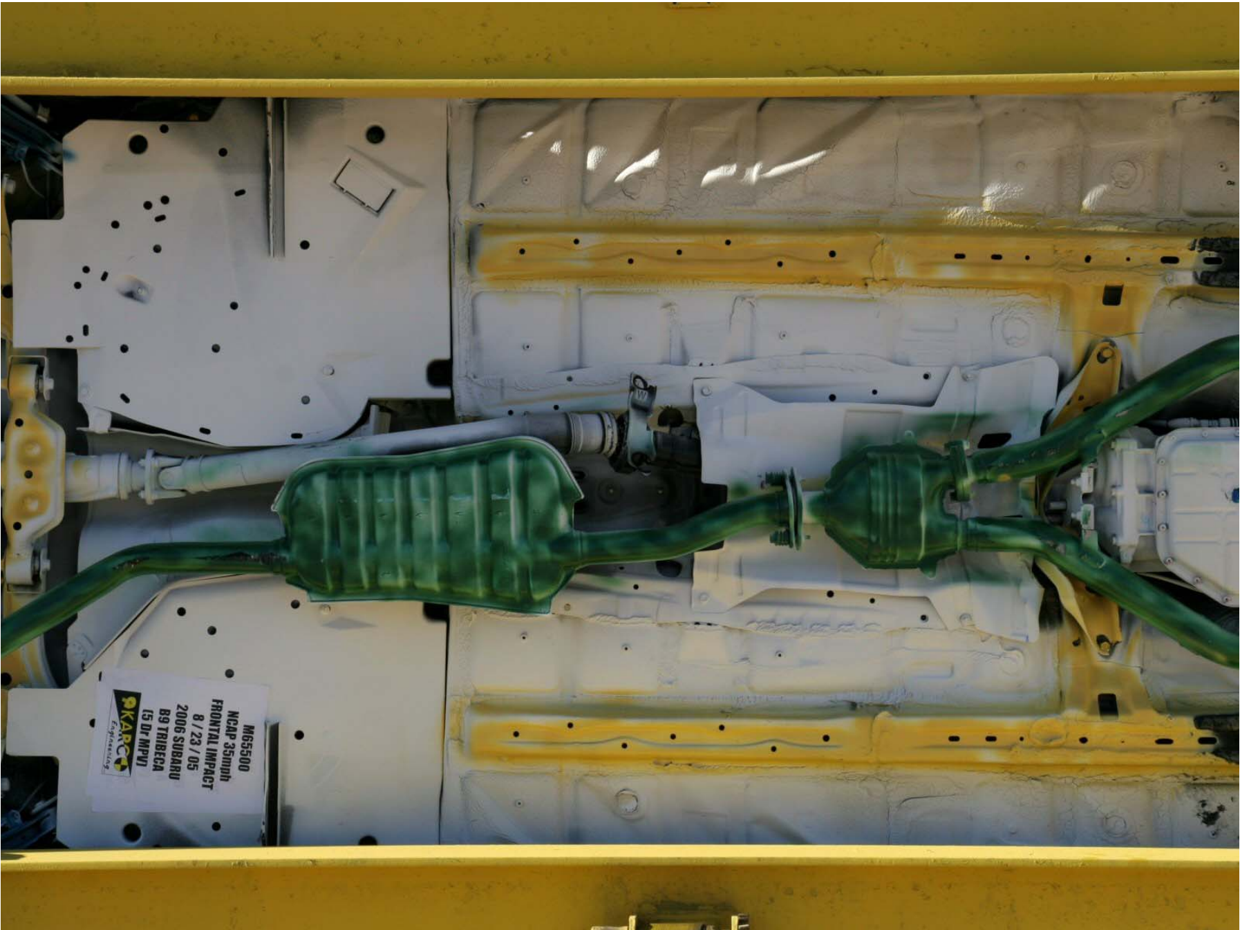
Figure A-27: Post-Test Mid Underbody
