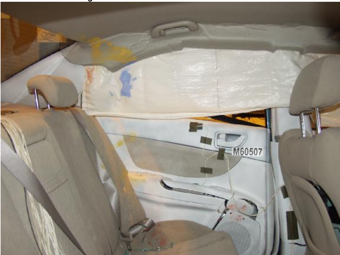
Figure A-46: Post-Test Left Rear Interior Trim
