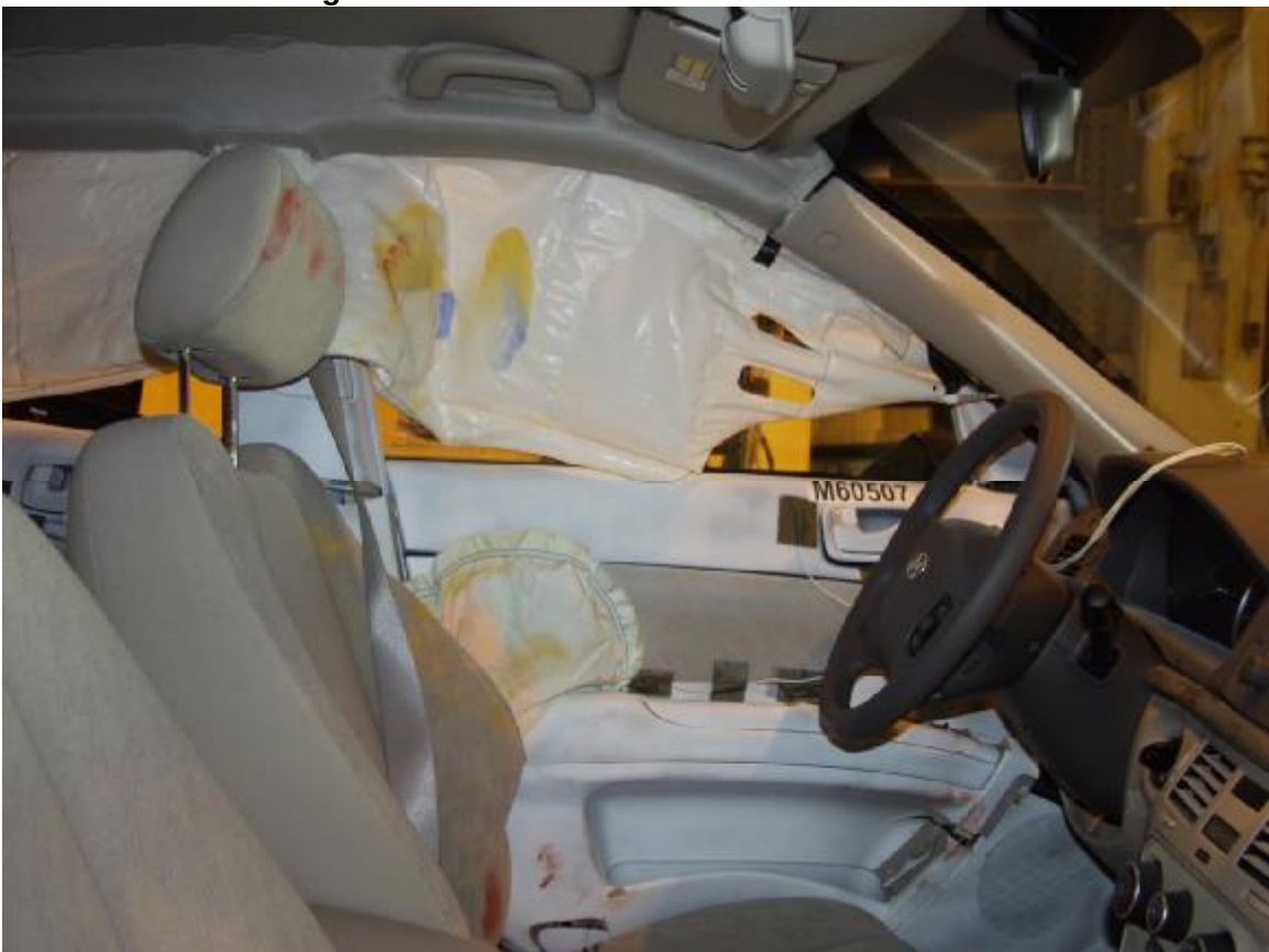
Figure A-44: Post-Test Left Front Interior Trim
