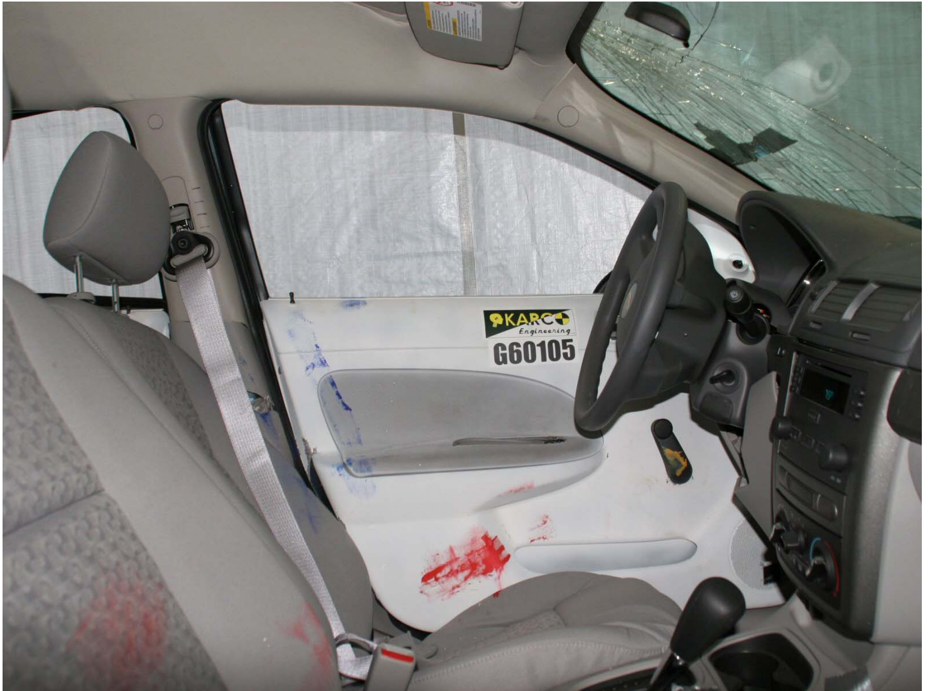
Figure A-43: Post-Test Front Door Panel (Interior)
