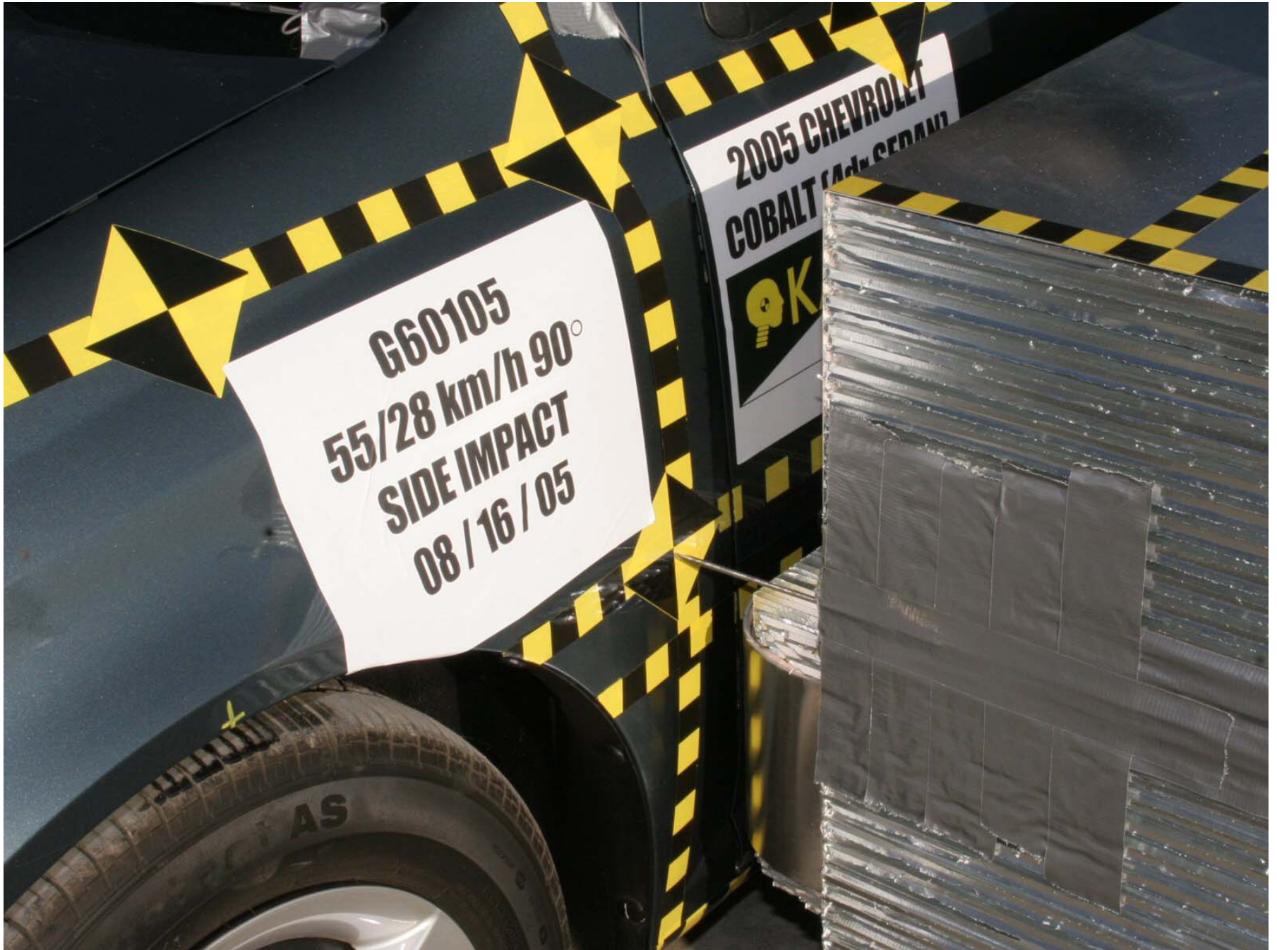
Figure A-25: Pre-Test Left Impact Point
