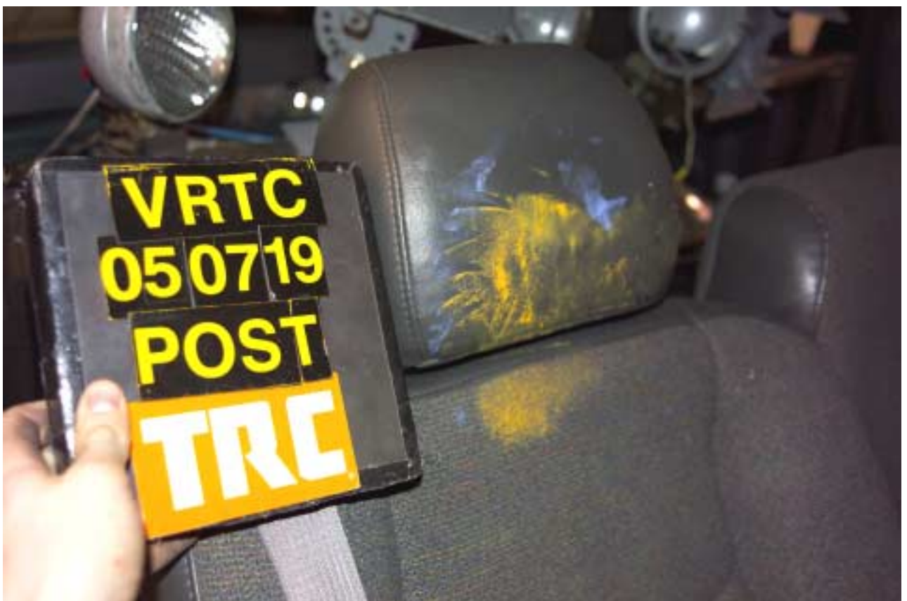
Figure A-124 Post-Test Bullet Vehicle Passenger Dummy Head Contact - View 3
