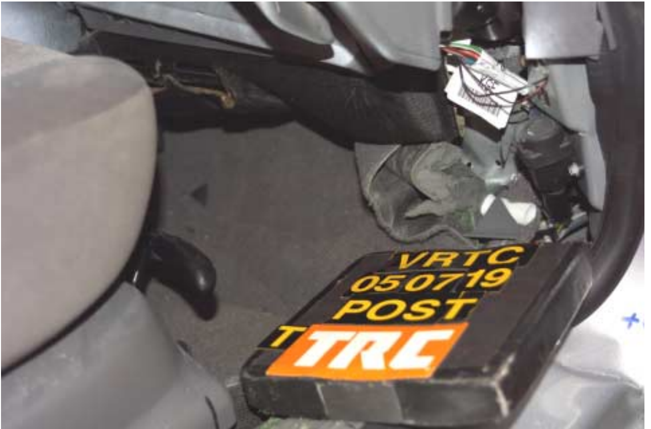
Figure A-129 Post-Test Target Vehicle Passenger Floorboard Deformation View
