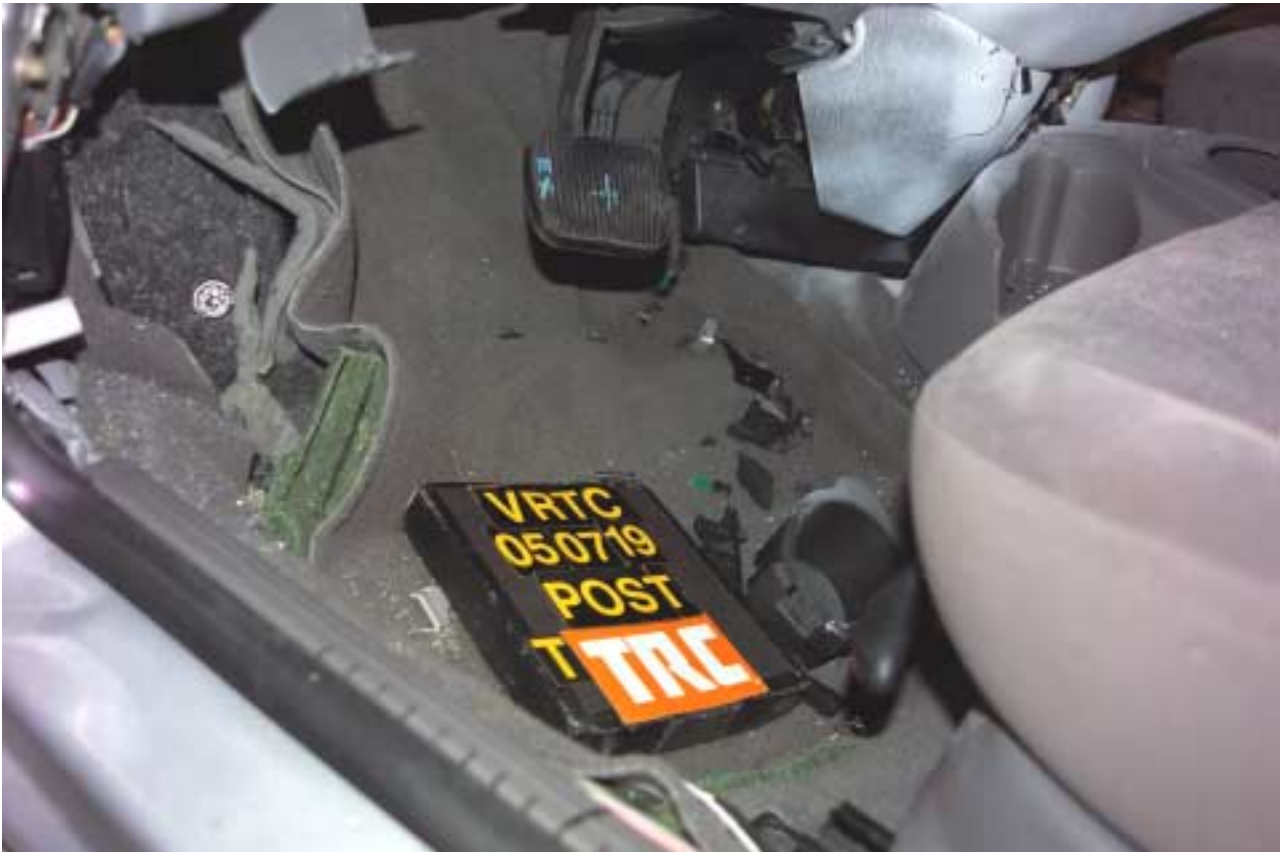
Figure A-127 Post-Test Target Vehicle Driver Floorboard Deformation View
