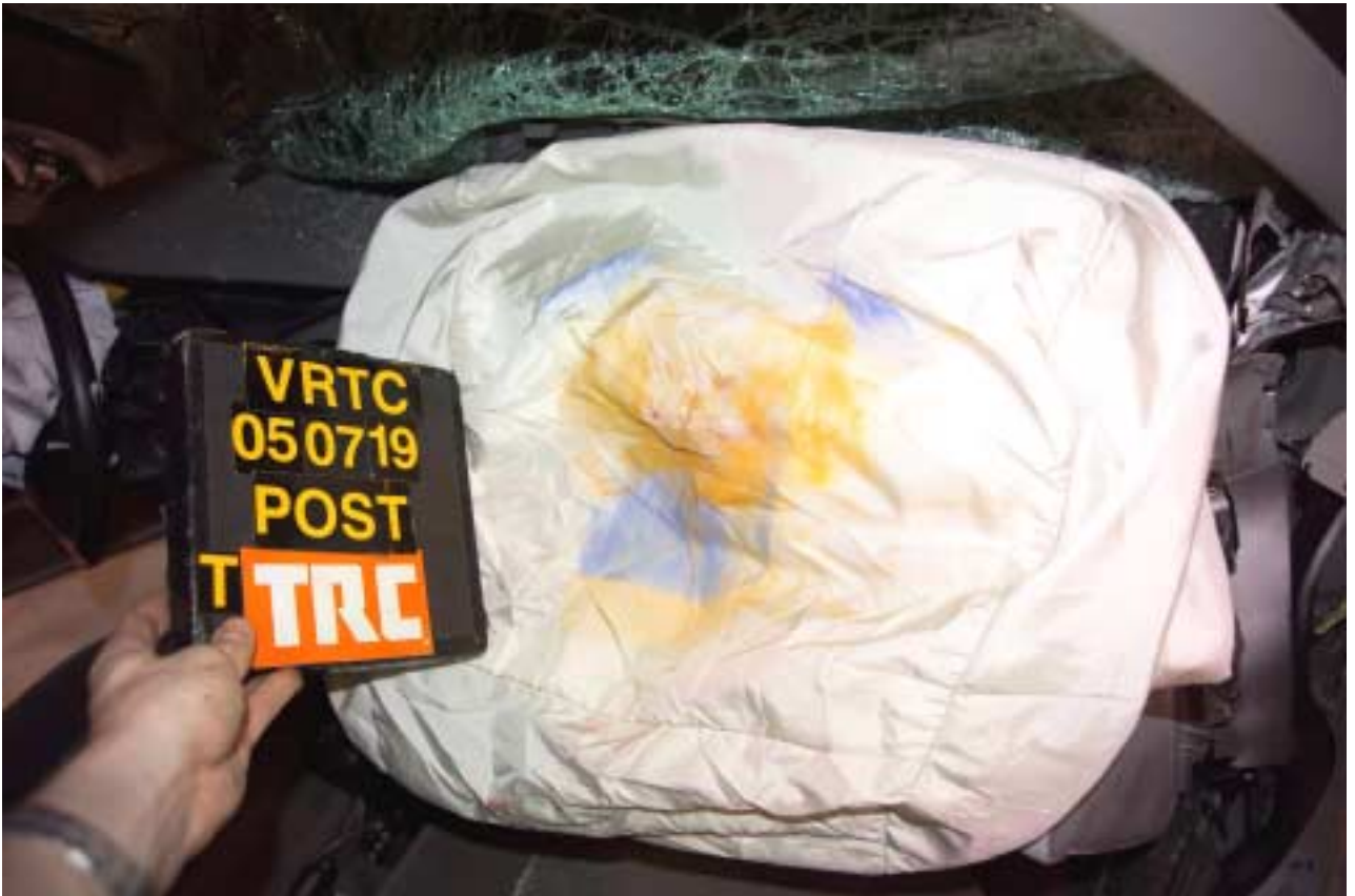
Figure A-111 Post-Test Target Vehicle Passenger Dummy Head Contact - View 2
