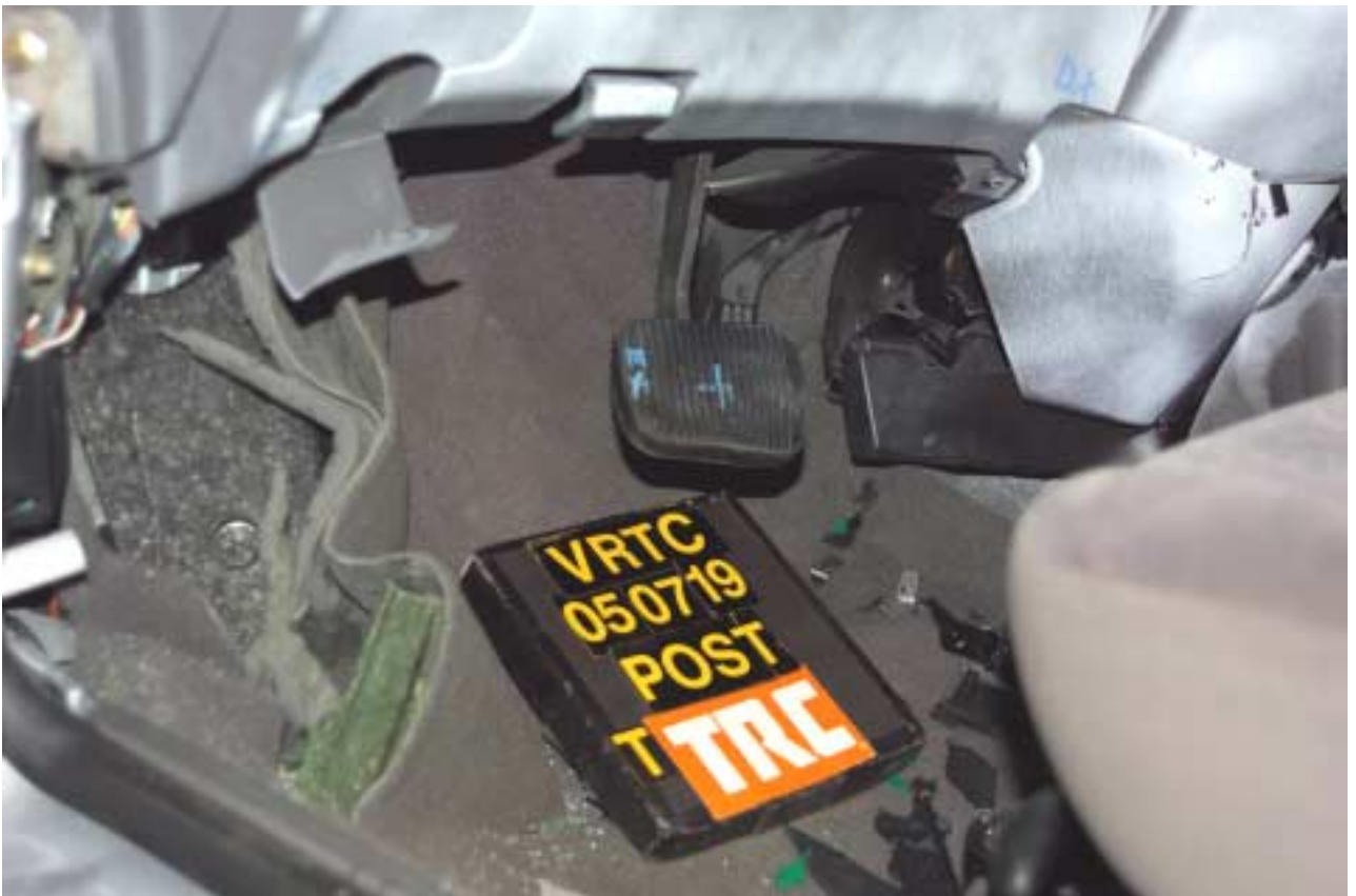
Figure A-128 Post-Test Target Vehicle Driver Toeboard Deformation View
