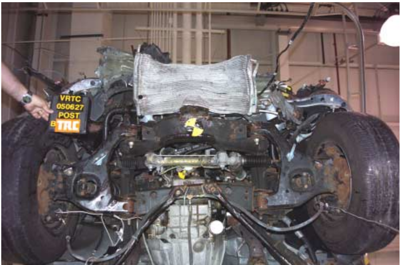
Figure A-61 Post-Test Bullet Vehicle Front Underbody View
