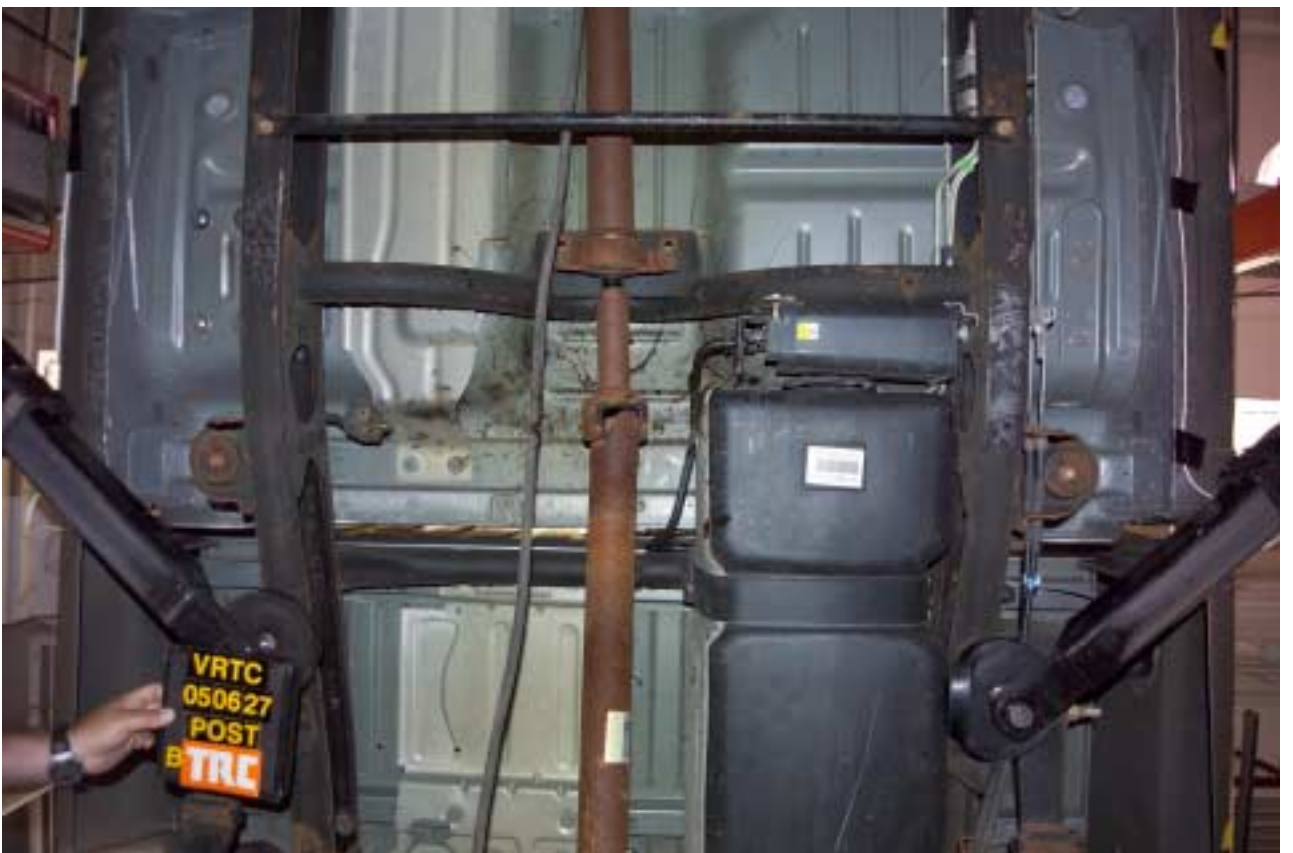
Figure A-67 Post-Test Bullet Vehicle Mid Underbody - View 2
