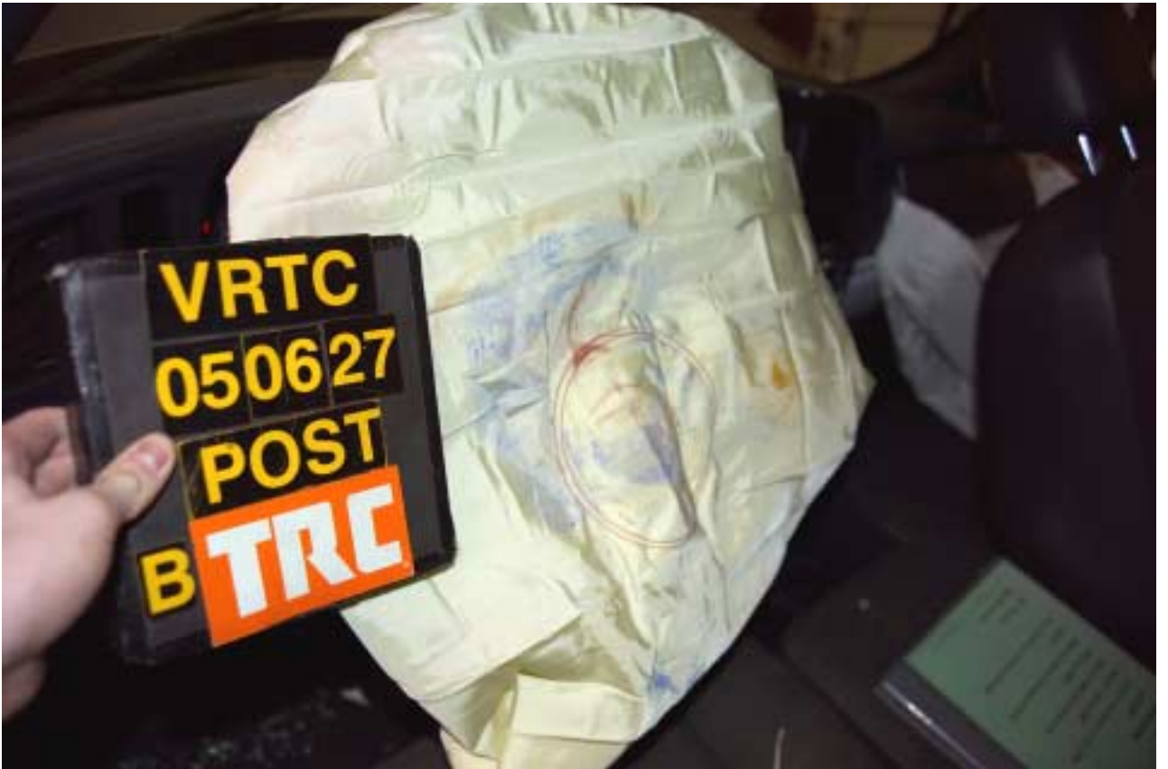
Figure A-125 Post-Test Bullet Vehicle Driver Dummy Head Contact - View 2
