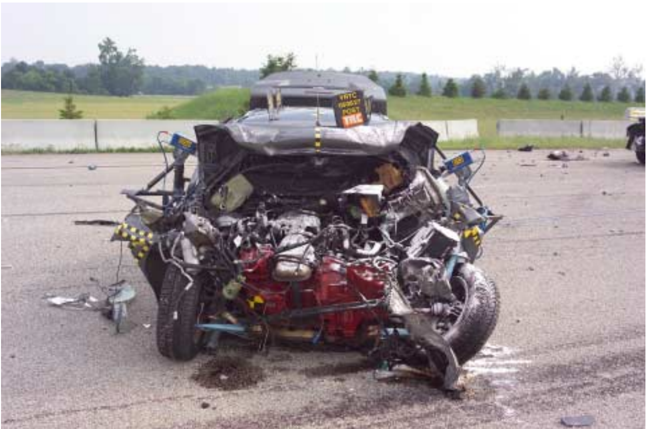
Figure A-16 Post-Test Target Vehicle Front View
