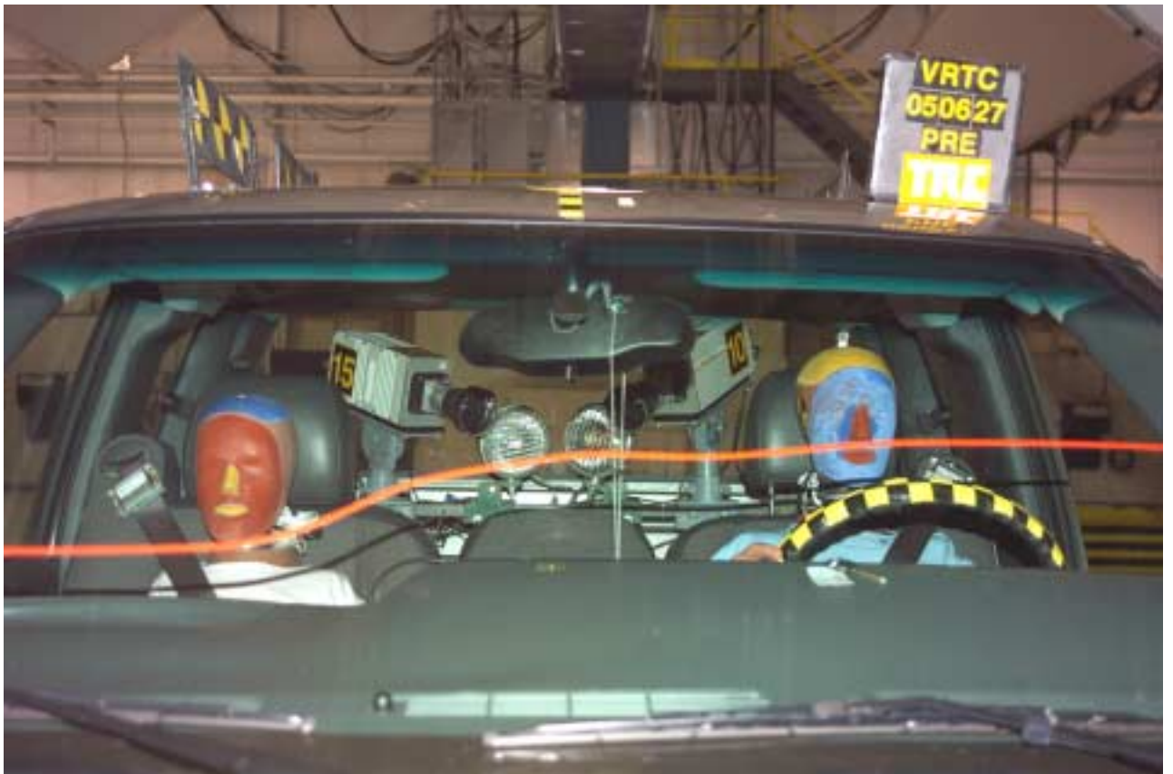
Figure A-94 Pre-Test Bullet Vehicle Driver and Passenger Dummies through Windshield View
