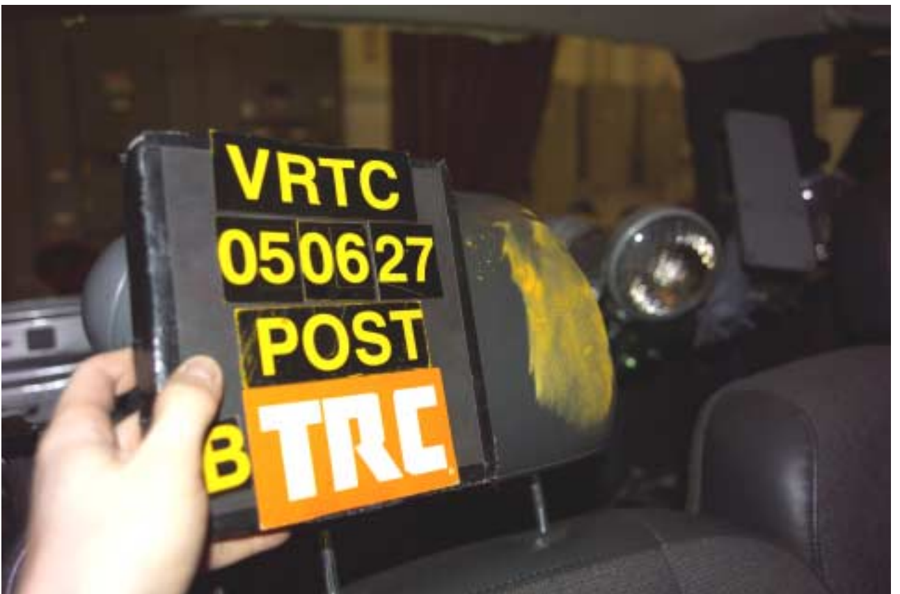
Figure A-132 Post-Test Bullet Vehicle Passenger Dummy Head Contact - View 3
