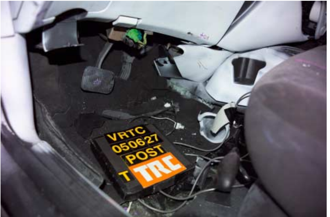
Figure A-135 Post-Test Target Vehicle Driver Floorboard Deformation View
