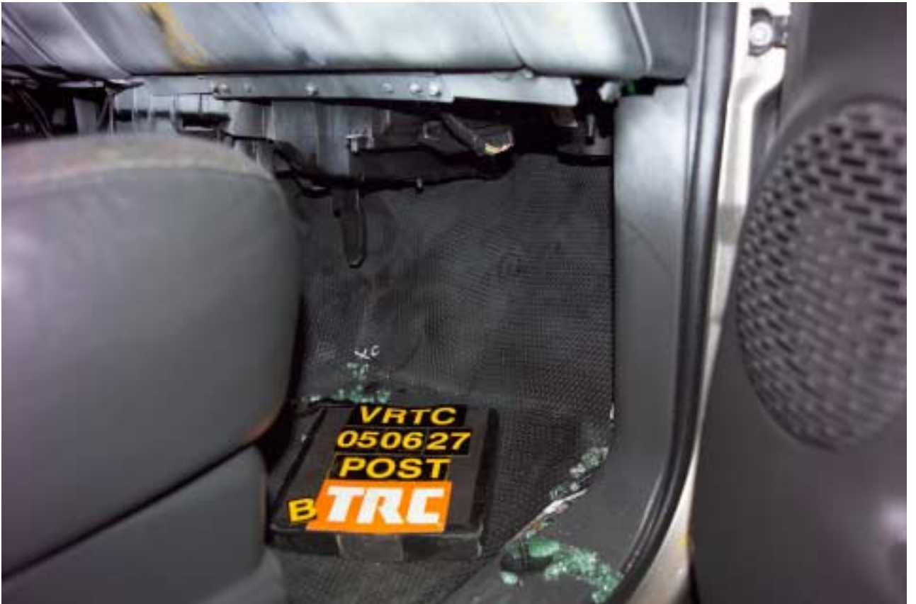
Figure A-141 Post-Test Bullet Vehicle Passenger Floorboard Deformation View
