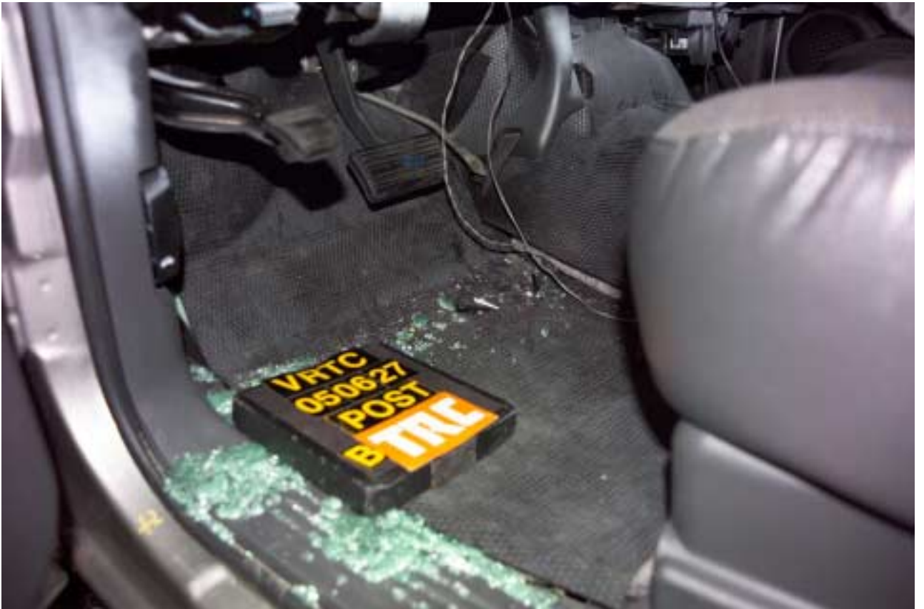
Figure A-139 Post-Test Bullet Vehicle Driver Floorboard Deformation View
