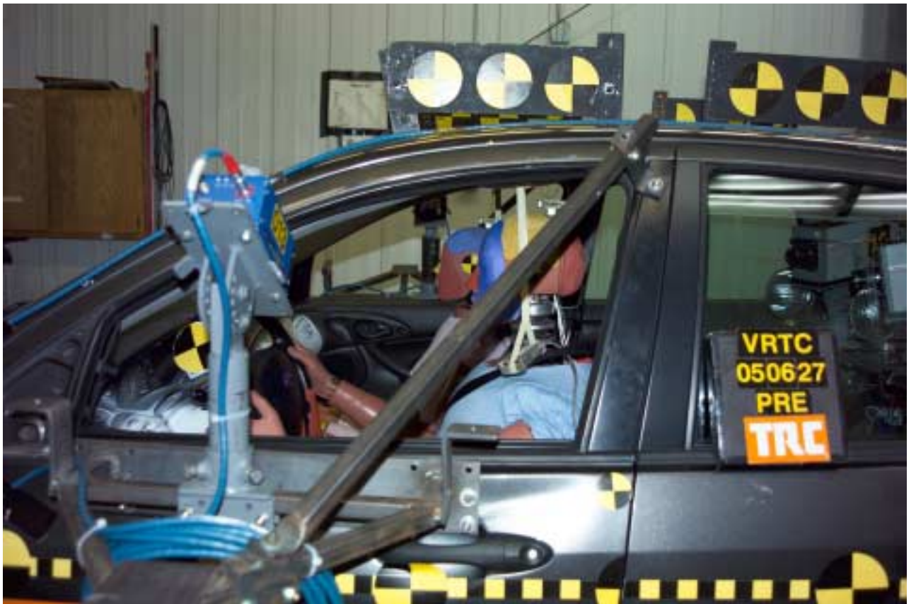
Figure A-78 Pre-Test Target Vehicle Driver Dummy - View 2
