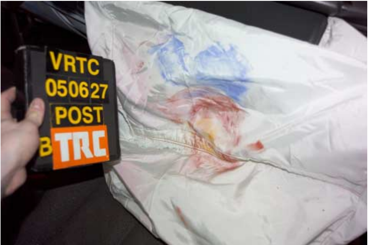
Figure A-131 Post-Test Bullet Vehicle Passenger Dummy Head Contact - View 2
