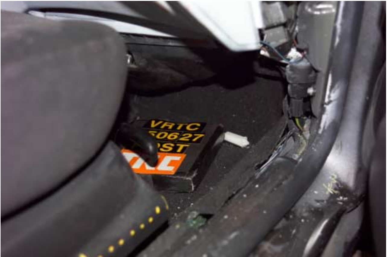
Figure A-137 Post-Test Target Vehicle Passenger Floorboard Deformation View
