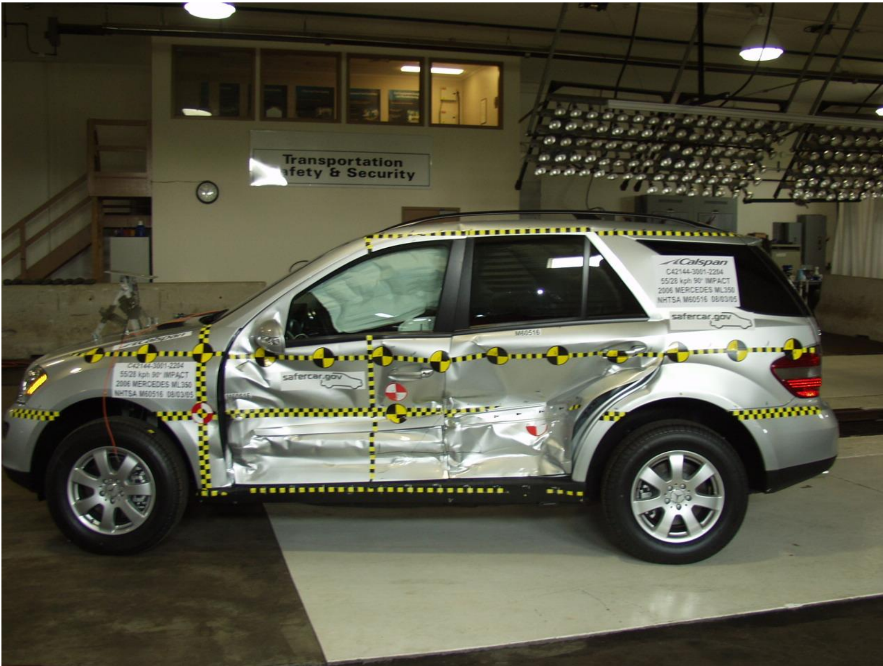
Figure A-6 POST-TEST IMPACTED SIDE VIEW OF TEST VEHICLE
