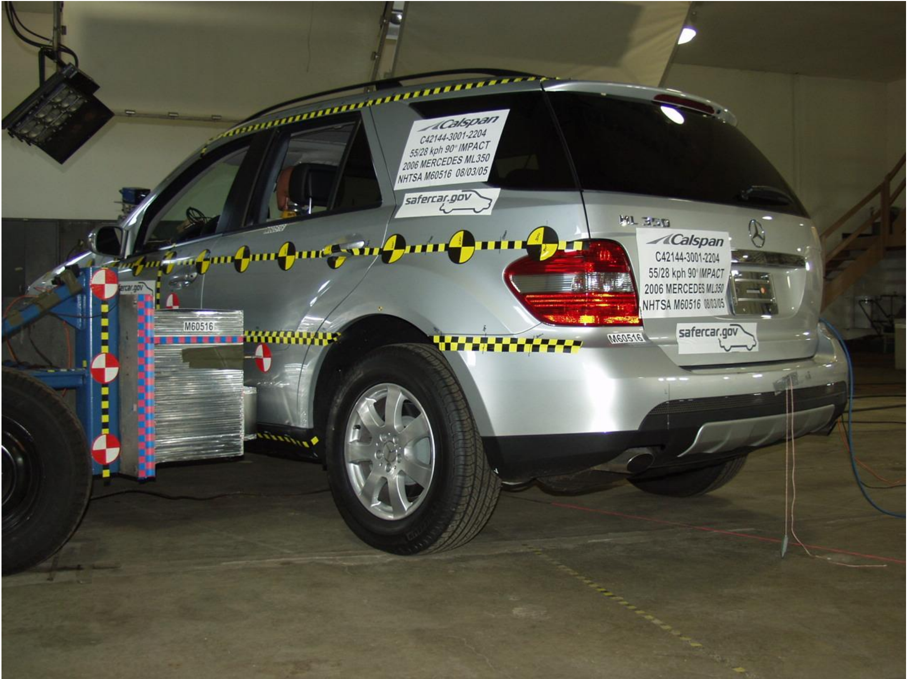
Figure A-38 PRE-TEST RIGHT SIDE VIEW OF MDB WITH IMPACTOR FACE IN POSITION
