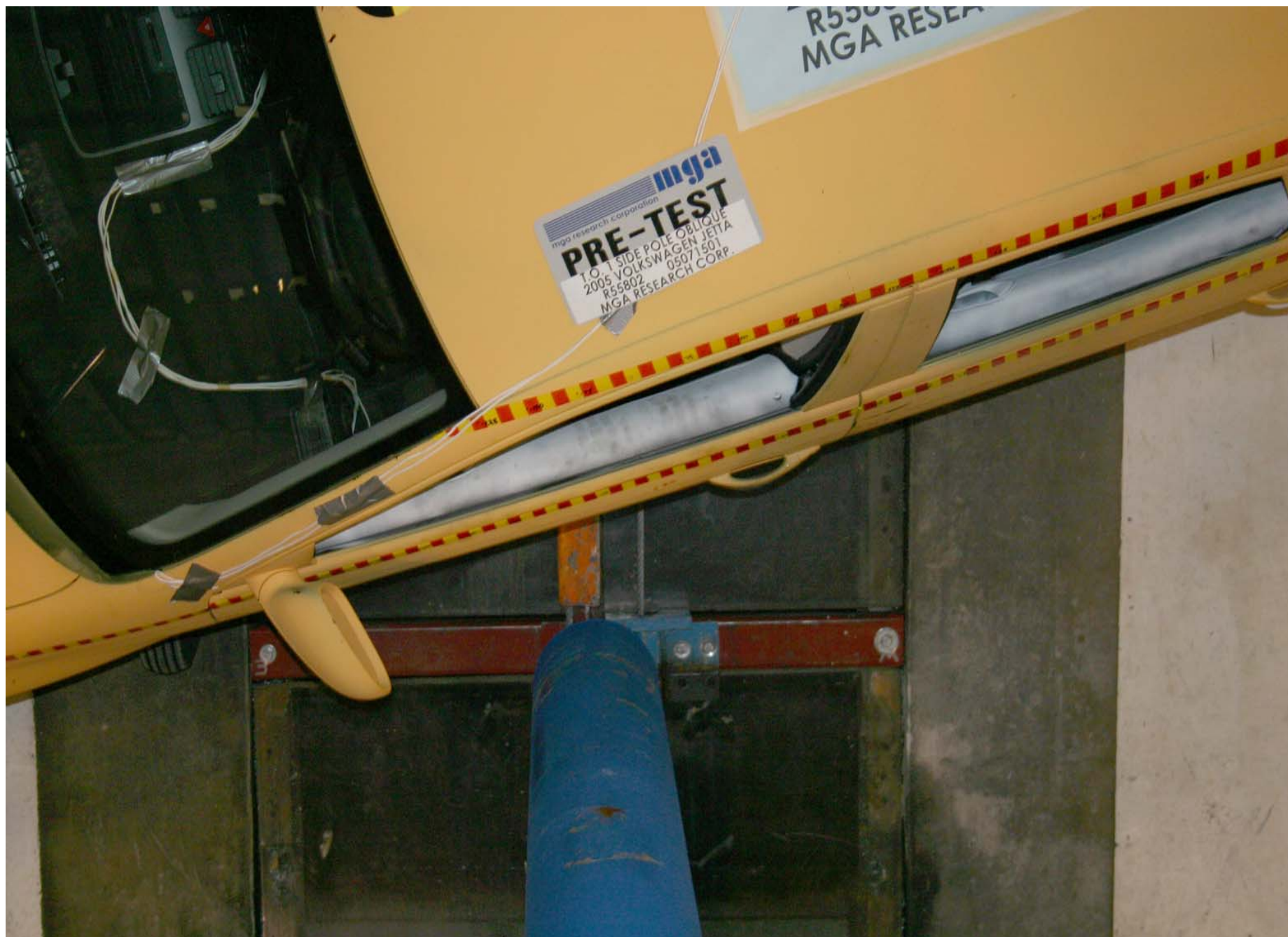
Pre-Test Vehicle Overhead View Positioned Against Pole (Close Up)
